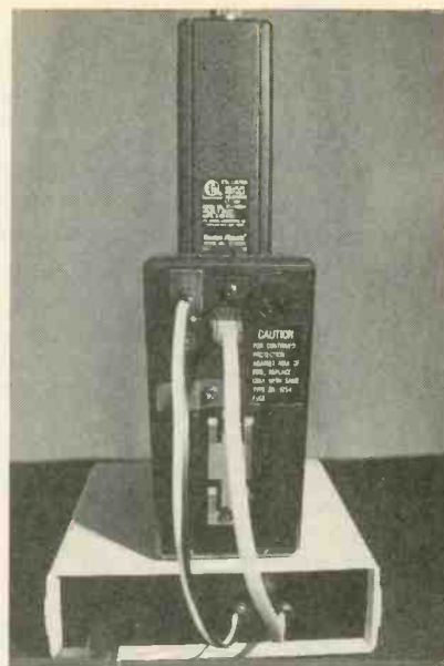
Shown here is the wiring interface between the battery-charging stand and the Battery-Butler.
