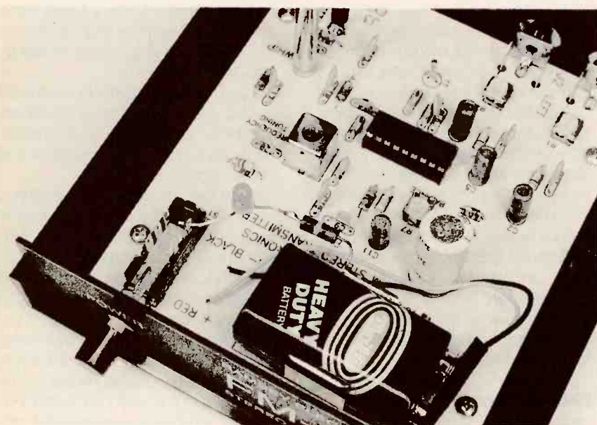
The assembled circuit board is shown here. Note the addition of an LED and a 1K resistor in series, which act as a power indicator (see text).
