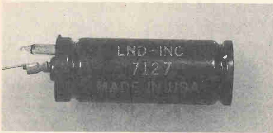
The Geiger Mueller Tube. Be sure to handle it very carefully!
