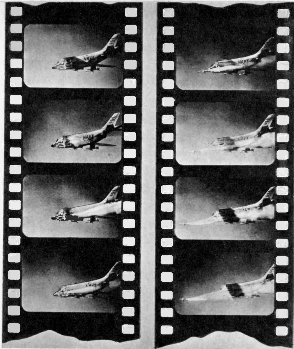
Rapid fire sequence shows Sparrow III, Navy air-to-air missile, being launched from F3H.2 Demon interceptor. Plane carries four missiles which are fired at target automatically when within range.
