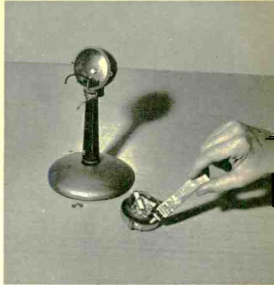
Position cartridge in case and glue shock mounts in place. New shocks may be made of excess rubber.
