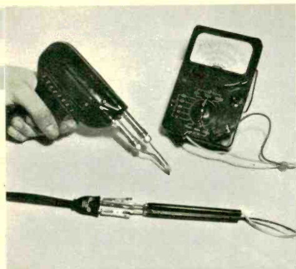
For a quick check, connect an ohmmeter across the gun's plug. Shake and tap the gun to check for an intermittent open in the primary circuit.
