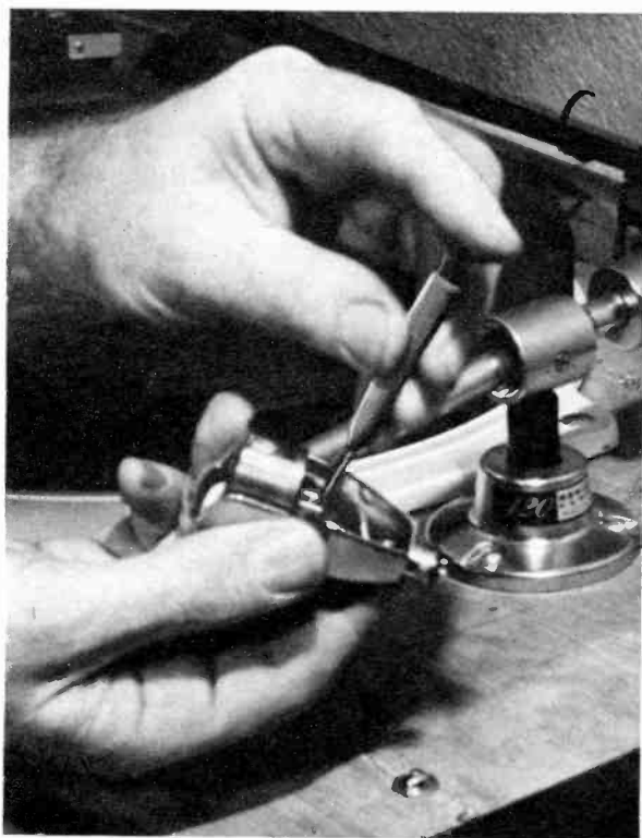
Careful attention to manufacturer's instruction must be paid when installing cartridge in head. Hum and noise in a system are often due to error in grounding and wrong wiring of cartridge.
