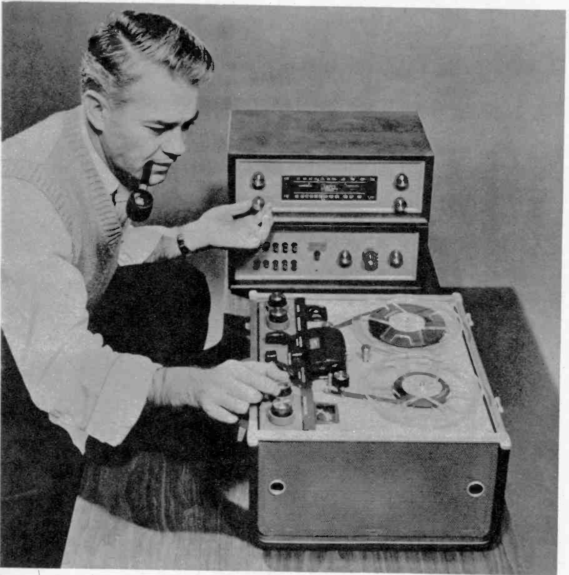
An Ampex 960 tape recorder is being used above to tape a stereo broadcast from AM-FM tuner. Units shown are the Ampex stereo tuner and amplifier. Similar setup lets you record monaural sources.
