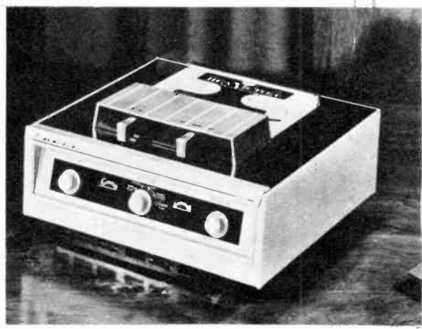
Bell "overture" has 3¾ ips speed, plays tape stereo cartridge. It uses 9 transistors, weighs 25 lbs., has volume level meter, 3 inputs.
