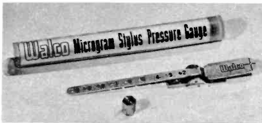
Above are some of the stylus pressure gauges available. At left is one by Clevite Walco, at right is a Garrard. The Walco gauge is unusual in that it has no springs; it uses movable counterweight.
