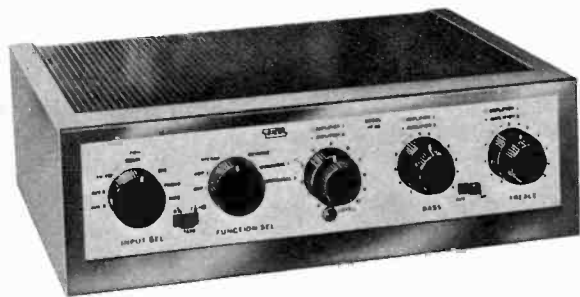
Eico stereo preamp is sold assembled, $64.95, or in kit form, $39.95. It has ganged controls, tape and record equalizer, channel reverse, hum balance.
