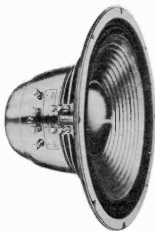
Dual voice coil 12-inch University woofer can be adjusted for 700, 2,500 or 5,000 cps high-end cutoff to suit requirement of the tweeter.
