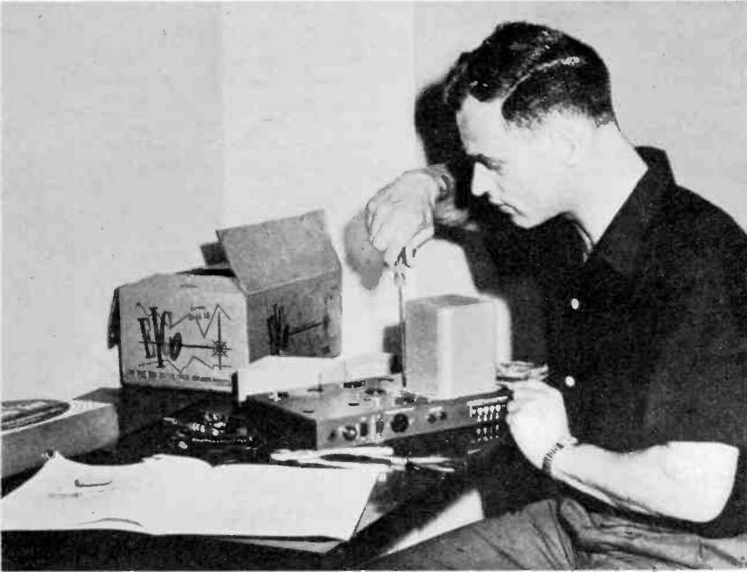
Assembling the Eico HF-50, 50-watt basic amplifier. After mounting external jacks and tube sockets, the heavy output transformer is installed on the chassis. Explicit step-by-step instructions are included with the kit and must be followed at all times for best results.
