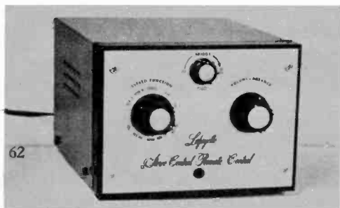
Left: Lafayette stereo adaptor is self-powered, sells for $27.50 in kit form. It has provision for a third channel, plus a phase and channel reverse switch.
