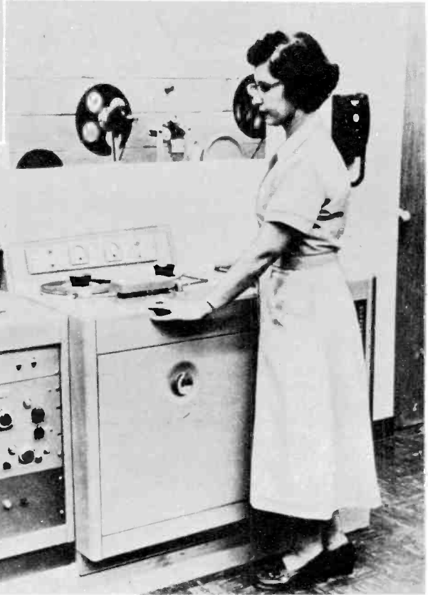
View of Soundcraft factory tape quality control room where tapes are tested against magnetic specs.
