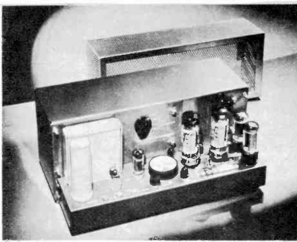
Marantz 40-watt power amplifier has hum level of -90 db at 40 watts. Damping is more than 20; 20-20,000 cps; 4, 8, 16 ohm terminals. Price: $219.
