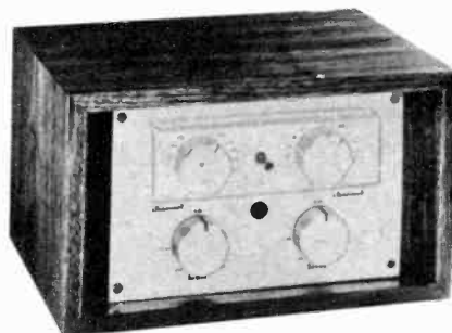
Marantz Model 3 electronic crossover for stereo programs has independent on-off and level control for each channel, low and high frequency knobs.
