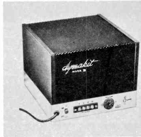
Mark III Dynakit 60-watt basic amplifier has 4, 8 and 16 ohm speaker terminals, outlet for powering a preamplifier. IM distortion is less than 1% at 60 watts. Price of kit: $84.95.
