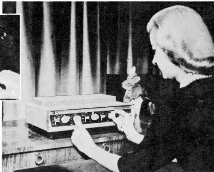
Stromberg-Carlson stereo control amp provides 12 watts for each channel, with individual controls for both channels, plus a master gain adjust.
