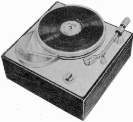
Rek-O-Kut turntable kit costs $39.95, has 33 \frac{1}{3} rpm speed, endless-belt drive. Noise level is -47 db at average recording level; 4-pole motor.
