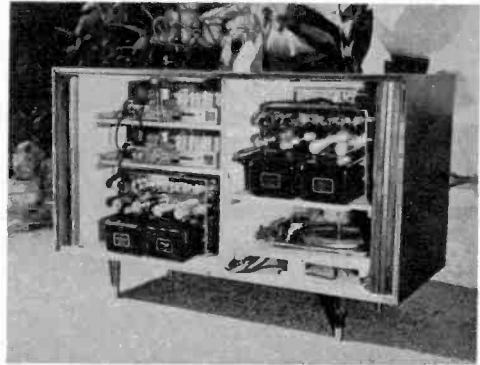
Compact installation in cabinet, front and rear view, includes two McIntosh MR-55 AM-FM tuners, two McIntosh preamplifiers, Magnadette tape recorder and stereo preamp with two VU meters. Turntable is a Miracord XS-200 automatic. Rear view shows two 60-watt McIntosh basic amplifiers installed vertically. Note ample area provided for good circulation of cooling air currents.
