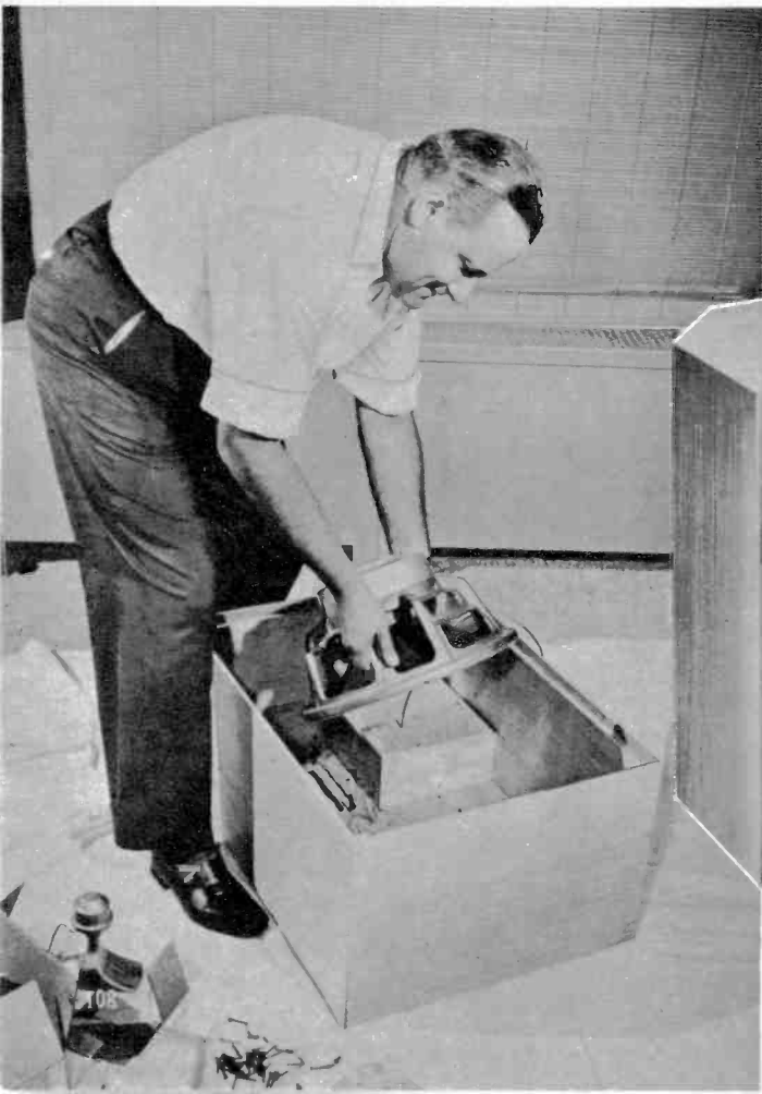
University makes a variety of high-quality speaker kits, including the 3-way KEN-15 model shown here which holds a 15-inch woofer. Plywood veneer gives professional look. All hardware, plastic grille cloth, etc., included.
