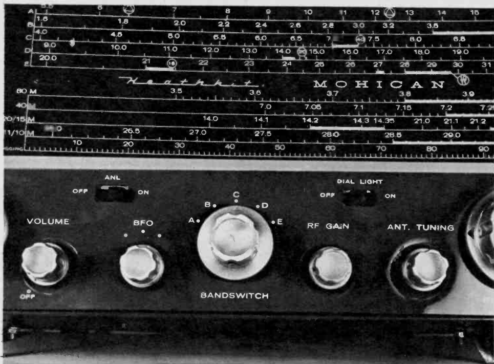
Above: Five-band "Mohican" receiver, made from a Heathkit, is a solid-state set. Works either on dry cells or AC power unit. The slide-rule dial has separate scales for regular tuning of AM and short-wave bands and for band-spreading the special ham bands.
