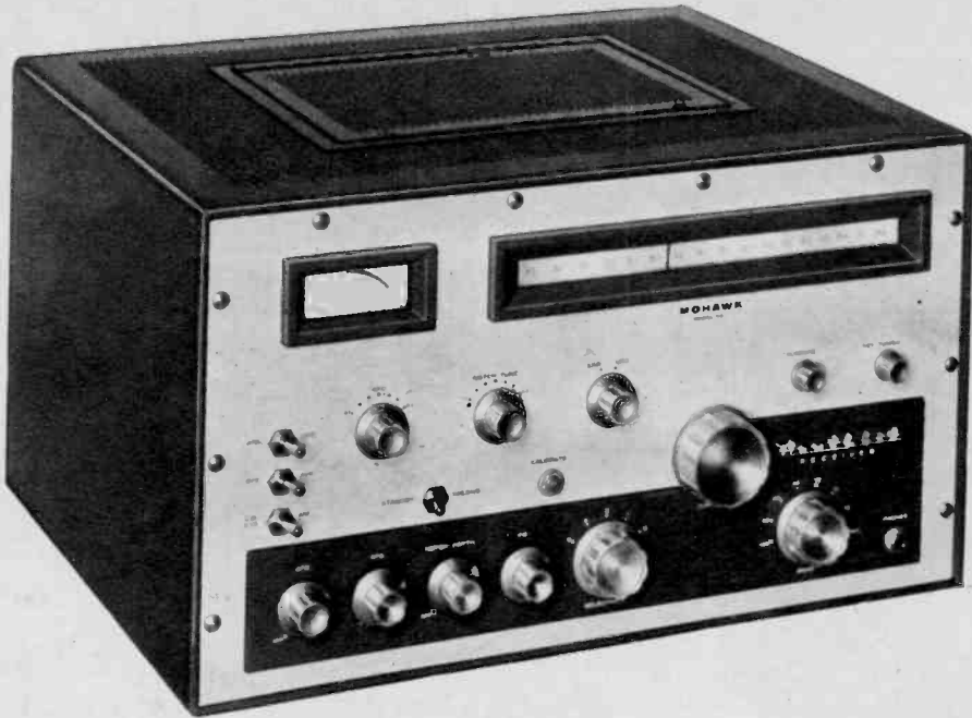
Multiplicity of knobs and switches gives operator of multi-band receivers complete control of all circuit functions. In this Heathkit "Mohawk" eight-band set, a different slide-rule scale pops into view in the long dial bezel as the band-selector switch is rotated. Set includes crystal-controlled calibrator.
