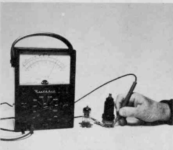
For occasional testing of just a few tubes, use individual sockets, which cost only a few cents each, and touch the VOM leads to their soldering lugs. This is a much more positive method than attempting to touch the probes directly to the base pins. The latter are too close for comfort.
