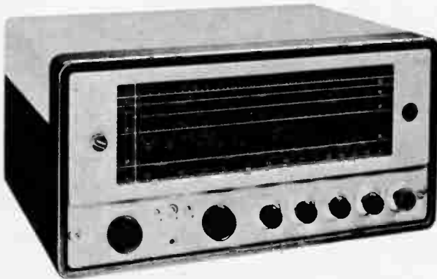
"Slide-rule" type dial is used in Hallicrafters SX-62A, a six-band job that includes the FM broadcast range, AM radio and four short-wave bands. Never a dull moment with this set!
