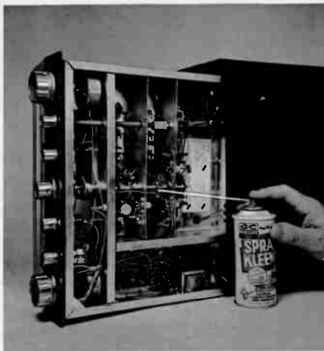
Right: This is probably most important service operation performed on multi-band set: Cleaning the switch contacts with special spray preparation in a pressure can. Use sparingly, as a little goes long way. This is under view of chassis of the Mohican.
