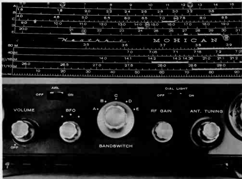
Above: Five-band "Mohican" receiver, made from a Heathkit, is a solid-state set. Works either on dry cells or AC power unit. The slide-rule dial has separate scales for regular tuning of AM and short-wave bands and for band-spreading the special ham bands.
