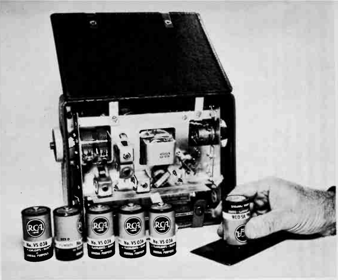
Above: If loose batteries like these "D" cells are used, it is important to keep their terminals clean and bright, so that they make good contact when they are stacked. A few strokes against a piece of sandpaper or emery cloth do the job satisfactorily.
