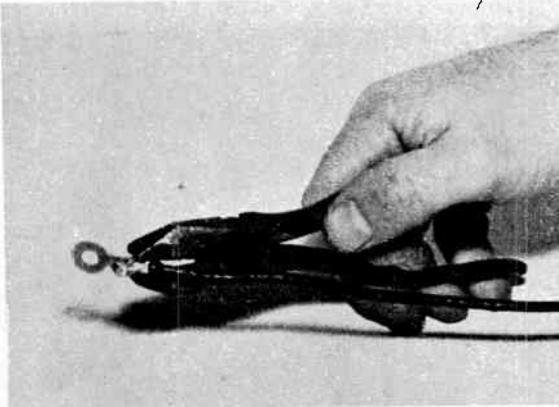
Blunt, strong jaws of electrician's pliers are also fine for holding and squeezing jobs. Typical use for them is to close the ends of a terminal lug around the end of the wire that's soldered to it.
