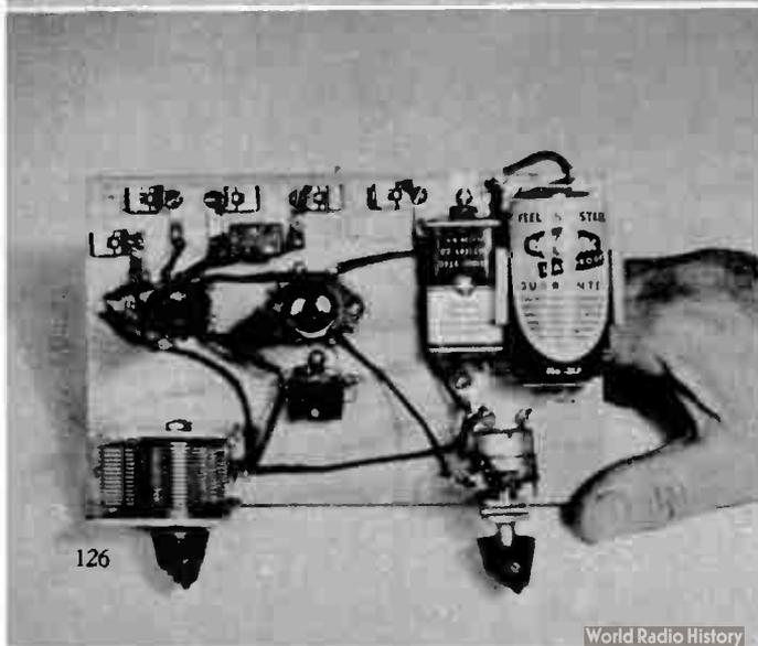
This is completed "chassis" ready to operate. Batteries fit in the spring clips on baseboard. Battery "B" should last 6 months.
