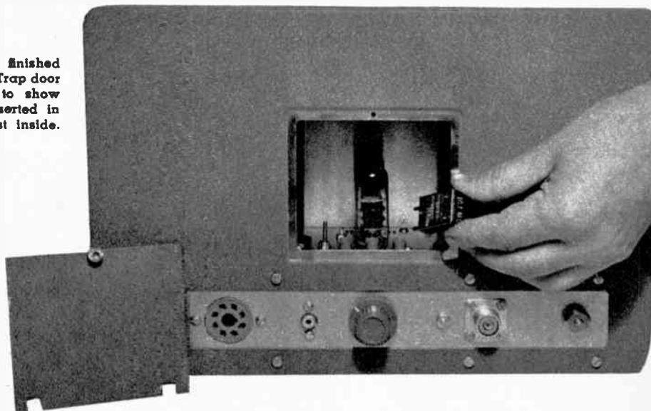
and a four-position crystal-VFO switch. Access to the three crystal sockets is through a small trap door in the back of the cabinet.
