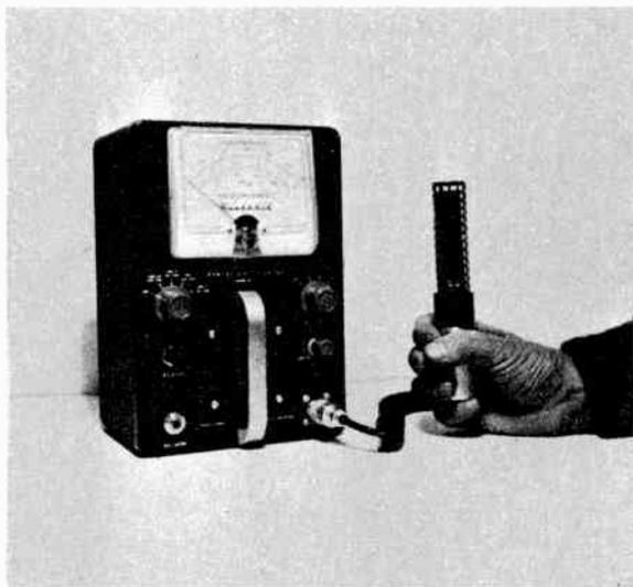
The Heathkit Radiation Counter has the probe on the right. Loudspeaker, giving out tone signals to indicate radioactivity, is under the carrying handle. Complete kit is available for about \$80.
