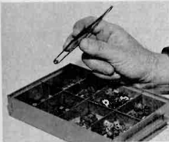
Ever try to pick up a tiny washer, nut or similar small item with your fingers? You can save time and temper by using a pair of these long tweezers.
