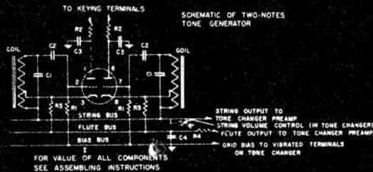
Above is the schematic diagram of an individual tone generator of the electronic organ. Single 12AU7 tube functions as a dual audio oscillator and produces two notes of different frequency.
