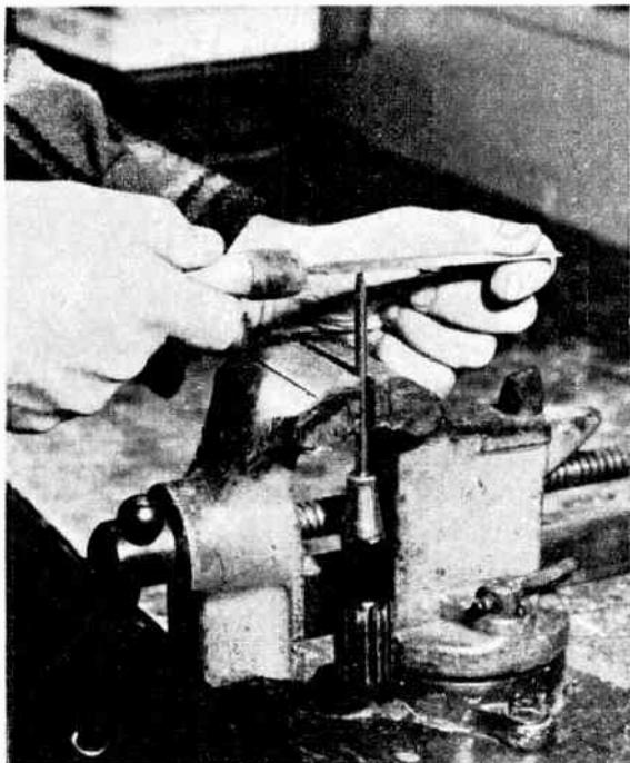
It is important to keep the tip of the screwdriver blade flat and square. It is bound to wear with use, and therefore should be touched up frequently. A sure sign that it needs attention is its tendency to deform the slots of screws when pressure is applied. A few strokes of a fine file usually do the trick. Remove any burrs left by rubbing the blade lightly over fine oilstone.
