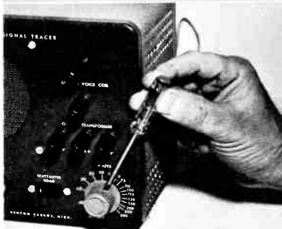
When it is necessary to turn a "tough" screw, use this grip. Get the handle's end into base of palm, under thumb joint, and support the ferrule (part into which blade fits) with the thumb and forefinger. You can thus exert both pressure and turning effort at the same time. Leverage in a screwdriver is determined by handle size; the greater its diameter, greater the lever action.
