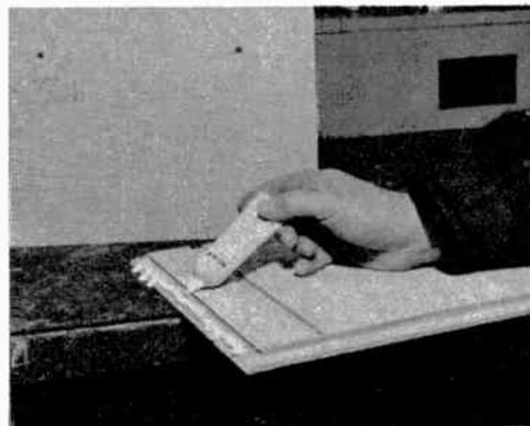
6. Glue is applied to beveled edges of second end panel and top panel. Though a little too much has been applied in this photo, it does no harm.
