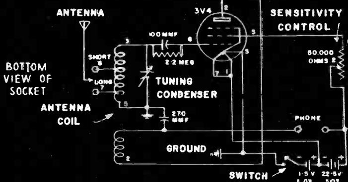
At top is the wiring of one-tube set. At bottom is schematic diagram, details of socket connections.
