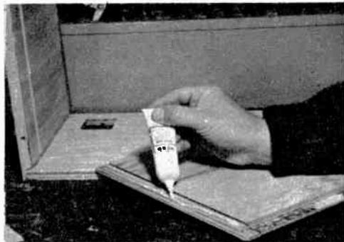
4. Here glue is being applied to the beveled edge of the bottom panel of the box. This will be placed against the forward beveled edge of the end panel as demonstrated in picture No. 3.
