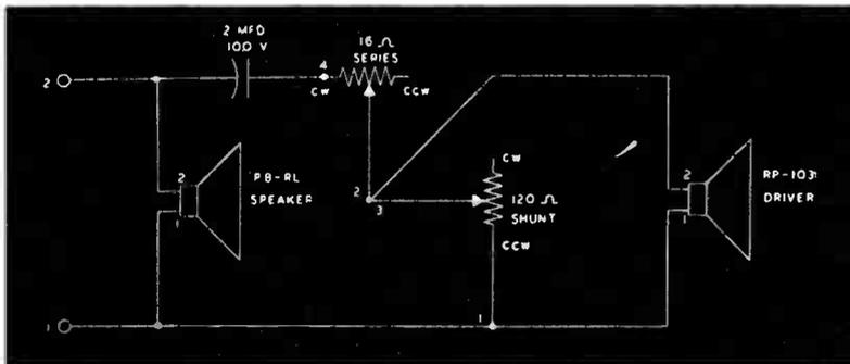
25. This wiring diagram shows the loudspeaker connections.
