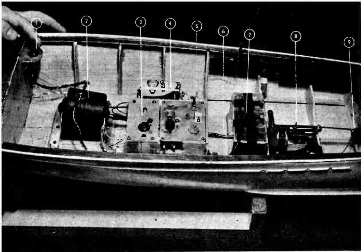
Inside of the R/C model boat, with the superstructure removed: 1. Drive motor switch. 2. Drive motor. 3. On-off switch and meter jack of receiver. 4. Flashlight cells for receiver. 5. Receiver panel. 6. Propeller drive shaft. 7. Storage battery. 8. Rudder escapement. 9. Rudder post. Various parts are distributed to balance boat in water: motor is forward, storage battery toward stern.
