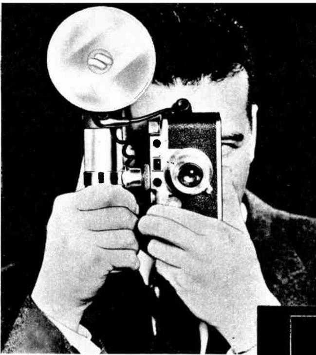
Here a typical small electronic repeating flash unit is shown mounted on a Leica camera. This is the Strobonar Seven, which derives its high voltage from but a single large dry battery.
