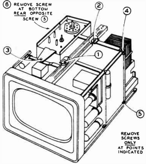
Though tight and compact, the receiver is easily opened when this sequence of operations is followed.
