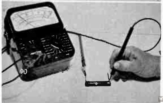
To measure resistance of a fixed resistor, clip one test lead to one terminal and touch other lead to second. Be sure circuit tester is set to DC.
