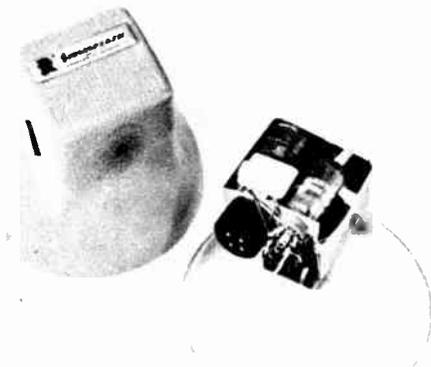
transformer T. This transformer is virtually identical with the small ignition coils widely used in model airplanes. The switch SY, representing the "synchronizer" contacts on the camera shutter, is open. The secondary winding S of the transformer connects to electrode 3 in the flash tube, placed somewhere along the gas-filled spiral between electrodes 1 and 2.
