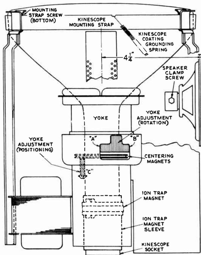
Skeleton top view of the set shows how loudspeaker is nested neatly against body of the picture tube.
