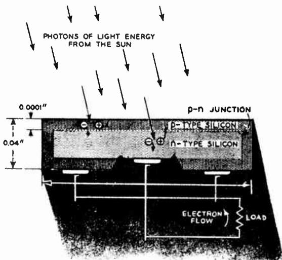
Fig. 4. Cross-sectional view of a silicon p-n junction solar cell, illustrating the creation of electron-hole pairs by photons of light energy.
