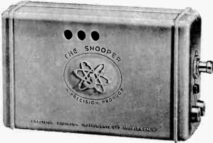
The Model 108 "Snooper" is a basic Geiger counter, taking about as much pocket space as three packs of cigarettes. Produces a loud series of clicks in earphones (not shown) in the presence of radioactive material, the number of clicks increasing as the material becomes closer. Works on one flashlight battery and one 22½-volt hearing aid type B battery. Size is 1½x3x5 inches. Price, \$29.95.
