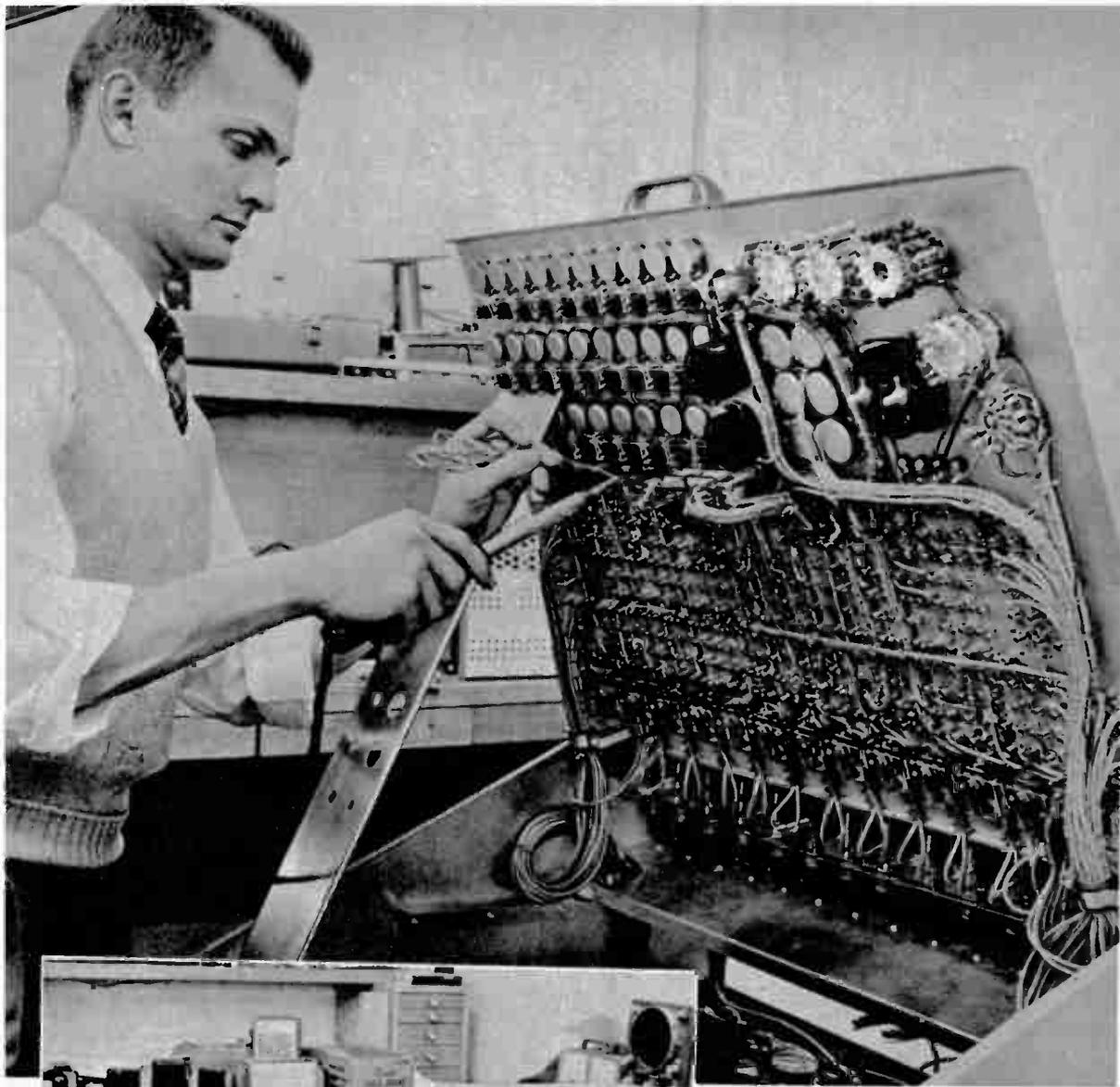
Carl Heald, project engineer on the development of the analog computer kit, puts a few finishing touches to the wiring of a laboratory model. Hinged main panel is easier to work on than the chassis of many radio sets.
