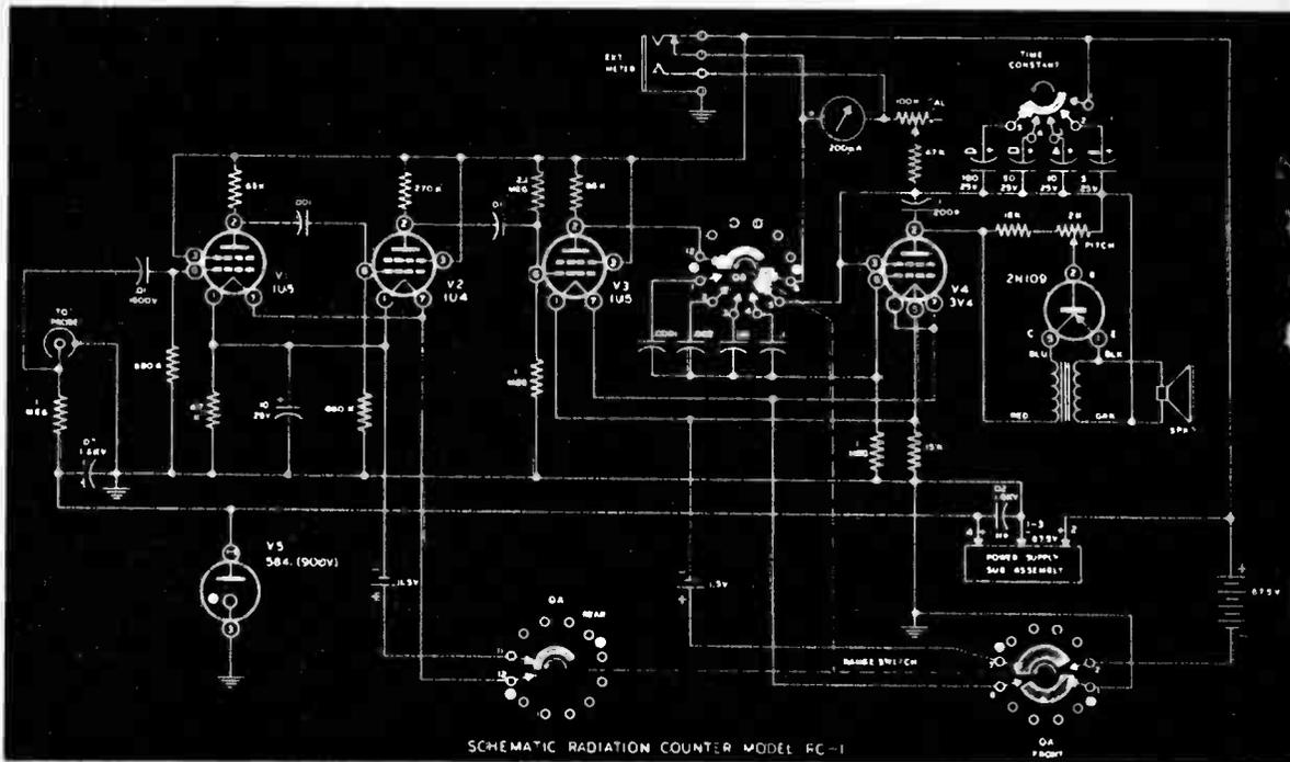
Complete schematic diagram of Heathkit Radiation Counter. The device marked 2N109 is a transistor.
