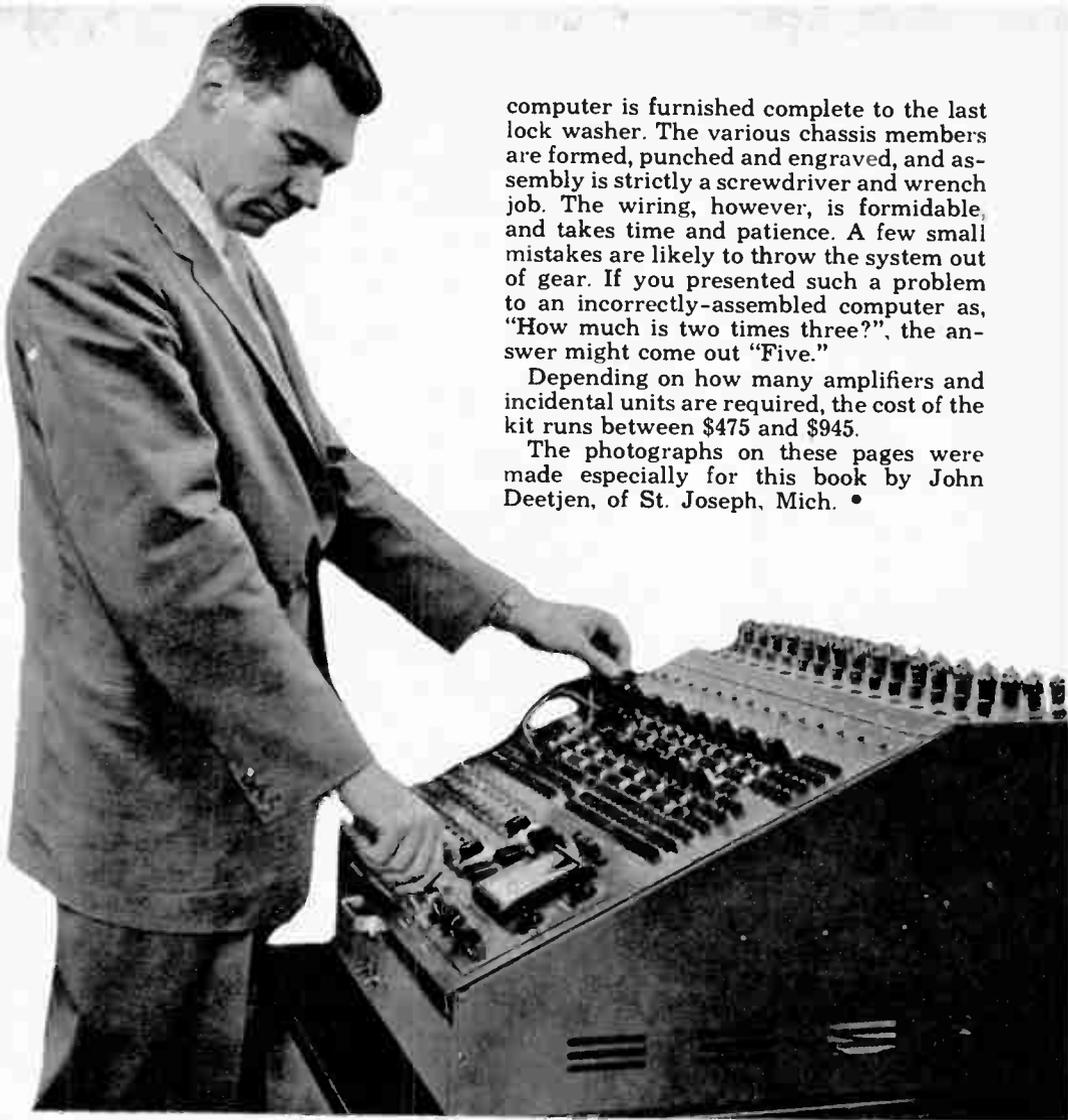
computer is furnished complete to the last lock washer. The various chassis members are formed, punched and engraved, and assembly is strictly a screwdriver and wrench job. The wiring, however, is formidable, and takes time and patience. A few small mistakes are likely to throw the system out of gear. If you presented such a problem to an incorrectly-assembled computer as, "How much is two times three?", the answer might come out "Five."
