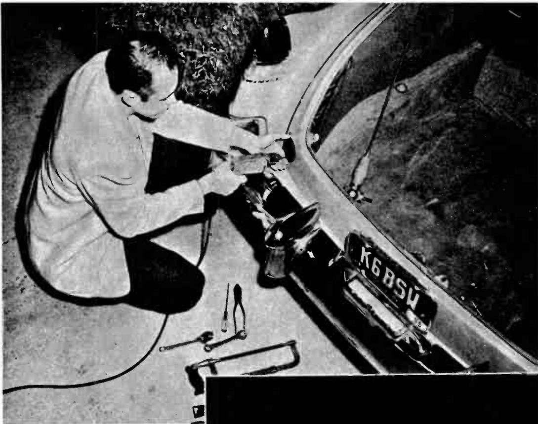
With electric drill, holes are bored for mounting whip antenna. Lead-in from antenna to equipment up front is easily snaked through trunk and under seats and floor mats. Antenna, in trunk, fits on powerful coil spring and "gives" if it brushes obstruction.
