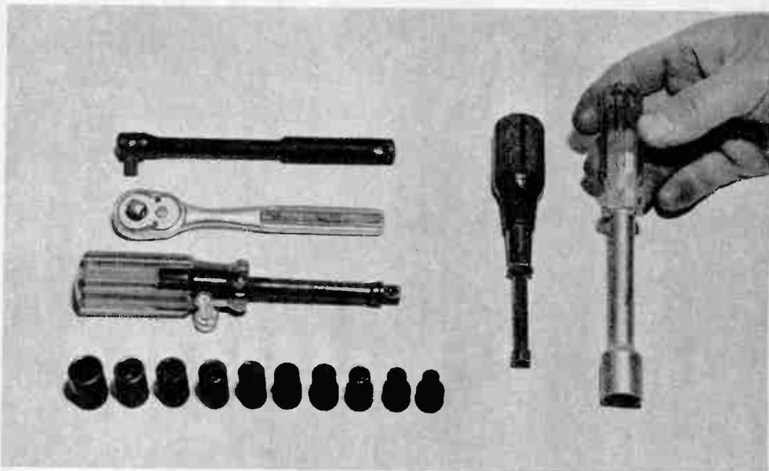
Combination spread out horizontally, left above, is a ratchet socket wrench set. Individual nut wrenches,  $3/16$  to  $7/16$  inch in size, bottom row, snap on square ends of any of three holders above them. Top, adjustable angle handle; center, ratchet handle; bottom, screwdriver-type driver. This is an extremely useful handful of tools. Individual nut-drivers, on right, are much like screwdrivers. One on extreme right has a hollow shank and is especially designed for volume control shafts.
