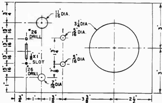
Panel drilling layout for cabinet model
