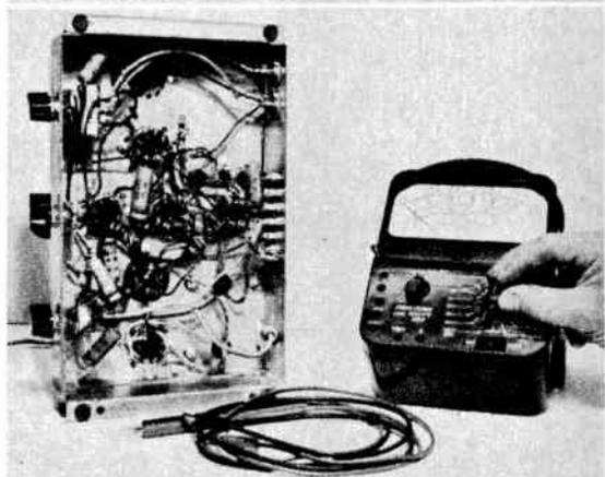
Connect test leads at meter. For DC measurement (most usual one in amplifiers, receivers, etc.) attach alligator clip to end of negative lead and fasten to clean spot on chassis. Latter is invariably minus side of DC circuit in equipment.
