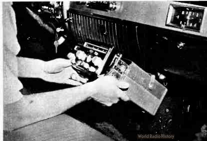
Transmitter is eased into its case on right. Receiver is already in case on left, where it is usually placed, nearer operator, as it requires more "knob-twisting." Both chassis are easily installed, removed.
