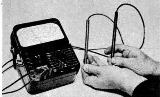
**DON'T** try to move circuit tester by pulling leads.
