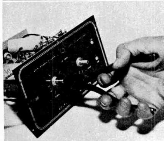
Flat jaws afford a good grip on hex nuts if the shaft of the control device is not so long that it will extend out into the joint of the tool.
