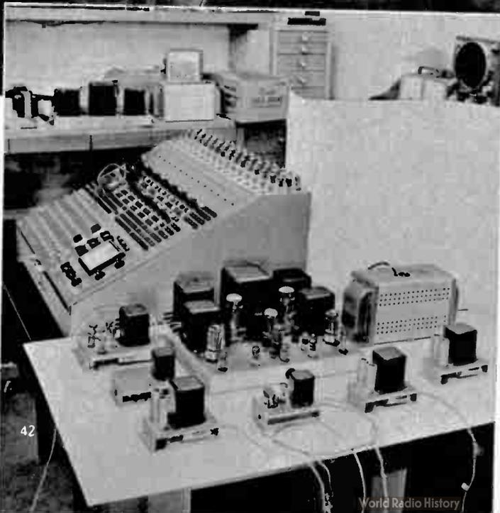
On the table are some units that are normally stored inside the angled cabinet. Large center unit is the amplifier power supply; to its right, a constant-voltage transformer that smooths out power line fluctuations. Smaller chassis are oscillators and power supplies.
