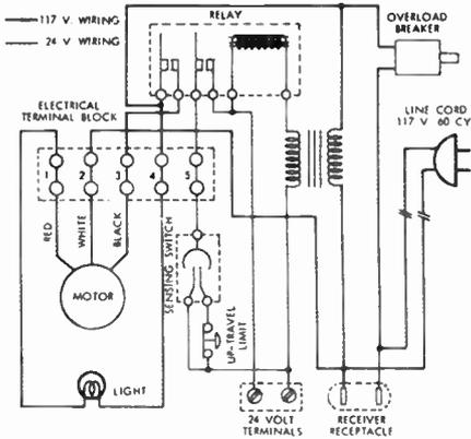
Here is wiring diagram of the motor head unit.
