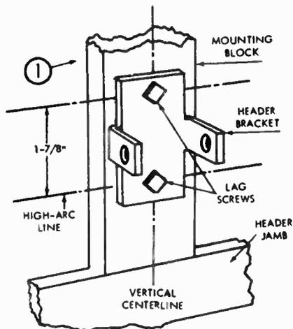
The drawings on these pages show some of the details of the garage installation. The motor is belt-coupled to a chain drive on the long horizontal rail. The chain carries a trolley which in turn is connected to the garage door itself by an L-shaped arm. The motor is equipped with a safety clutch, and the door stops in transit if it encounters any obstruction. Power to the motor also goes off.
