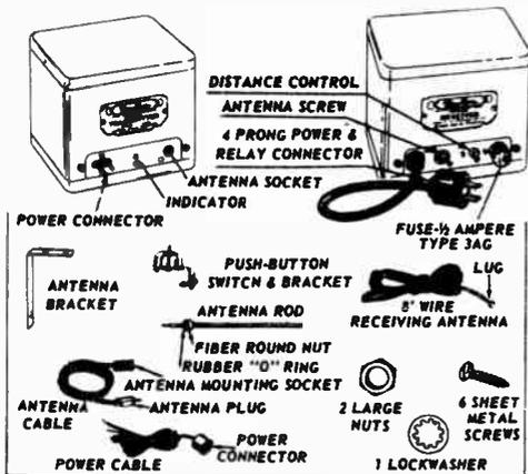
Left. These are the essential electronic parts of radio-control units of the garage door opener.
