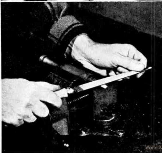
Tips of soldering irons must be kept smooth and clean. Frequent filing eliminates pitting. Use a fine file. To "tin" a tip after cleaning, plug in the iron and hold solder against it as it heats up. Copper wire loops of gun-type iron are readily replaceable. It is ordinarily impossible to solder aluminum. Solder merely forms globules on it, which run off. The tips of all soldering "irons" are made of copper; they're not iron at all.
