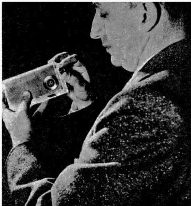
This one has its place in the sun, and in darkness, too! Edward Keonjian, General Electric engineer, demonstrates it—an experimental sun-powered broadcast receiver. Tuning knob is on front surface; volume control on end.
