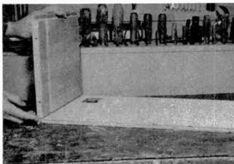
3. Back of box is placed face down on workbench and used as a form to keep the box itself square during assembly. One of the end panels is being positioned. On level-table, it will stand alone.
