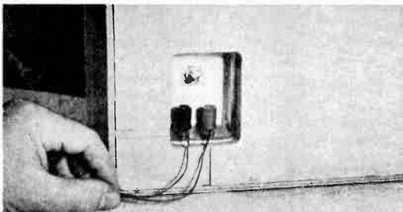
26. Here back has been screwed into place. The two binding posts are for connection of speaker system to hi-fi amplifier. Knurled shaft adjusts volume from tweeter.
