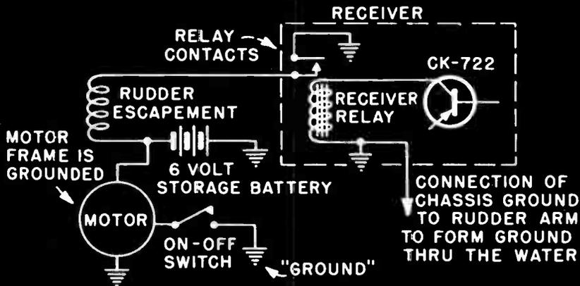
Diagram above of boat wiring shows connections of receiver relay, rudder escapement and motor drive.
