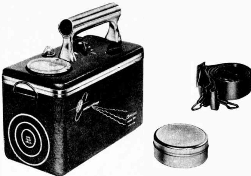
Completely self-contained, the "Oracle" is a portable uranium prospecting instrument measuring only 10x5x6 inches overall and weighing about 8 pounds. It uses 10 Geiger counter tubes and operates even if several fail. Costs \$395 and is made by the Chicago Nuclear Instrument and Chemical Corporation.
