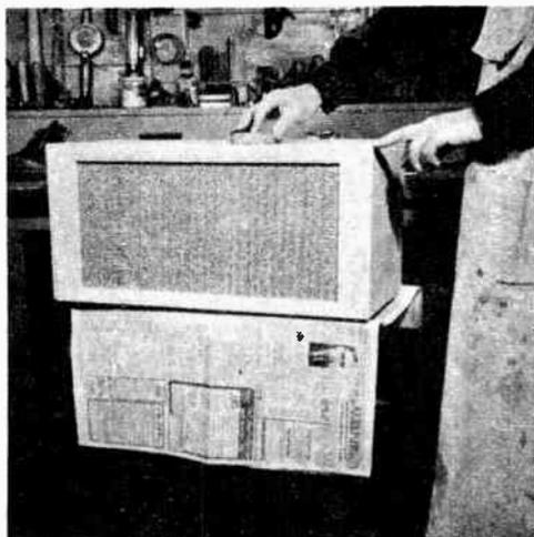
27. Although plywood panels of the loudspeaker box are furnished already sanded, a final treatment with very fine sandpaper is recommended.
