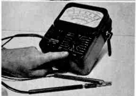
Preparatory to making resistance or continuity checks with circuit tester, "zero" the meter by short circuiting test leads together and turning the ADJ:OHMS knob until needle swings to 0.
