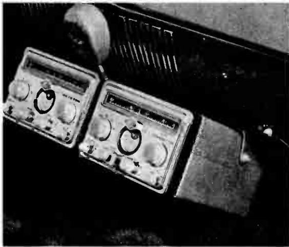
Microphone hangs on dashboard hook above Gonsett G66 receiver and matching G77 transmitter. Units are only  $6\frac{1}{2} \times 4\frac{1}{2} \times 9$  in. in depth. Receiver covers 6 bands including regular AM broadcast band. As band switch turns, a drum dial turns and correct slide rule-type tuning scale comes into view. A similar arrangement is used in the transmitter. Angled units permit driver to read at a glance.
