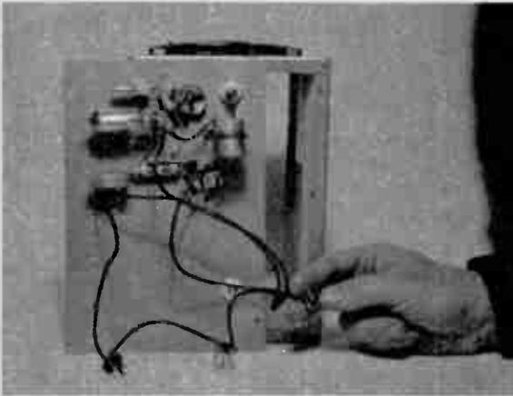
Here is a back view of transmitter panel, assembled and wired. Small connectors are for batteries.
