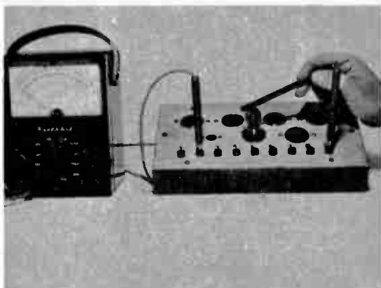
Are internal elements of a tube touching where they shouldn't? An easy way to find out is to connect multimeter between suspected elements and tap tube with pencil. If needle flickers (on high-ohm resistance scale) the tube is bad.
