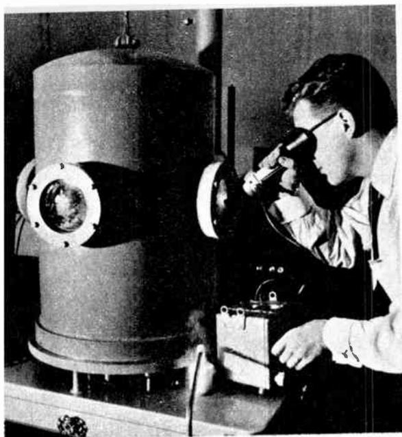
C. A. Lee, Bell Telephone physicist, peers into vacuum oven and adjusts gauge to determine the temperature in diffusion chamber where the new germanium transistor is made. Tiny impurities give the material unique electronic properties.
