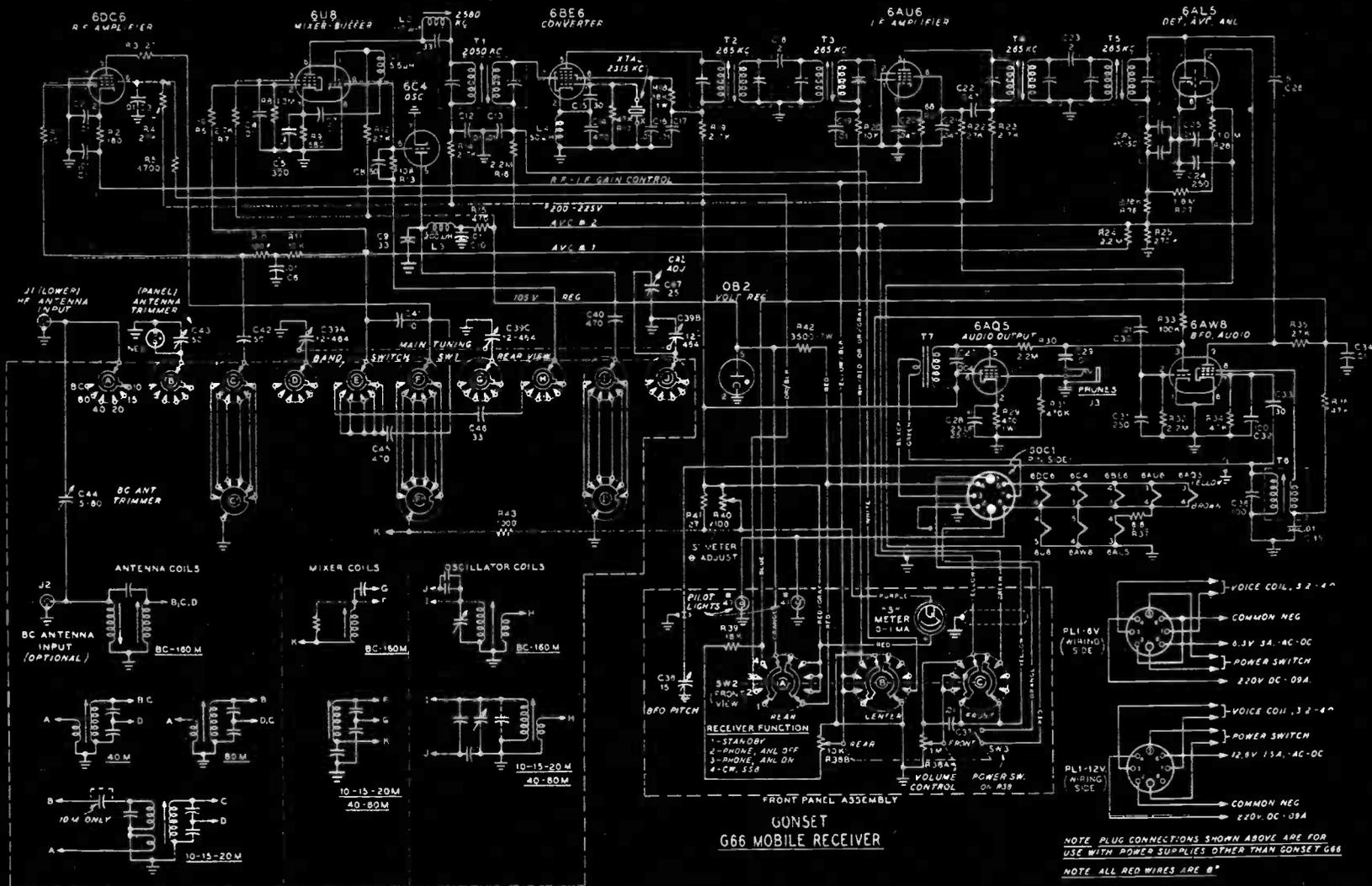
Complete schematic diagram of Gonset G66 mobile receiver. Note use of 2315 kc. crystal oscillator, with 6BE6 converter tube, top center, for second conversion of signal from 2050 kcs. to 265 kcs. (2315 - 2050 = 265).
