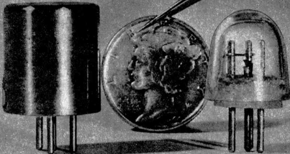
These are laboratory models of silicon (left, with brass cap) and new germanium (right, in glass) transistors announced by the Bell Telephone Laboratories. The dime in center gives size comparison.
