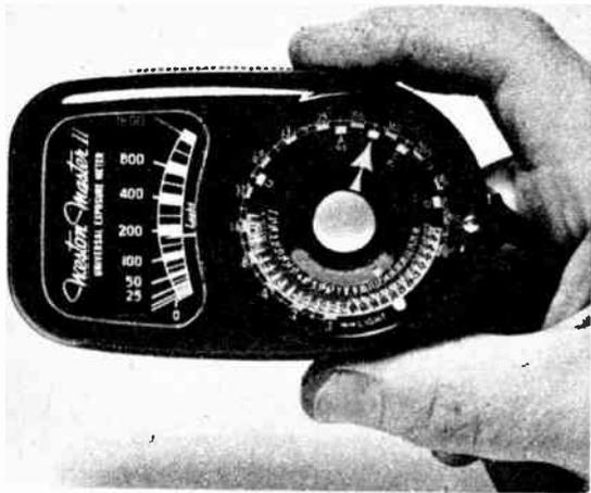
Popular application of older type "solar battery" is represented by photographer's exposure meter. A light-sensitive cell generates minute current which registers on microammeter. Scale of latter is calibrated in lens openings and shutter speeds.
