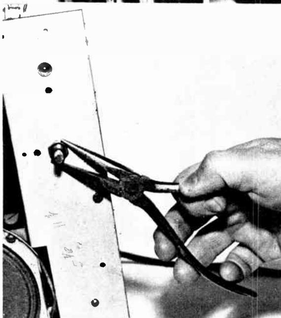
DON'T use long-nose pliers on sizable nuts such as those to be found on volume controls, switches, etc. It is sure to twist the tool's fine ends out of alignment and render them useless for fine parts.
