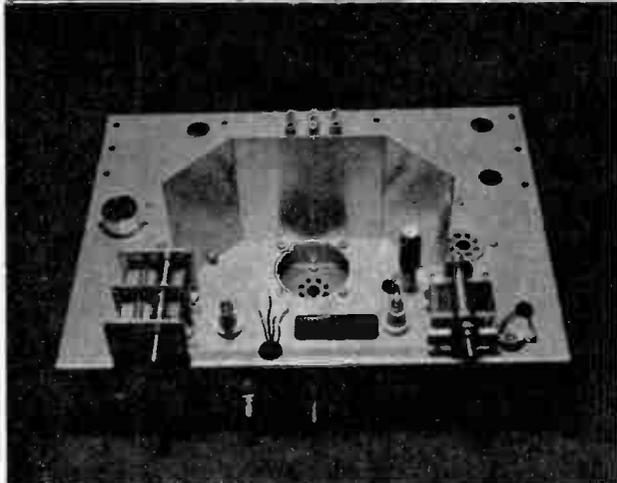
Chassis view of the completed transmitter. The rectifier tube, in hand, fits in socket behind large power transformer, at left foreground. Smaller unit at the lower right is filter choke in high-voltage DC supply circuit.
