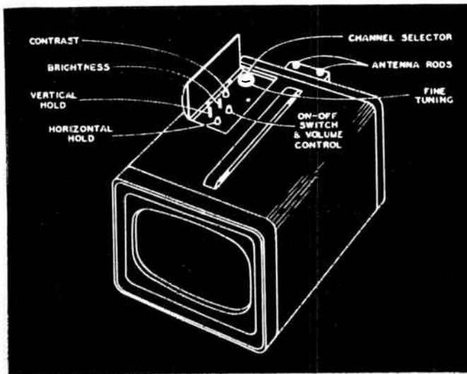
Tuning controls of "Personal" television receiver are under lid near the back of the cabinet.
