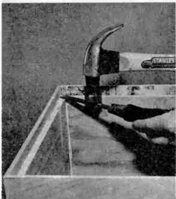
7. With ends, top and bottom of box joined, clamp nails are driven flush with recessed lips. Screw-driver blade is used to avoid damaging corners.
