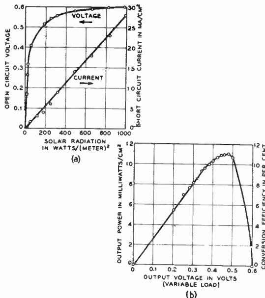
Fig. 5. Electrical characteristics of a silicon p-n cell at an operating temperature of 17° C.
