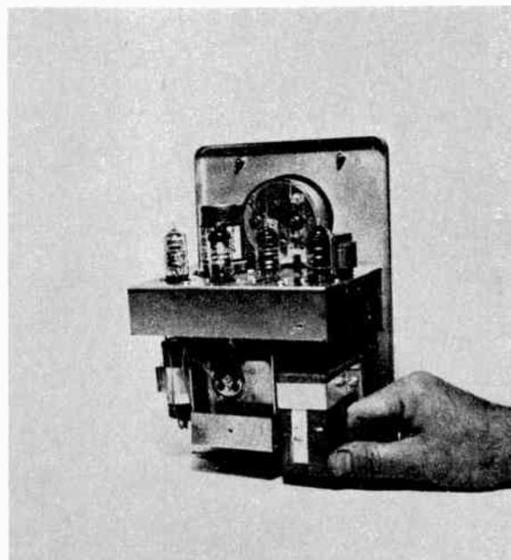
Inside of Heathkit Radiation Counter looks like that of vacuum tube voltmeter or a small radio. Its batteries are held in clamps at the bottom.
