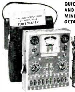
QUICKLY AND EFFICIENTLY TESTS RADIO AND TV TUBES INCLUDING: SEVEN PIN MINIATURES; EIGHT PIN SUBMINARS, OCTALS AND LOCTALS; NINE PIN NOVALS
