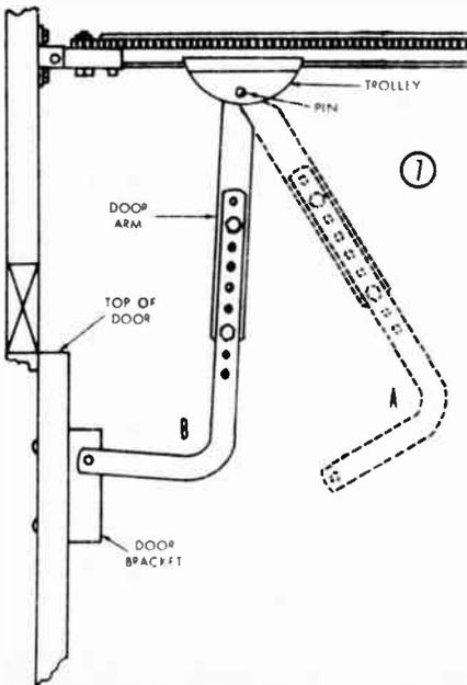
7. With door closed, trolley is near end of rail and door arm is vertical. Arm can be unhooked readily if manual operation of door is desired.
