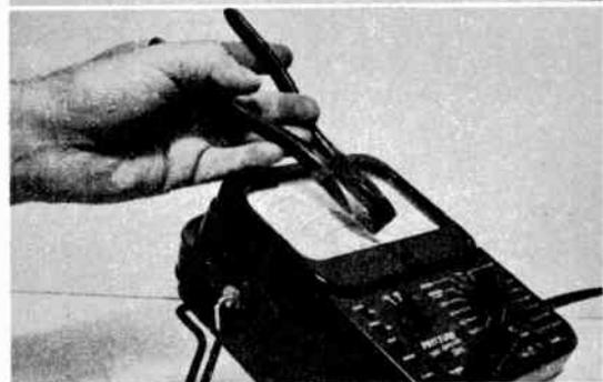
**DON'T** try to check AC line voltage by means of regular test prods; if they touch, there'll be a grand short circuit and blown fuse. Instead, make a simple test cord with regular attachment plug on one end and pins on other to fit meter jacks. It is interesting to observe the line voltage variations as appliances go on and off.
