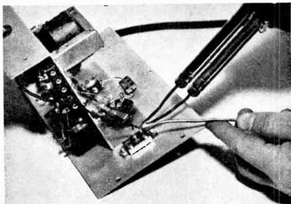
**DON'T!** If chassis is placed in this position, melting solder and rosin will run into the switch, possibly fouling up contacts inside. Remember that hot solder flows just as freely as water.
