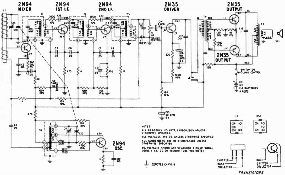
Here is complete schematic diagram of Zenith all-transistor portable. Earphone plugs into jack J1, between the 2N35 transistor and audio transformer T4. The output stage uses two 2N35's in push-pull.
