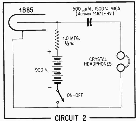
tutes a serious shock hazard, we do not recommend connecting the headphones in series with the other elements in the way this was done in Circuit 1. Instead, high-impedance headphones are capacitance-coupled to the circuit through a 500-mmfd 1500-volt mica capacitor. Crystal-type headphones can be used to advantage.
