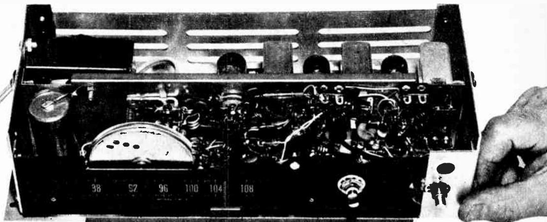
Chassis view of Heathkit FM tuner with cabinet off. Dial is calibrated directly in mcs., from 88 to 108.
