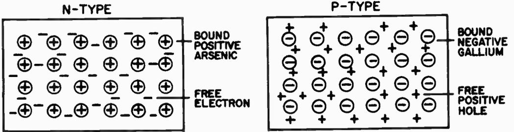
N-type, or electron-rich silicon is made by adding minute traces of an element like arsenic to silicon. From each arsenic atom that is added, one electron (unit negative charge) detaches itself, thus becoming free to move, and leaves behind the arsenic atom with unit positive charge bound into the crystal structure. Thus, n-type silicon consists of silicon to which is added equal numbers of free electrons and bound positive charge, so that there is no net charge.
