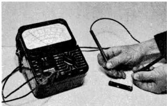
Electrical resistance of body is in line with values of resistors commonly used in electronic equipment, as this simple finger test shows. Indicated value on meter is about 500,000 ohms. Resistance is relatively low when fingers are damp and clean; higher when they are dry and dirty. A sensitive meter will fluctuate even when the pressure of fingers on the test leads is changed.
