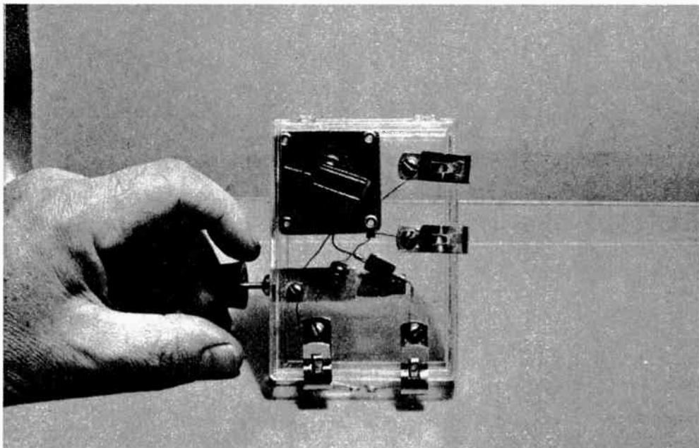
**It uses a crystal detector and earphones, requires no batteries or other current and will produce excellent results with a good aerial.**
