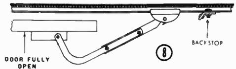
8. Position of door and trolley when the door is fully open. The backstop prevents over-running.
