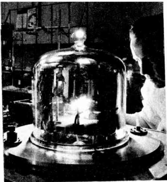
A Bell Laboratories technician performs one of the operations in making new germanium transistor. Here electrical contacts are made to germanium by vaporizing a metal onto the surface of the material. Later on, wire leads are attached.
