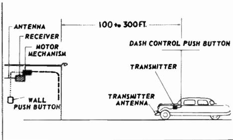
Transmitter installation diagram. Tube's filament is warm when car's ignition is on, but transmitter sends out signal only when push button is pressed.
