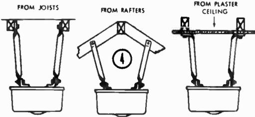
4. The method of installing pipe hangers for the motor depends on the construction of your garage.
