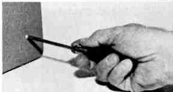
A spring-blade screwdriver, or a regular screwdriver with screw-holding attachment is invaluable for places that are too crowded for fingers.
