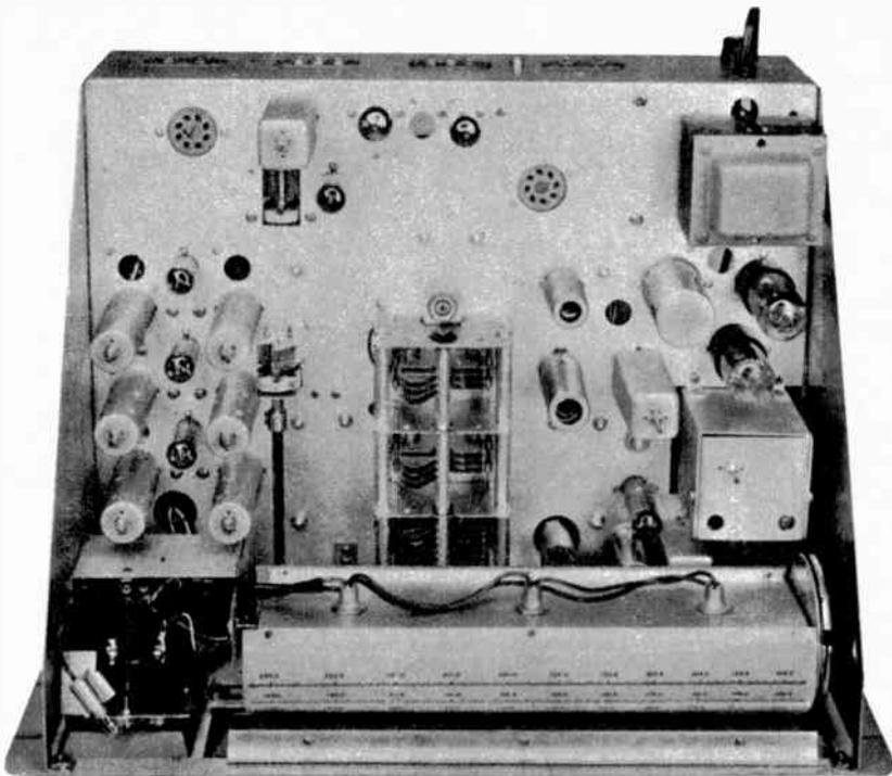
Large drum dial of NC-300, which turns as band switch is turned, is well illuminated by three lights set into it, as evident in chassis view above. Empty sockets at the rear are for connection of optional accessories such as 100-kilocycle crystal calibrator, converters, etc. The underside of chassis, shown in photograph below, is crowded but orderly. The chassis slips out of the cabinet readily for inspection.
