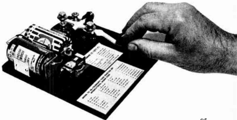
wiring in picture form; right schematic equivalent of picture diagram. Directly below, finger points to tiny transistor that is used as tone oscillator. Knob above key adjusts tone pitch. Ear-phones connect to binding posts at bottom right of same picture. Photo lower right shows underside of complete transistor oscillator. The holes in peg-board are very convenient for passing wires. The unit comes in kit form. Lafayette Radio, NYC 13.
