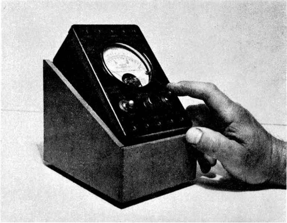
A circuit tester is easier to read when in an inclined position and much less likely to fall over or be pulled over on its face. Here a small Weston Model 697 meter has been fitted with a simple box made of plywood scraps. Bottom of box has "feet" of rubber-head tacks which discourage it from sliding.
