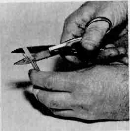
The job of trimming copper braid from connector cables, a nuisance with pliers, takes minutes with scissors. High-grade scissors hold their cutting edges for a surprisingly long period of time, as the thin wire of the copper braid is very soft.
