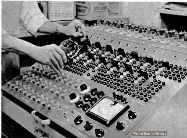
The angled cabinet has been designed to make the entire front face of the computer simple to operate, as demonstrated here by Chalmer Jones, assistant to the president of the Heath Company.
