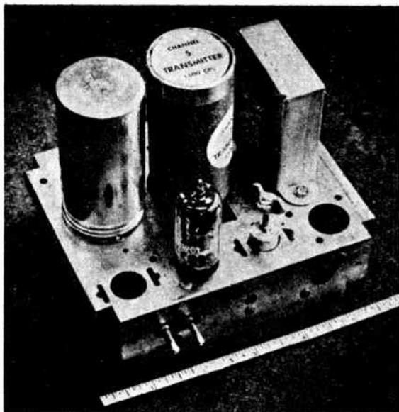
Chassis view of transmitter. Only one tube is used, and operation is dependable. Round unit in center is channel selector which is replaceable.
