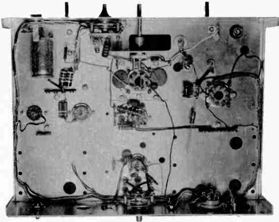
The photograph above affords an under view of the DX-35 transmitter's chassis with some of the small parts as well as a small portion of the wiring in position. The photo below shows the underside of the completed chassis. The box, lower center of the picture, is shield for components of oscillator section.
