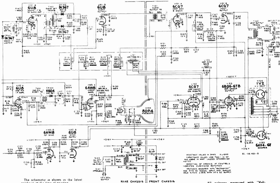
The schematic is shown in the latest condition at the time of printing. All resistance value in ohms. K = 1000
