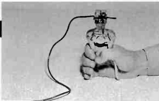
. . . and squeeze the handles. Wire remains clamped in the left jaw. Right jaw, containing cutters, moves outward and strips off the insulation. One set of cutters accommodates four sizes of wire.
