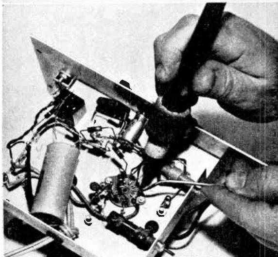
Pencil-type iron is indispensable for making or loosening connections in tight spots like this.
