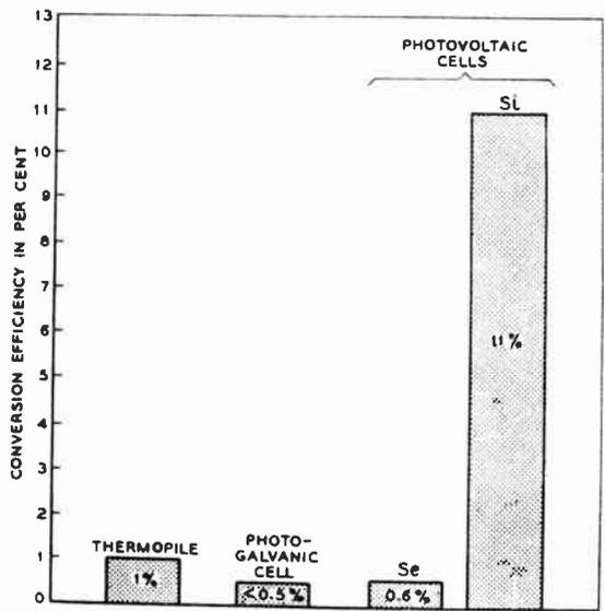
Fig. 1. Relative efficiencies of various devices for converting sun's rays to electrical energy.
