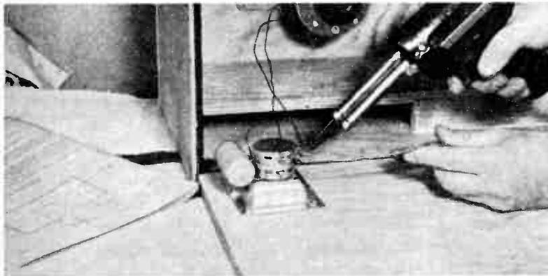
24. With back cover close to box, final speaker connections are made to terminal plate.
