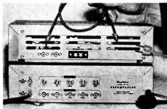
Back view of FM tuner stacked atop pre-amplifier. Connection between the two is made by shielded cable with plug fittings. Large plug at lower right connects pre-amp to main power amplifier.
