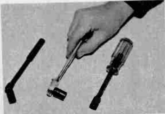
The three handles of the socket wrench set give a choice of driving angles. Ratchet handle, in center, is reversible for forward or back action with same motion. The angled handles afford great leverage; be very careful not to overtighten nuts.
