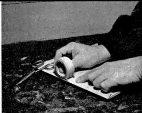
2. First step is to run masking tape along beveled edges to protect them from glue squeezed out of joints as members are joined. Glue remaining on wood makes the final finishing very difficult.
