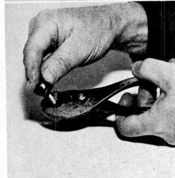
Serrated jaws of slip-joint pliers are designed to grip round objects. This tool is most useful for bolts, antenna rods, instrument shafts, etc.
