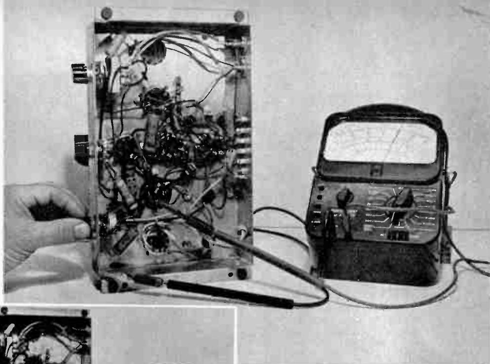
It is often desirable to have meter connected while adjustments are made in equipment under test. With equipment turned off, attach positive lead with snap-on alligator clip, just as with the negative lead, thus leaving both hands free.
