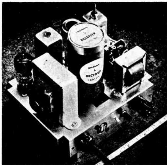
Chassis view of the receiver which contains two tubes and is similar in appearance to transmitter.
