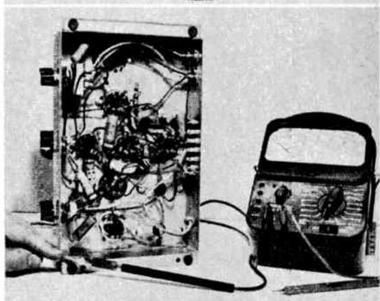
Holding positive test probe well away from its exposed metal end, test voltage by touching latter to appropriate point in circuit. One-hand method practically eliminates danger of shock. (Turn page.)
