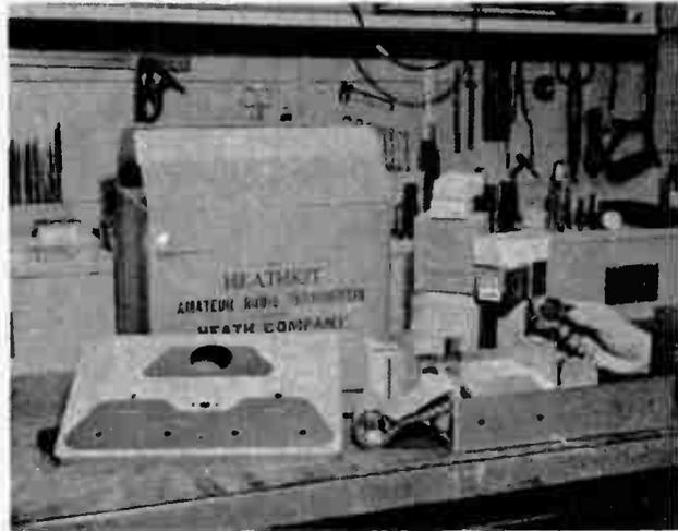
Chassis with major parts mounted. The large hole in its center is for 5146 power amplifier tube.
