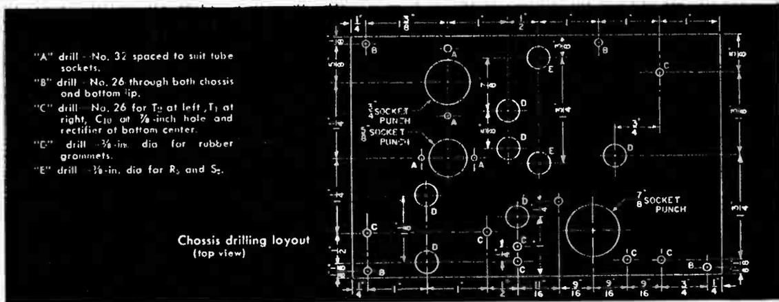
the chassis at the places shown in the bottom view, page 139, when the transformers and sockets are assembled with 6-32 x  $1/4$ -inch and 4-40 x  $1/4$ -inch machine screws. Soldering lugs are also placed on these screws for ground tie-points. Rubber grommets are used in the six  $3/8$ -inch diameter holes marked "D" where leads from the transformers, switches and volume control pass through the chassis.
