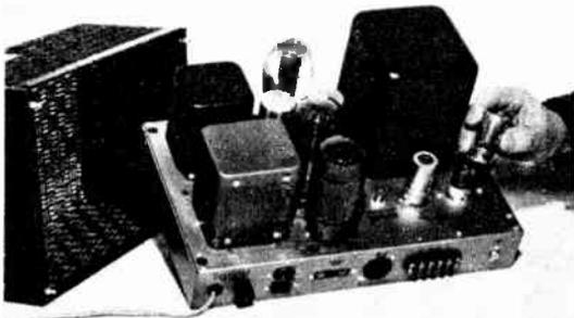
Hardware-cloth steel cover protects the chassis of the Heathkit W-5M amplifier, above left, and allows ventilation of hot tubes. Finger points to protective fuse in holder. All connections are made to bottom apron. The cover is readily removable, left. Large, heavy transformers provide its power-handling capacity. Wiring of the W-5M hi-fi amplifier is relatively simple as evident in schematic diagram and photograph directly above. The cylindrical units are capacitors.
