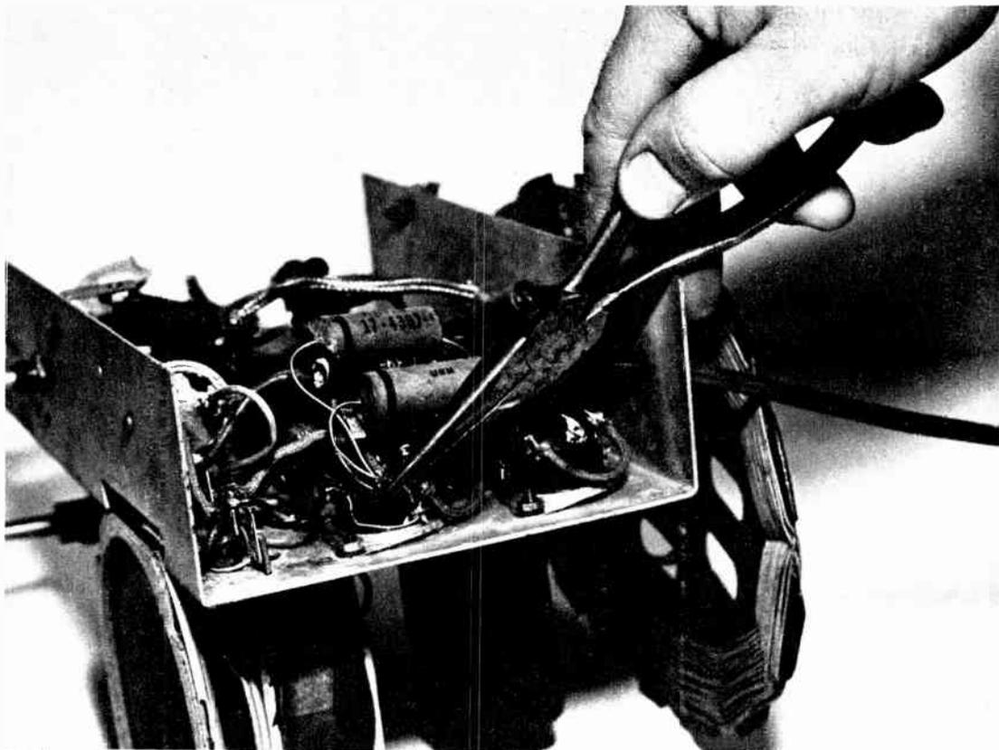
Long-nose pliers are for light bending and holding. Use them especially to place wires in the holes of soldering lugs and terminals and avoid the use of fingers for the purpose. Oil of skin may make soldering joint difficult or impossible.
