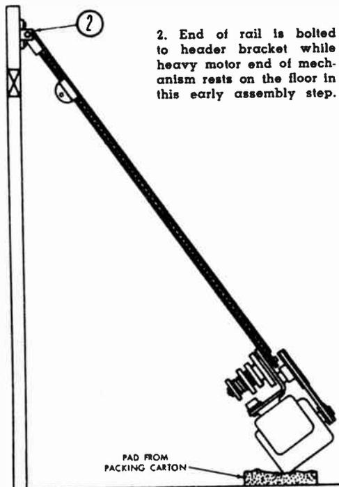
2. End of rail is bolted to header bracket while heavy motor end of mechanism rests on the floor in this early assembly step.
