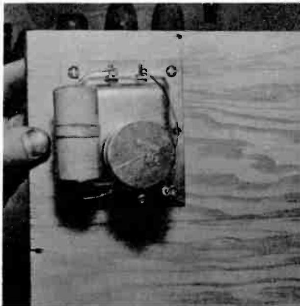
22. The rubber strips act as an acoustical seal. In this photograph, the terminal plate is mounted on back surface of back cover of the speaker box.
