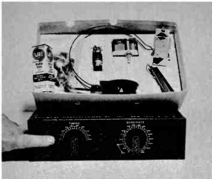
Components for one-tube battery set are in the upper box section. Finger points to scales printed on the outer section of the box.
