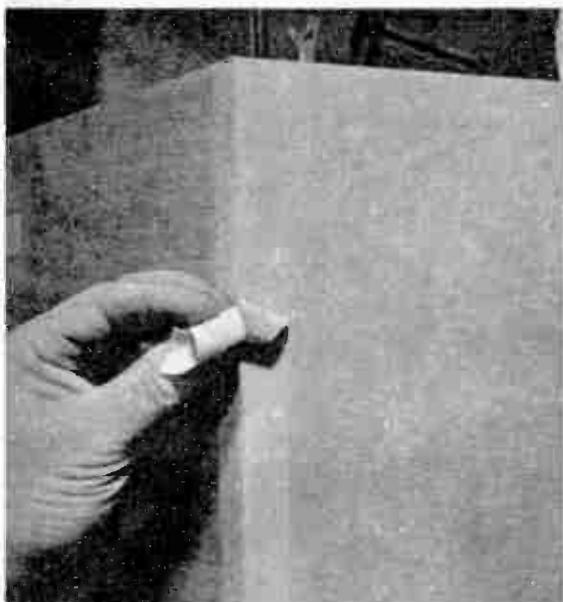
9. After glue has set, masking tape is stripped away. The corner joints are now tight and sharp.
