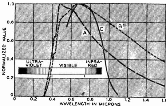
Fig. 6 (diagram directly above). A—solar energy distribution; B—solar photon distribution; C—short-circuit response, of the silicon solar cell.
