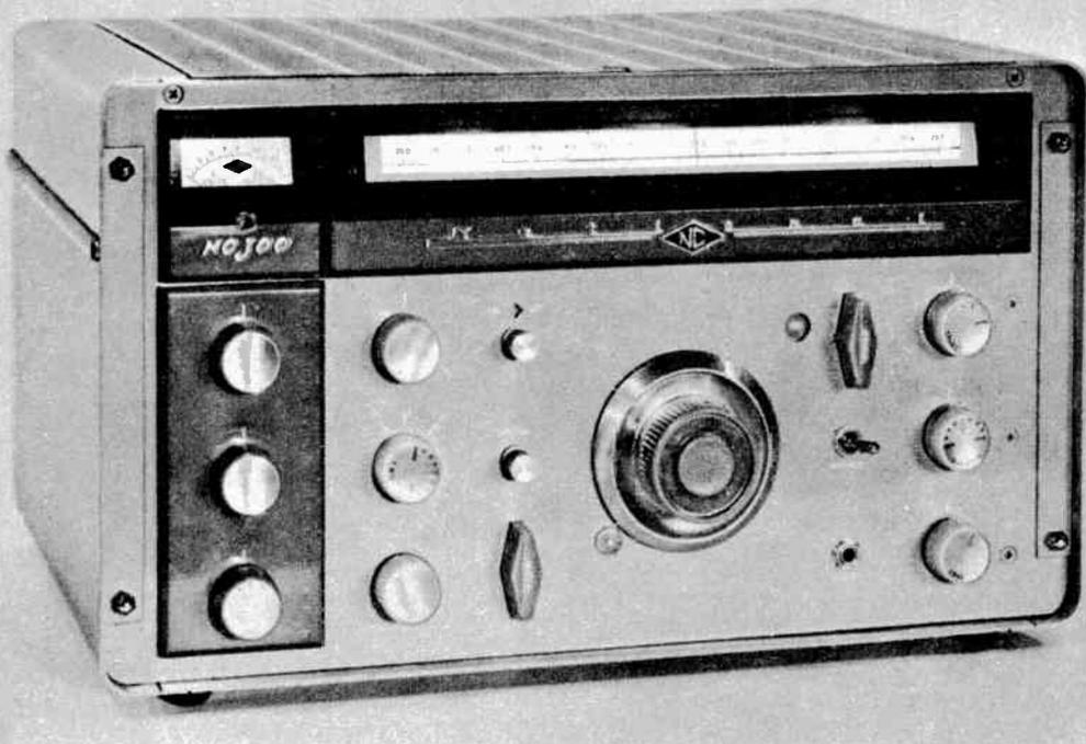
Large tuning knob in center of the National NC-300 receiver moves pointer over the drum dial at its top.
