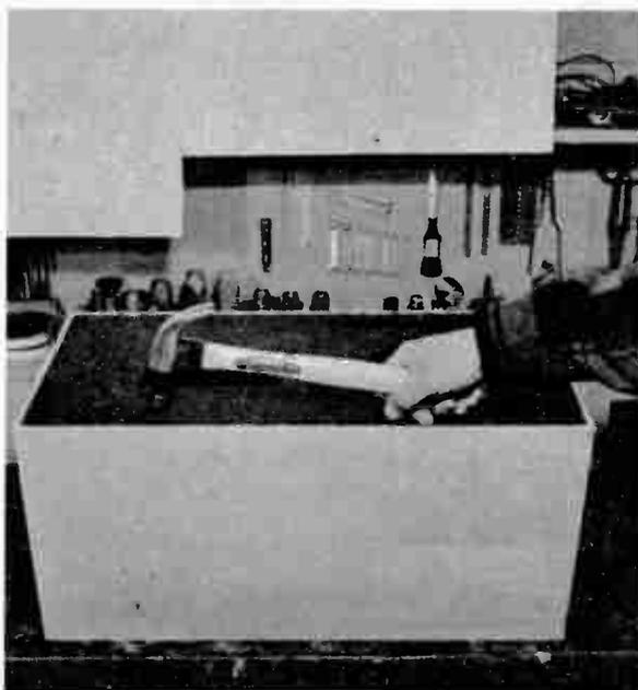
12. Dropping snugly against the recessed lips of the box, the speaker board is securely fastened with a series of closely spaced finishing nails.
