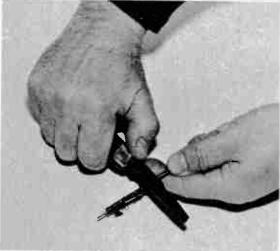
With the insulation off, scrape wire clean with the BACK edge of the blade, to avoid nicking.
