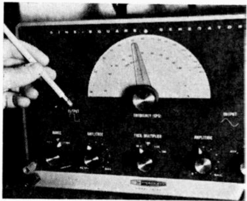
On Heathkit 1G-82 Sine-Square Generator front-panel controls are marked with output wave form. Pencil points to square wave.
