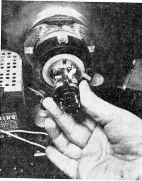
First loosen wing nut, then slide off yoke clamp. (In many sets this will be ion-trap magnet held by a spring around tube neck.)
