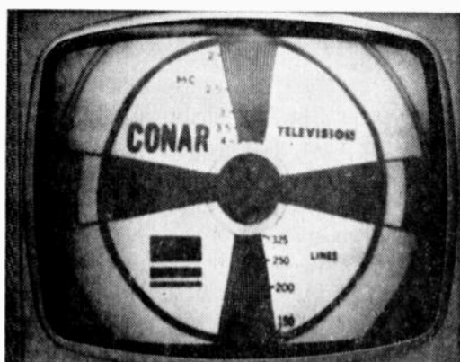
Fig. 5. Excessive contrast results in loss of picture detail and subtler gray shadings.
