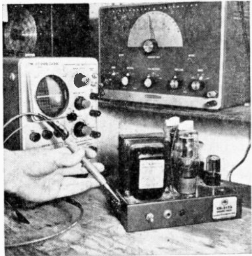
Fig. 6. Heathkit Model 1G-82 Sine-Square Generator and Tektronix 317 Oscilloscope being used to check output of hi-fi amplifier.
