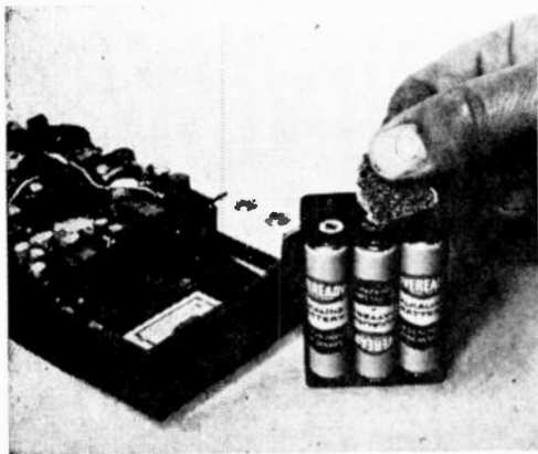
Corrosion on battery-holder terminals leads to intermittent operation, particularly if W-T is used around salt water; best cure is to sand off corrosion with fine sandpaper. Above, always check batteries under load, since output voltage can vary greatly. Batteries here registered 9V with no load, 8V on receive, 4V on transmit.
