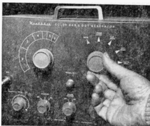
Fig. 11. Color generator is tuned to frequency of an empty channel and set to generate dots.
