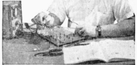
Transistor experiments on programmed breadboard— using oscilloscope.
