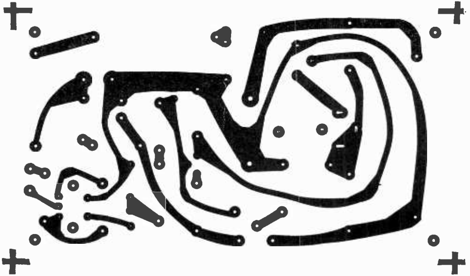
Fig. 2. Actual-size printed circuit board. You can make the board yourself or purchase it (see Parts List). If you make your own board, drill the holes as shown.
