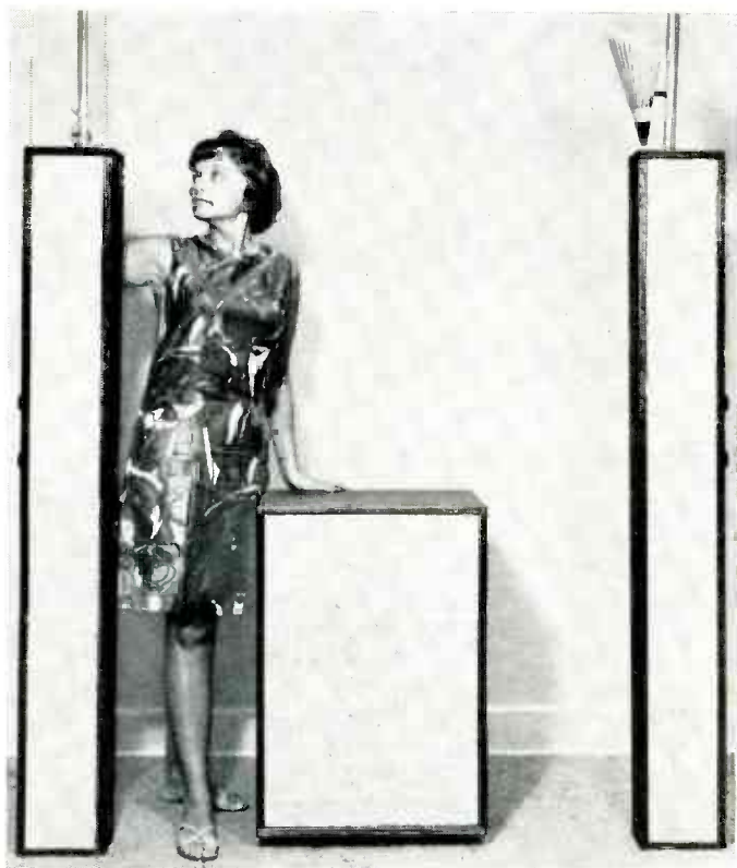
The mixed-signal woofer in this design was located in the squat box shown in the center of the photo. The "totem poles" on each side contained the satellite speakers.
