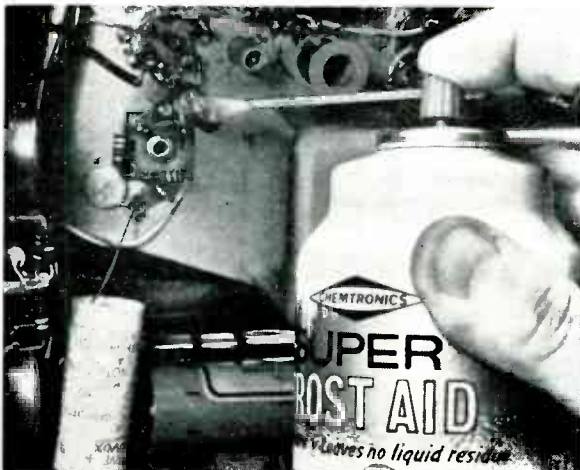
Loss of gain and erratic operation resulted from manufacturing defect in by-pass capacitor. Tipoff was gradual loss of signal after receiver had been in operation for an hour. Cooling down suspect components with freezing spray quickly pin-pointed defective capacitor.
