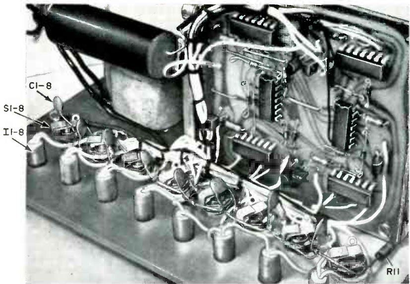
Construction is left to the builder. Here, the lamps, switches and capacitors are grouped in lines on the front panel. The PC board is mounted on a pair of brackets.
