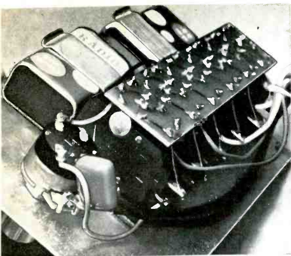
Fig. 7. Six normally open pushbutton switches are connected as shown here, one feeding each tone generator. Dc voltage comes from the same battery that powers the tone generator board.
