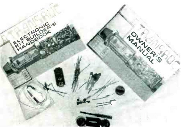
Several companies produce telemetry equipment for model rockets. Shown is Transroc, a kit operating on the Citizens Band with range of several miles paired with superhet receiver.
