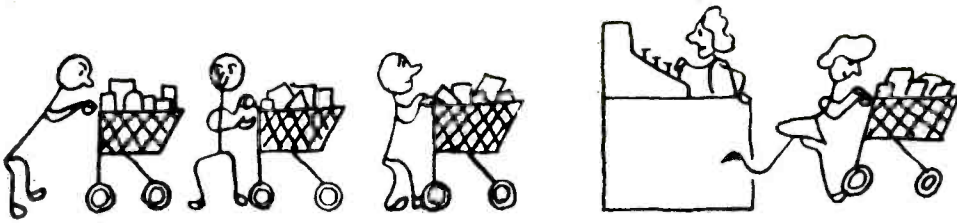
Fig. 3. Supermarket checkout counter can be used to explain "hole" flow in transistor.
