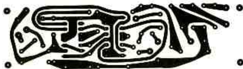
Fig. 2 Above is actual size foil pattern for the Prescaler circuit board. Component layout is shown at the left. Use low-power soldering iron and fine solder in the assembly.
