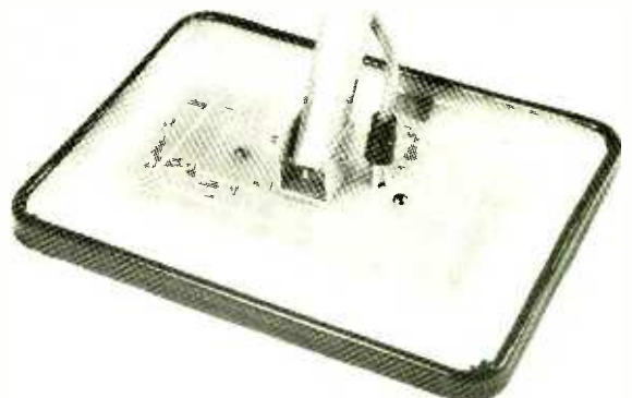
Fig. 5. The sensing coil is wound on plastic freezer container lid that is stiffened with Bakelite or phenolic. Phono jack is used to connect loop to oscillator cable.
