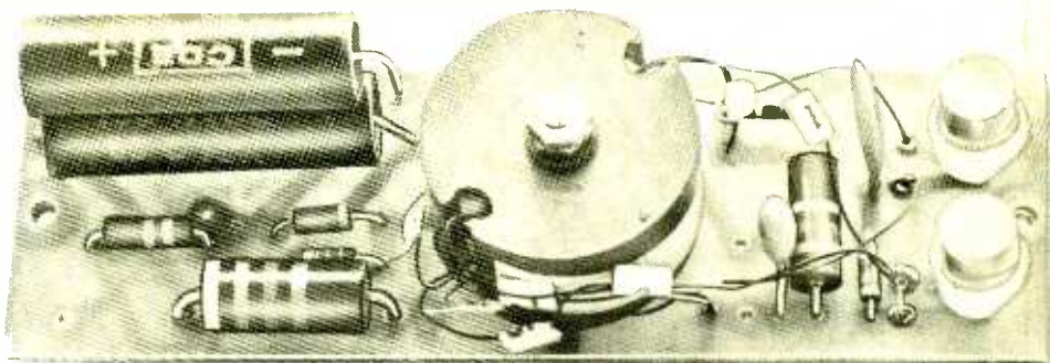
Fig. 3. Wired pc board assembly shows T1 mounted with hardware fiber washer. C4 is on top of C3.
