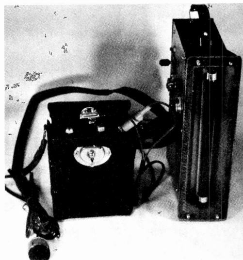
Batteries can be carried in cassette or binocular case with shoulder strap.
