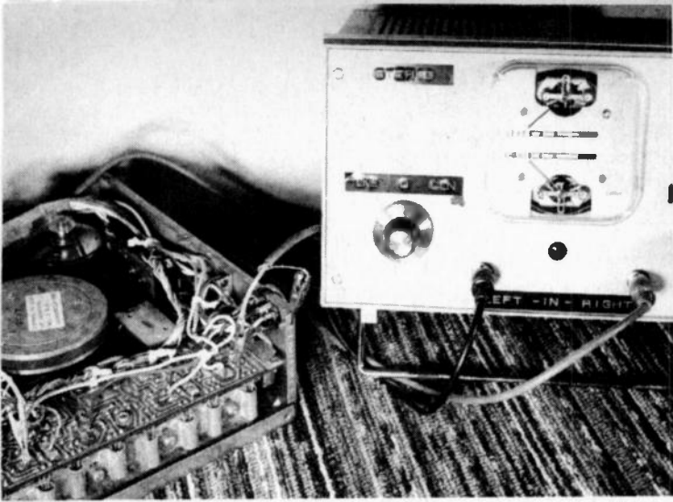
Figure 10. Locating the defective channel in a tape player.
