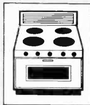
ELECTRIC RANGE 6–200 \mu T, MAJOR SOURCE OF MAGNETIC FIELD IS RESISTIVE HEATING ELEMENTS, DROP-OFF IS 1/r^3
