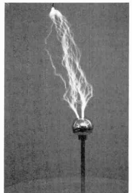
FIG. 8—THE SPARKS WILL JUMP even farther if a grounded electrode is placed near the discharge ball.
