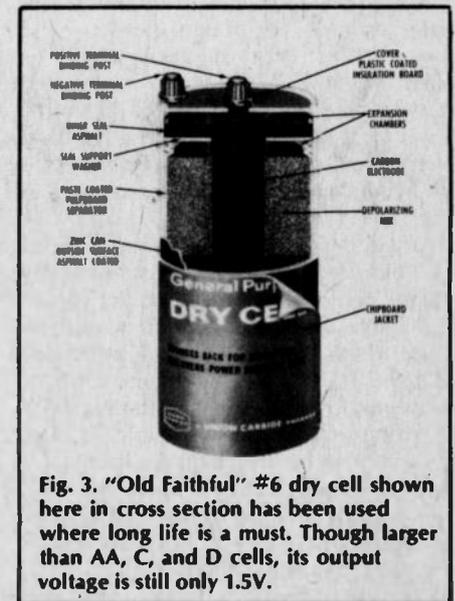
Fig. 3. "Old Faithful" #6 dry cell shown here in cross section has been used where long life is a must. Though larger than AA, C, and D cells, its output voltage is still only 1.5V.
