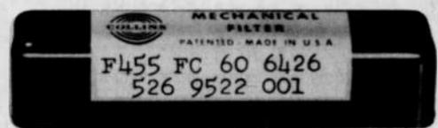
Fig. 7. This is the type of filter used to remove the unwanted sideband from the RF output signal.
