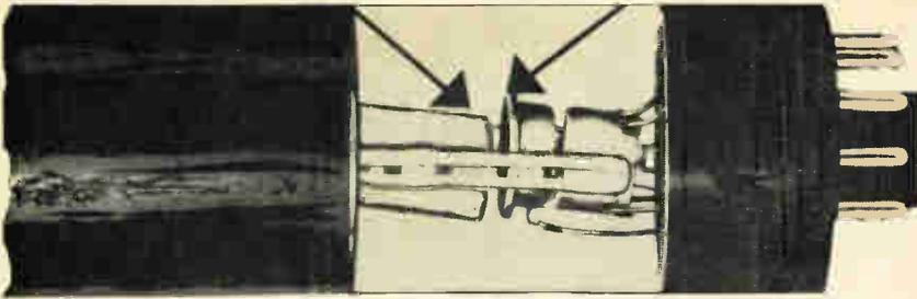
In one type of picture tube, a glow appears at the limiting aperture of the electron gun to signal any misadjustment of the ion trap. Arrows show the aperture at which glow appears
