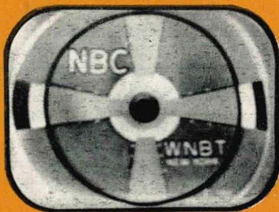
**Causes**—Focus control misadjusted, focus coil misadjusted, focus control or focus coil completely or partially shorted, ion trap misadjusted.
