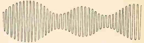
(B) AMPLITUDE-MODULATED WAVE
