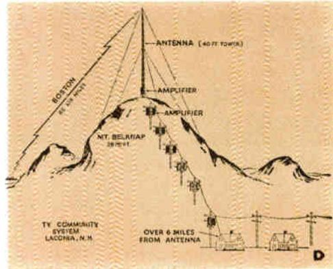
Community TV-antenna system, photo A, tapped to bring signal into a home. Photo B shows coaxial cable coming over and down a mountain. Tower amplifier station is shown in photo C. D illustrates system
