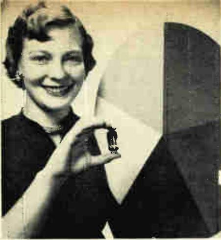
Above, tiny new receiving tube for color-TV sets regulates the brightness of the three primary colors on picture screen. The large wheel is televised in test patterns. Right, entire top of color-TV set lifts up for easy access to chassis
