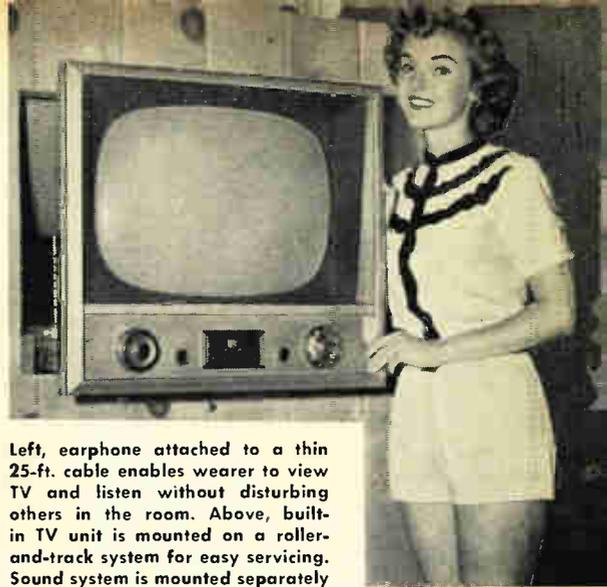
Left, earphone attached to a thin 25-ft. cable enables wearer to view TV and listen without disturbing others in the room. Above, built-in TV unit is mounted on a roller-and-track system for easy servicing. Sound system is mounted separately
