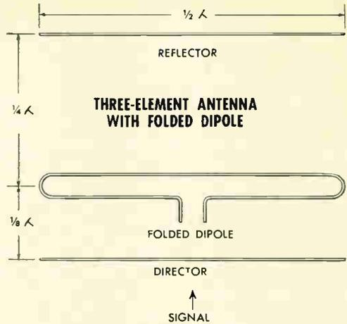
Left, this antenna is sensitive to signals from front. Above, sharp tuning is attained with folded dipole
