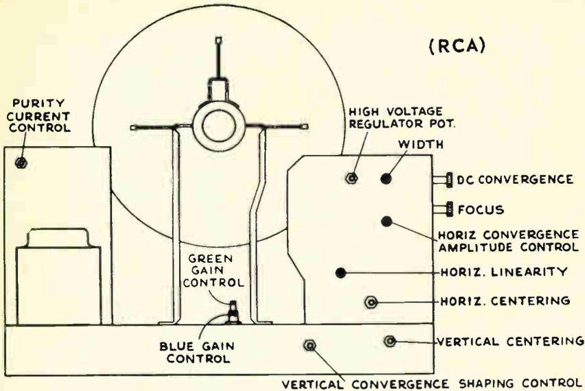
Diagram of rear apron panel shows additional controls necessary for color receiving
