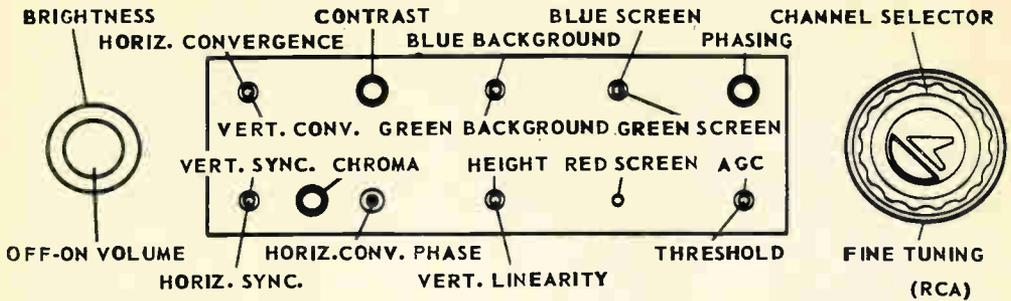
Front panel of RCA color-TV set has two more controls than black-and-white receiver
