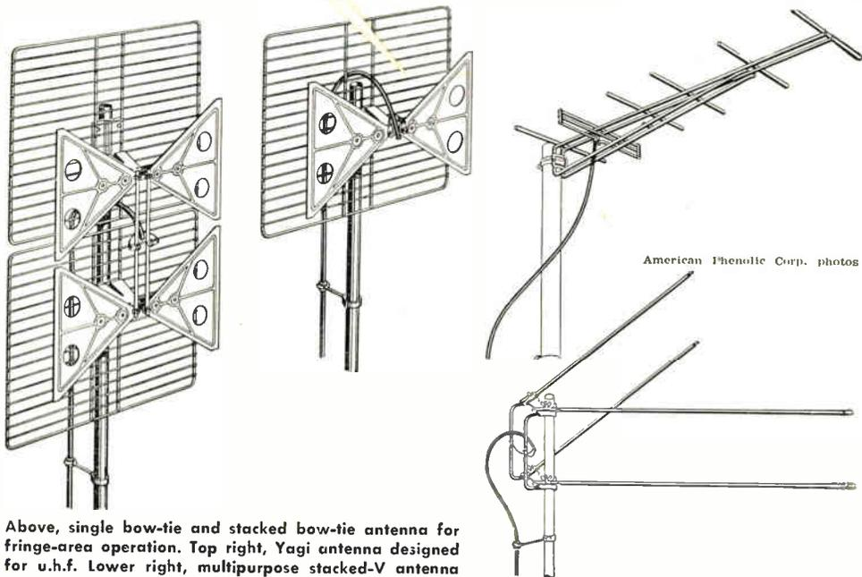
Above, single bow-tie and stacked bow-tie antenna for fringe-area operation. Top right, Yagi antenna designed for u.h.f. Lower right, multipurpose stacked-V antenna
