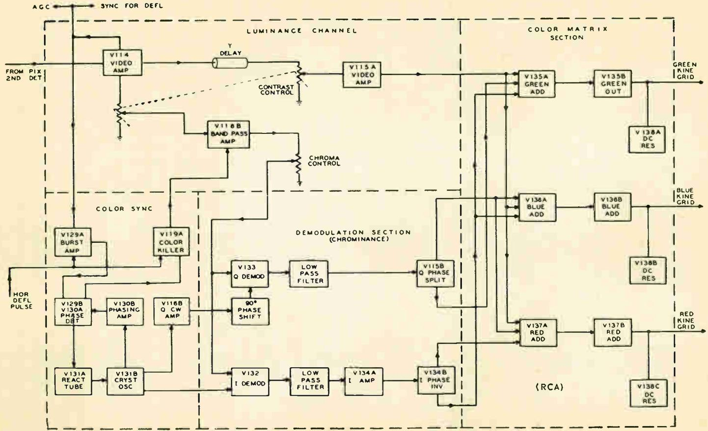
Video section of color receiver. Each block represents a tube, tube section or circuit
