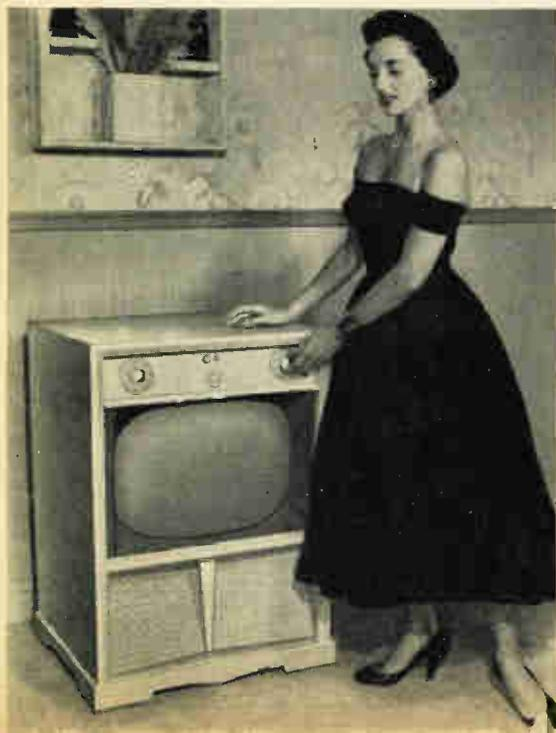
Left, recent improvements in TV sets include convenient top-panel tuning. Another feature of this receiver is the Unit-ized chassis which consists of individual plug-in units. Below, a decorative touch in indoor antennas. This type of antenna is claimed to provide ideal reception in city areas on all channels including VHF and UHF
