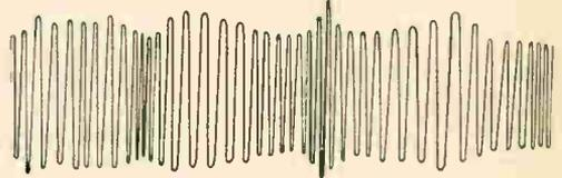
(C) FREQUENCY-MODULATED WAVE WITH AMPLITUDE AFFECTED BY INTERFERENCE
