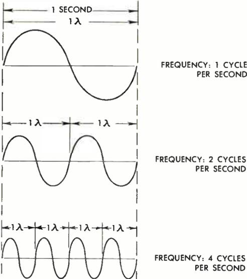
Note: The Greek letter "lambda" is used here as the symbol for wavelength. It will be noticed that the greater the number of cycles, the shorter the wavelength
