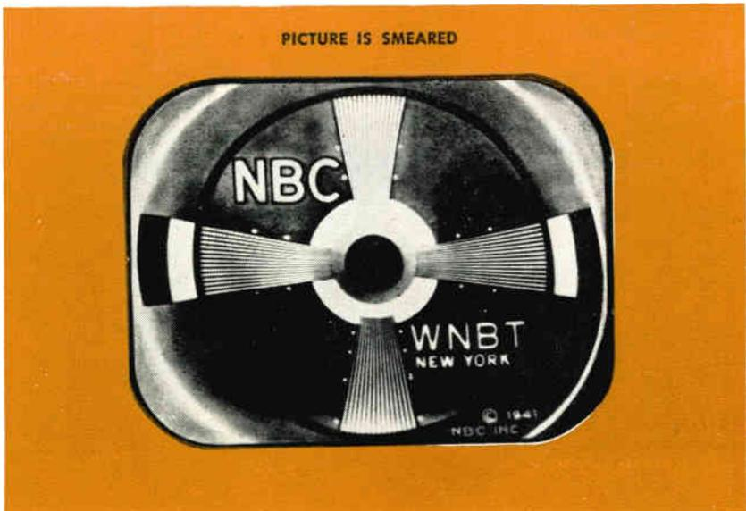
components are designed. Any defective part in these integrating and compensating networks can cause smearing. Occasionally, one of the video tubes will become slightly defective and give the same results.
