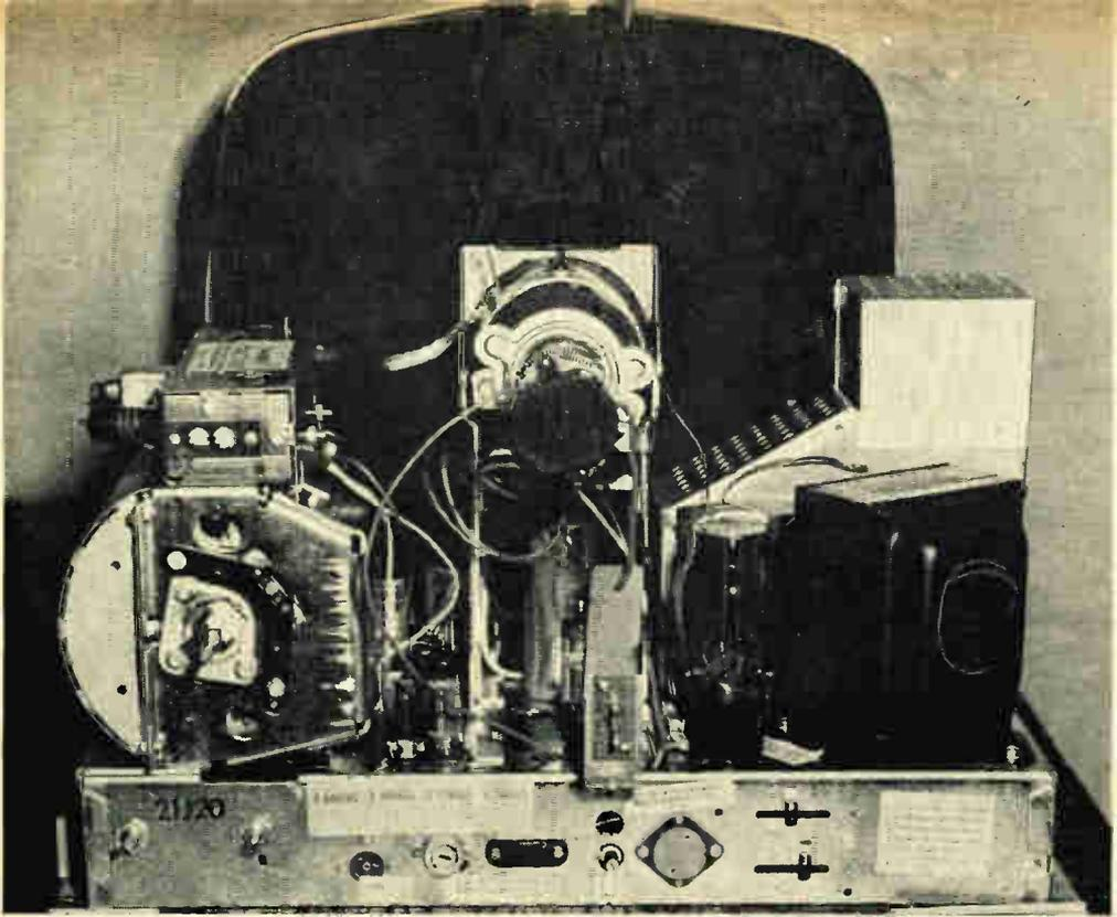
Secondary controls on most sets are behind the cabinet and adjusted with a screwdriver
