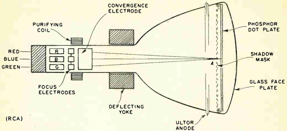
Operating components of the Tricolor Kinescope used in RCA color-television receivers
