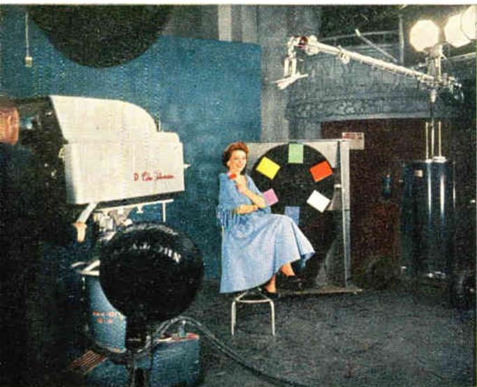
Before a telecast, each camera must be "tuned in" for delicate shadings of flesh tones. Here a cameraman focuses on a girl beside a color wheel to adjust camera for perfect color pickup
