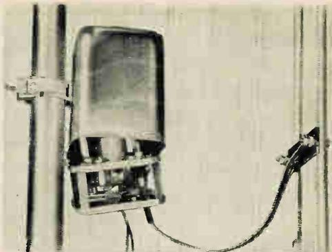
Signal booster mounted on antenna
