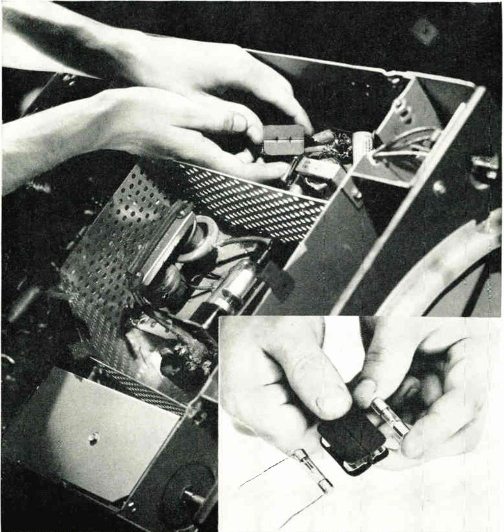
Danger points because of high-voltage buildups in your television set are illustrated on this and the following two pages. There will be no hazard, however, if you carefully "bleed" the current off these points by shorting them to the metal chassis of the receiver. Make a shorting tool like one shown in Fig. 22 on page 122. This picture series is excellent for familiarizing yourself with your TV set.
