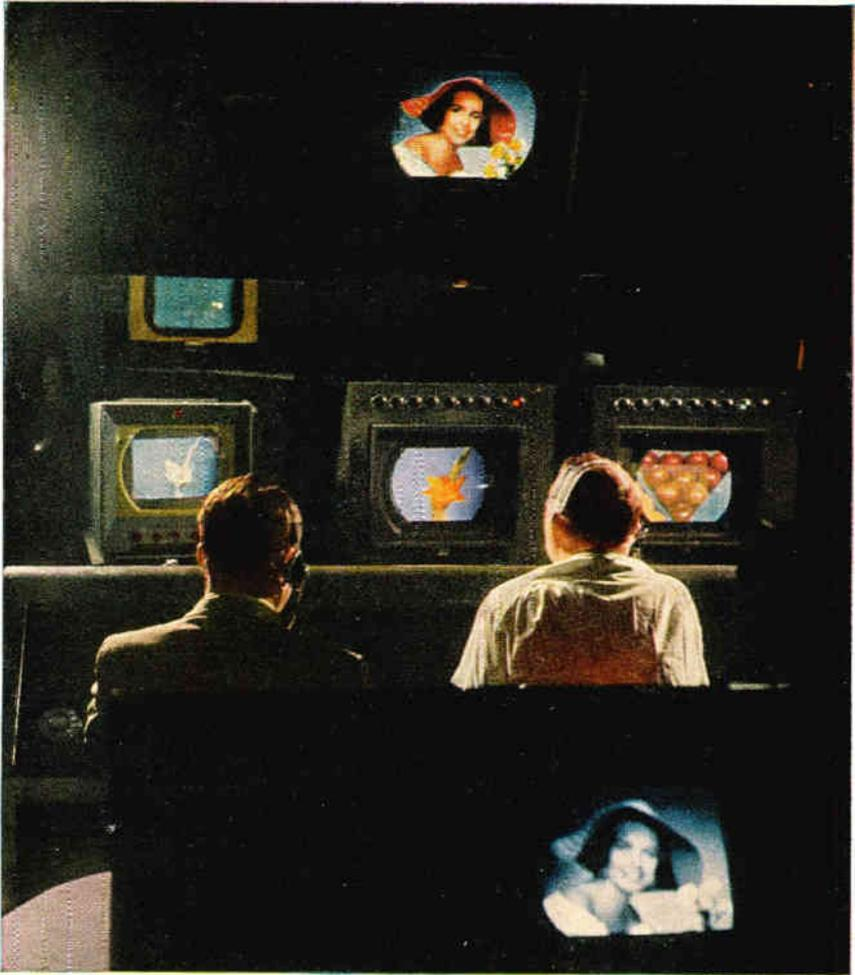
Control room during color telecast. Screen at lower right is black-and-white picture of scene in center, which is on the air. Engineer can switch on either of the other two scenes
