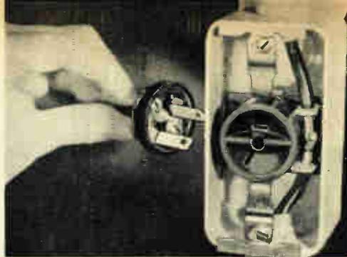
Left, primary controls are usually at the front of set. Right, tap-off device in master antenna system
