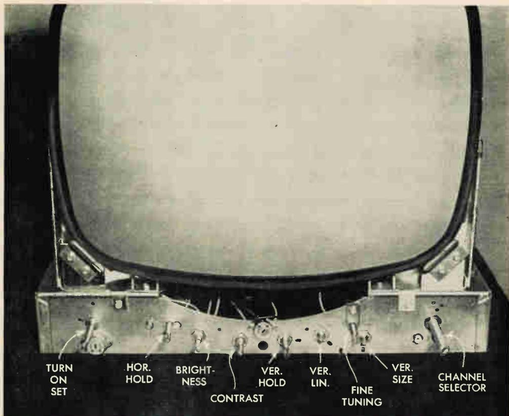
If the picture rolls around and around vertically, the vertical sweep circuit is not properly adjusted. To remedy this, make the necessary adjustment with the vertical hold control. Turn the control so that the picture is just barely drifting down. Then reverse the control slightly, moving the picture upwards, and it will snap into place.
