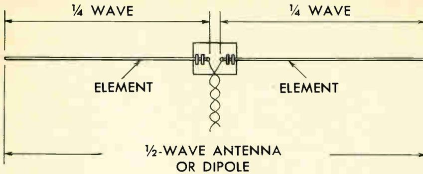
laid end to end about an inch apart. These elements are made of tubing, aluminum alloys being the most common materials because of their light weight, rigidity, weather resistance, etc. They are clamps at the ends of a block of insulating material such as Bakelite or one of the newer plastic compounds. A two-wire lead-in is connected, one wire to each element.
