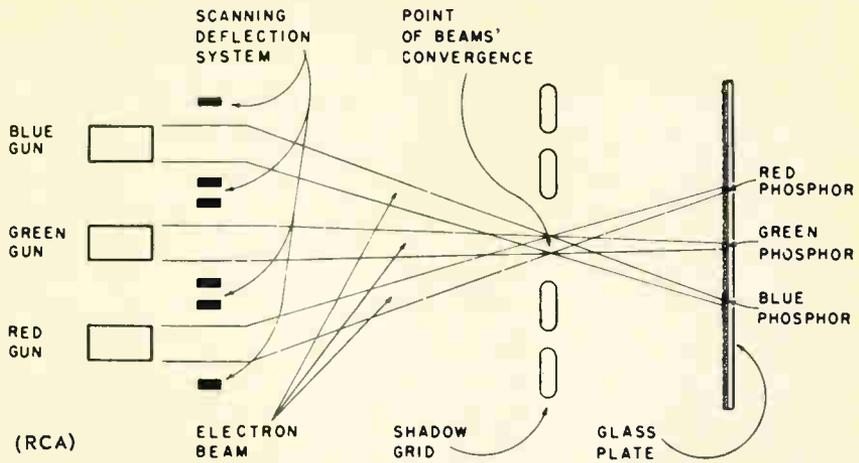
Shadow-mask line-scanning system uses picture screen dotted with the three primary colors
