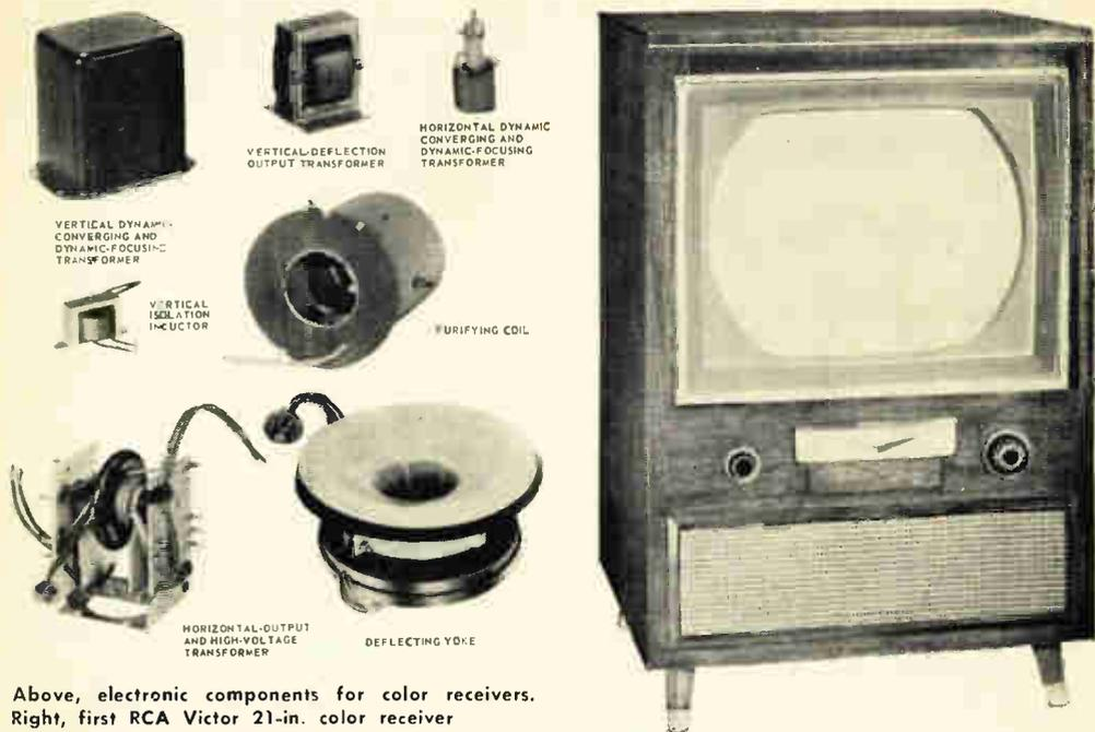
Above, electronic components for color receivers. Right, first RCA Victor 21-in. color receiver
