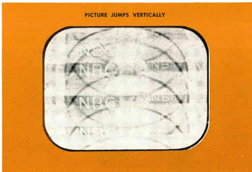
Replace vertical-sync-circuit tubes—sync clipper, sync separator, etc. Checking the filtering usually incurs a fair amount of signal tracing to find where alternating current may be entering the circuit.
