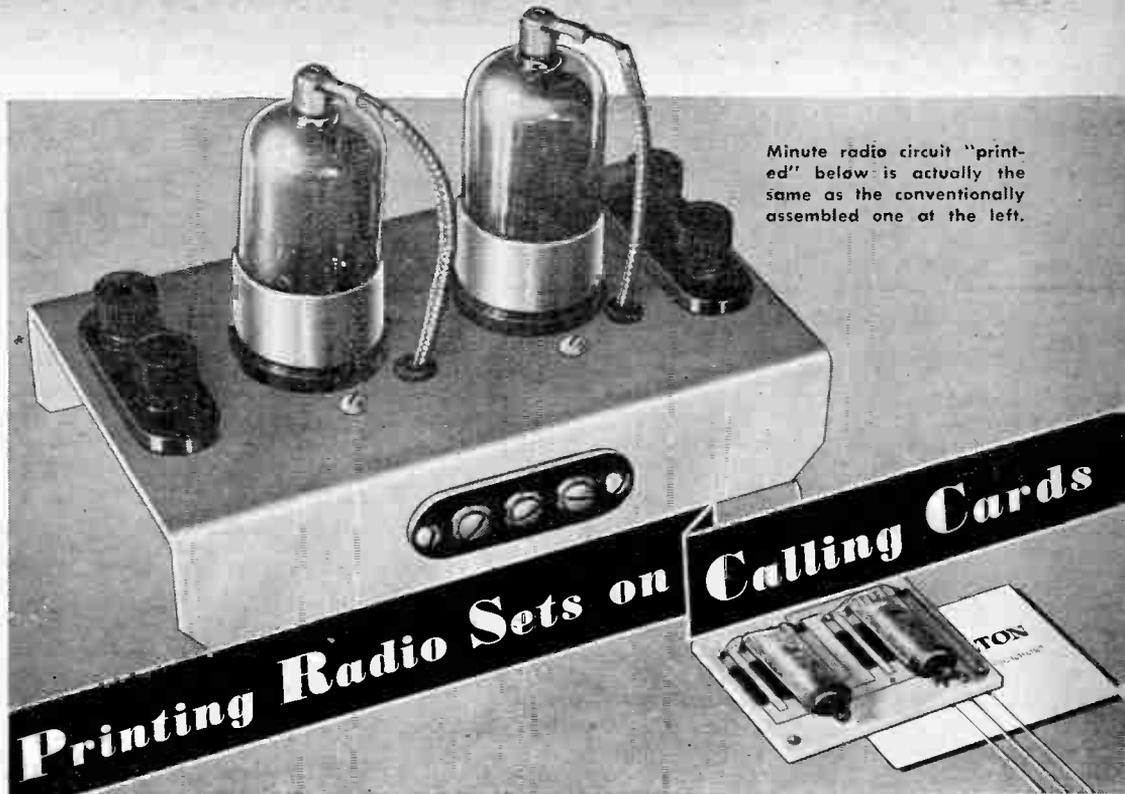
Minute radio circuit "printed" below is actually the same as the conventionally assembled one at the left.
