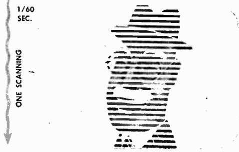
A second scanning, also taking 1/60 second, is needed to give a full image. This is called the "interlace." Scanning beam moves back and forth over spaces not covered first time. Consequently, the interlace lets you see parts of image you didn't see in first field. Sketches are exaggerated. Actually, there are at least 250 scanning lines in one field.
