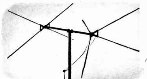
extremely important. It is roughly a tenth of a wavelength (one fifth the length of the dipole), but should be adjusted on the spot for best results. If this spacing is wrong, the secondary signals that the director shoves into the dipole will tend to cancel out the signal that the dipole picked up on its own hook, and the result will be a poor picture or no picture.
