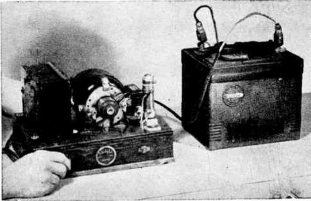
Connected to a house A.C. line, the homemade charger restores a battery at a rate up to 10 amp.
