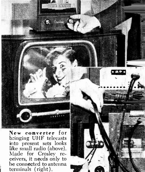
New converter for bringing UHF telecasts into present sets looks like small radio (above). Made for Crosley receivers, it needs only to be connected to antenna terminals (right).
