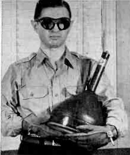
Protect yourself by wearing gloves and covering your eyes when you handle a picture tube. Hertzberg wears same goggles he uses when he sharpens tools on a power grinder.
