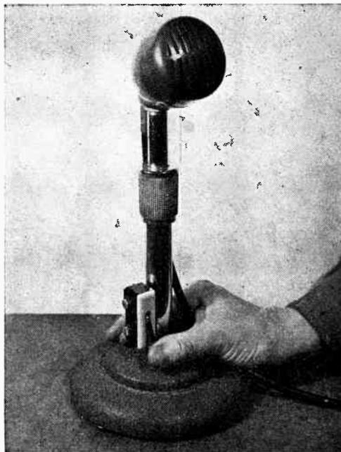
A push-to-talk control for an inexpensive microphone can be easily installed. Since it requires only very slight pressure, it can be kept shut for a long time without discomfort.
