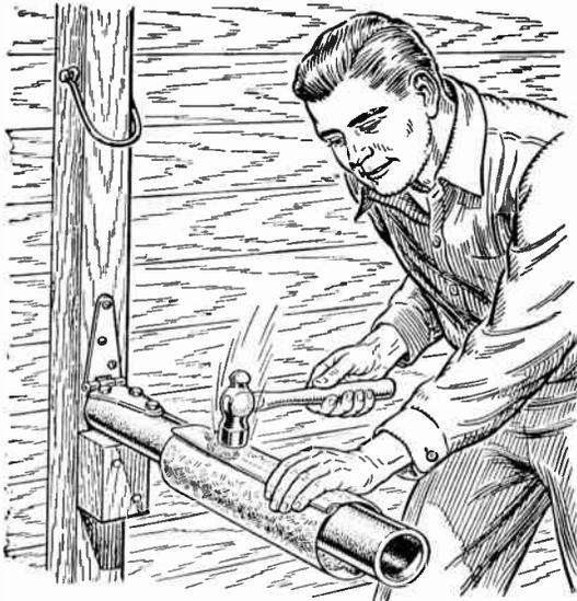
A PIECE of 4" pipe about three feet long mounted as shown can be used to form tubing from sheet metal. The hinge lets you swing it up out of the way when not in use. A block under the pipe adds rigidity.—*Ralph S. Wilkes, Keuka Park, N. Y.*
