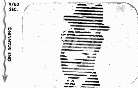
Each 1/60 second the scanning beam, a pin point of light, moves in slanting zigzag lines from top to bottom of tube. This produces a "field." As it moves, the beam momentarily records an image made up of tones ranging from black to wh<sup>ite</sup>. In a single field, your eye could see a recognizable image, but with spaces between lines picture would be incomplete.
