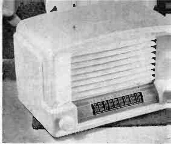
the receiver is held in place by the chassis screws. Make a plywood base slightly smaller than the radio bottom. Space the pivot and stop pins and three furniture glides to suit. A bolt and nut may be substituted for the pivot pin, but take care that it does not come into contact with the chassis.— *Glenn A. Wagner, Delmar, N. Y.*
