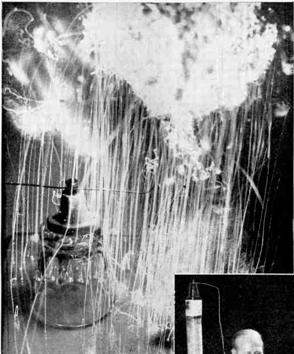
The stiff wire shown at the right carries the high voltage from the coil output to a wad of steel wool spread out on the loop. Can the steel wool take it? See above.
