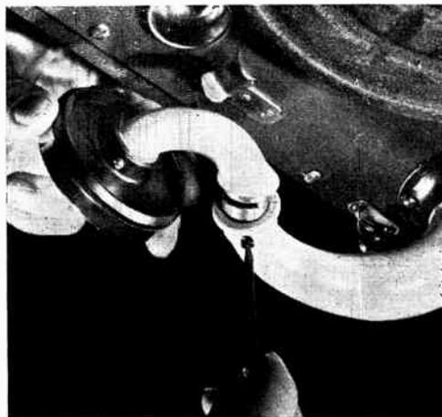
**Is the pickup head okay?** If not, it will either bottleneck the sound or bring it out sour. A damaged diaphragm causes distortion and loss of volume. Small dents may be pressed out.
