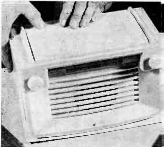
To locate the screw centers, cut a piece of paper the size of the plate, press it down, and transfer the imprinted marks for drilling.
