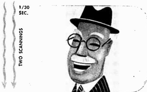
Complete TV image consists of two fields, one interlaced with the other. This is called a "frame." A new one is produced each 1/30 second. A succession of frames, one following the other without measurable delay, creates action you see. In effect, each frame is a still picture. Actually, there may be slight movement of image from one field to next.
