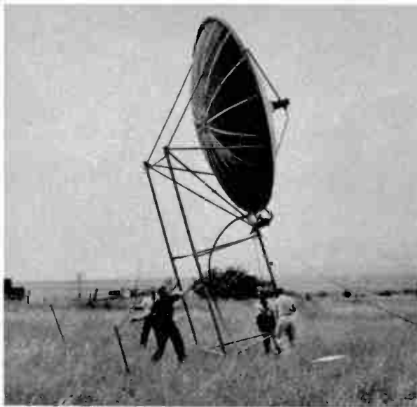
Those aren't supermen jockeying that huge antenna. Lightweight rig inflates with air, part of complete air-dropped radio system. Entire station includes two shelters, power unit, and antenna.
