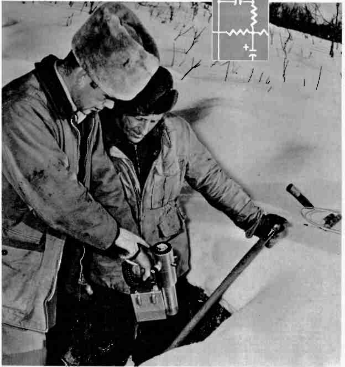
Radiation detectors and counters are among the many devices that require low-current high-voltage power sources. The uranium hunters above use a model made by Precision Radiation Instruments.
