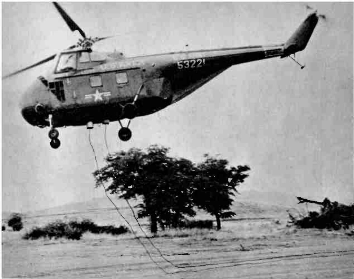
For certain military purposes, wire communication is preferred over radio. But the problem has always been how to lay sufficient wire fast enough. Here's a method that is proving successful at the Electronic Proving Ground. A 'copter at tree-top height spews out two lines at a mile a minute. Five hundred miles have been laid at speeds to 70 mph. Men in the "whirlybird" are in constant contact with the ground via field telephone, connected to the wires being laid. Two types of dispensers are seen below: cylinders that are outboard-mounted, photo at the left, and split pods that hold spliced reels.
