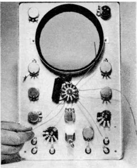
Rear view of O-11 panel with first parts mounted. These include variable resistors, switches, pilot light, ring support for face of cathode-ray tube. Some wires have been soldered to center switch.
