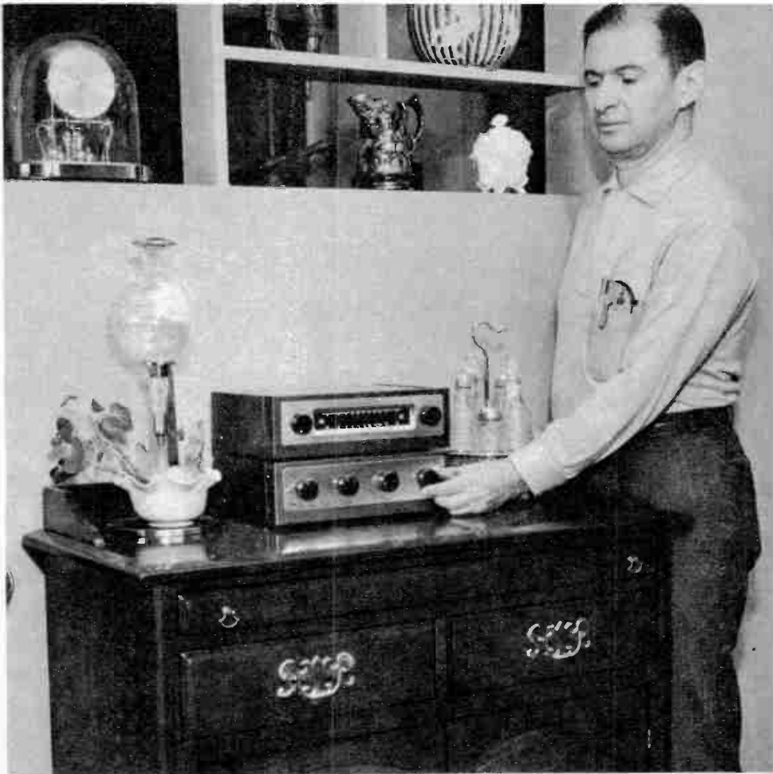
Serving table or buffet affords an attractive open spot for hi-fi units, leaving space for decorations, table accessories. Remember, in positioning amplifier, that it runs hot and requires adequate ventilation.
