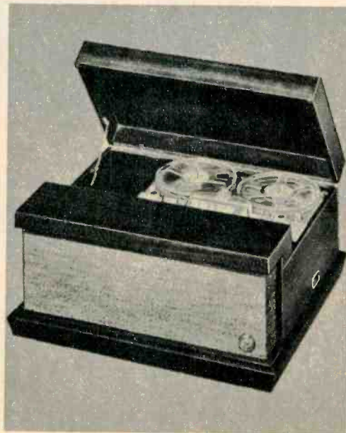
However, you can convert the Celeste recorder to stereo or 3-D sound by the addition of second speaker, second amplifier.
