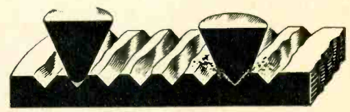
GOOD STYLUS PICKS UP HIGH FREQUENCIES; POOR ONE SKIPS THEM AND DAMAGES RECORD
