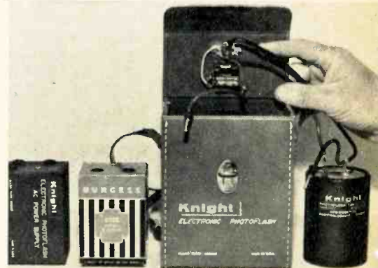
Parts of the shoulder-slung power source: case, with switch, outlet and safety resistor in flap; AC power unit; 300-volt dry battery and large storage capacitor.
