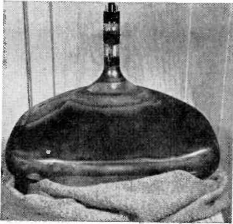
Avoid scratching face of old tube by placing on soft surface. Scratches increase danger of implosion and could affect trade-in value.
