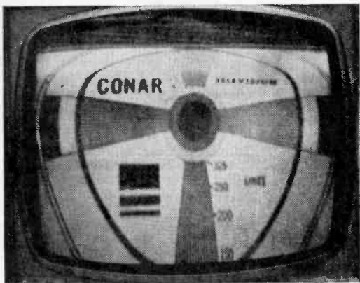
Fig. 24. Flat-topped circle can be made round again by adjusting both the vertical linearity and the vertical height controls together.
