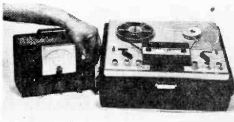
Align heads easily with test tape and VU meter across output (above)—be careful. Signal generator (below) feeds constant signal to recorder for head alignment.
