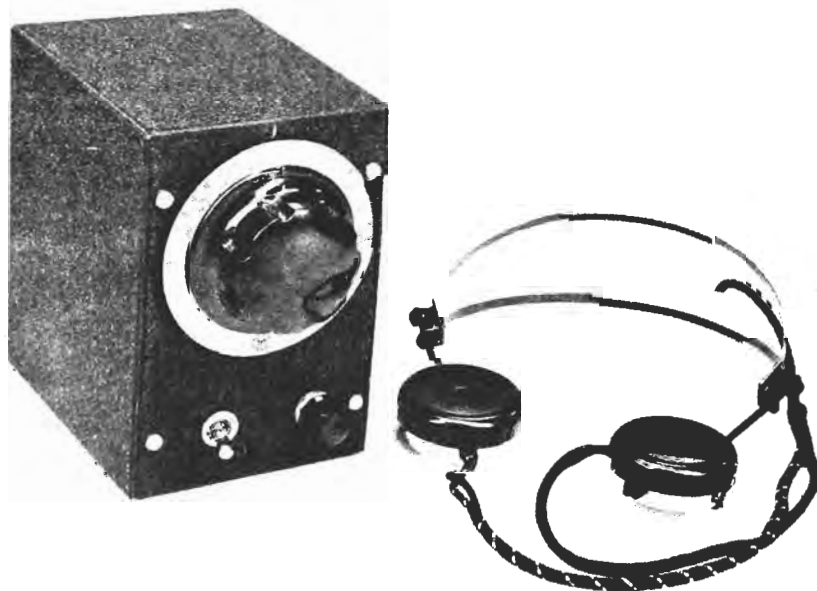
Over-all view of the experimental transistor receiver showing accessory headphones.
