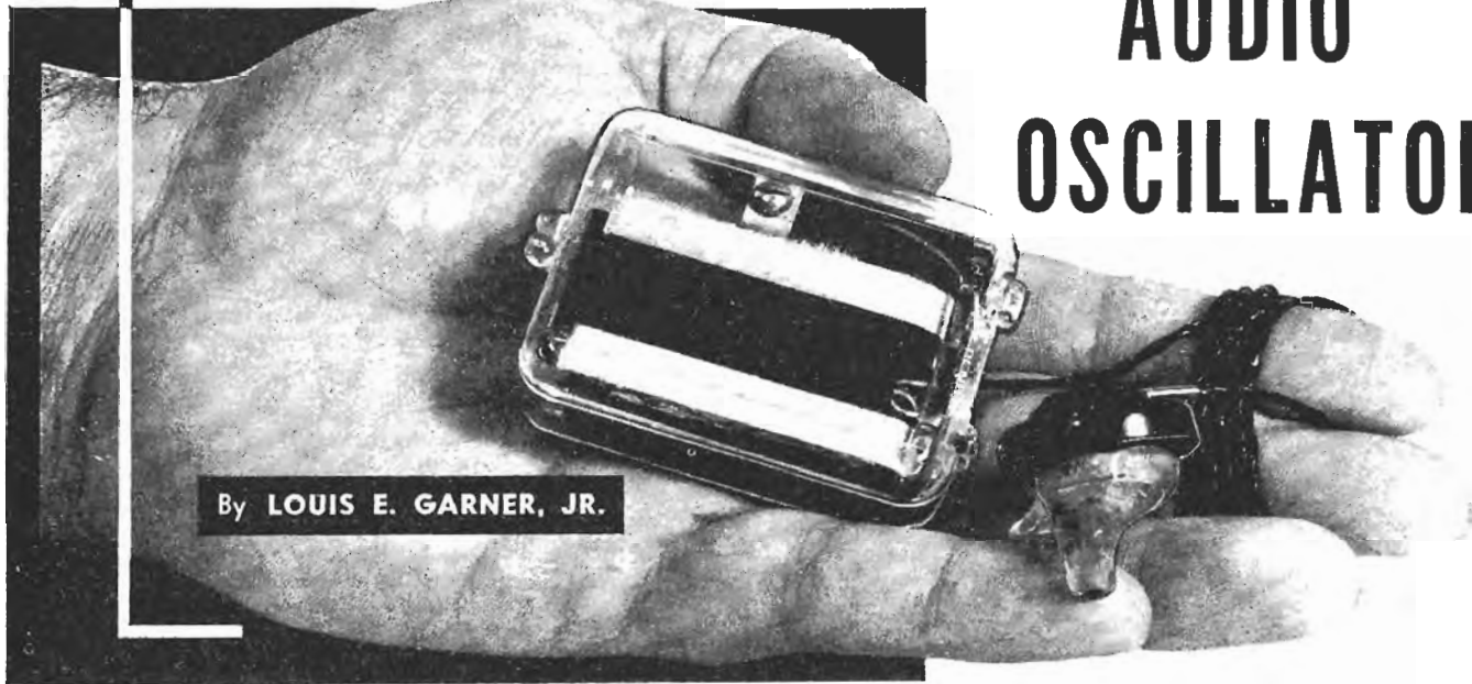
Fig. 1. "Light-powered" audio oscillator which is housed in tiny pill box.
