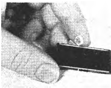
Fig. 5. Photocell used by author. Other sizes and shapes may be used. See text.
