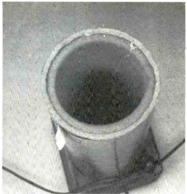
FIG. 3—LINE THE INSIDE OF THE TUBE WITH polyurethane foam. A piece of foam from a discarded mattress or sofa cushion will work just fine.
