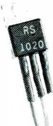
THE ZAP IS CONTROLLED BY AN SCR with extended leads. Note that the extension wires are insulated, and a short length of tubing is slipped over the wires and over the SCR leads.
