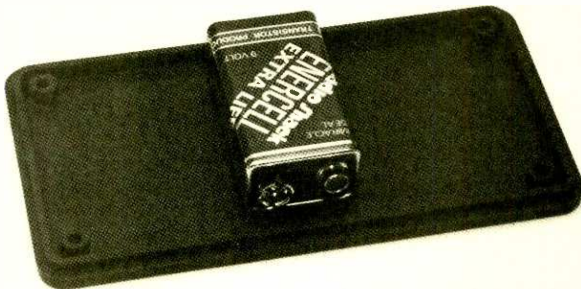
THE BATTERY is cemented to the case cover with a drop of RV adhesive. To replace battery, just pry up old unit with a knife or wide-blade screwdriver.
