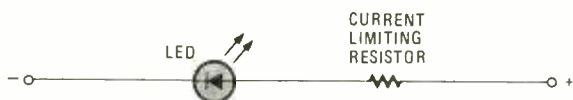
FIG. 1—HERE'S A TYPICAL light-emitting diode (LED) circuit that usually draws approximately 20 milliAmperes. The LED light is on continuously when power is supplied, causing a severe battery drain when left running over night. Often the pilot light consumes more power than the equipment itself would when left on after being used. What a way for a battery to go!
