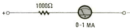
FIG. 1—THE TIME-HONORED voltmeter circuit that serves well in testing low-impedance voltage sources accurately. Ideally suitable for checking batteries, power supplies and low-impedance circuits. This is not the voltmeter to check low AGC voltages.
