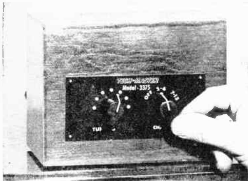
Semi-tunable type has switch for high or low band operation plus a fine-tuning adjustment.
