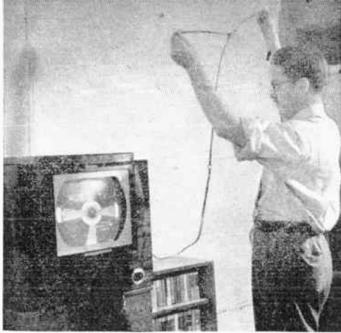
This one-channel antenna may actually surpass a roof antenna. Turn it to face the station.
