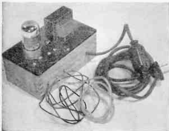
Top and bottom views of the panel of the A. V. C. unit show the set connections and wiring. The 2" high base is sawed from a small card-index cabinet
