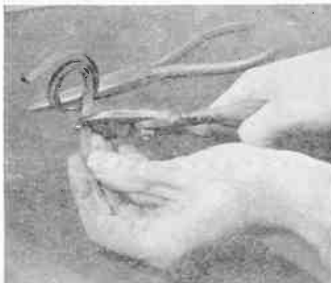
The bimetallic strip, cut from a thermostatic manifold control in a junked car, is pictured above, while the photo below shows the way it is mounted. At the left below, the operation of the device is indicated schematically. Directly at left is the circuit-breaking mechanism
