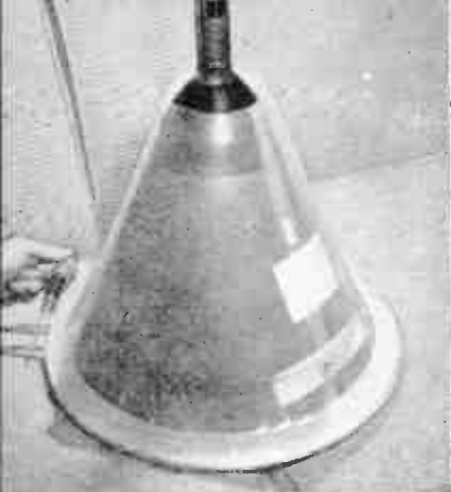
13 The entire metal shell of the 16AP4 is "hot," so it's wise to cover it with a plastic insulating hood and ring. The brackets I bought had a metal ring support.
