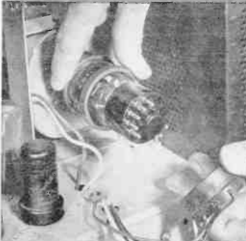
3. Tube socket and ion-trap magnet must come off—and be put back in same position.
