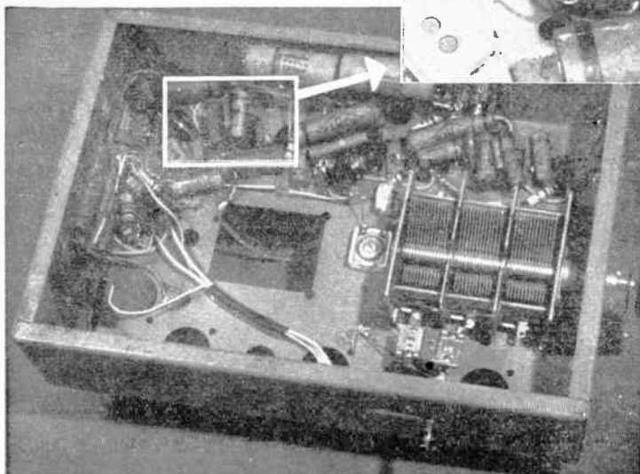
Wiring under the chassis of a receiver is a studied jumble. The close-up view above is that part shown within the square at left
