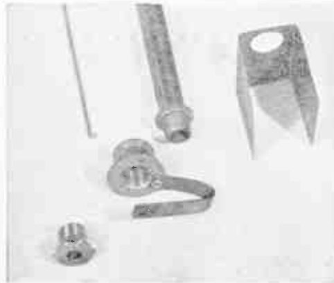
The bimetallic strip, cut from a thermostatic manifold control in a junked car, is pictured above, while the photo below shows the way it is mounted. At the left below, the operation of the device is indicated schematically. Directly at left is the circuit-breaking mechanism
