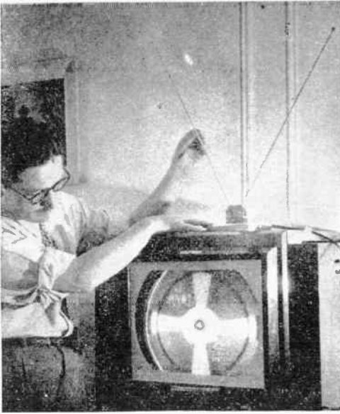
You can adjust the arms of this curtain-rod room antenna in direction, angle, and length.
