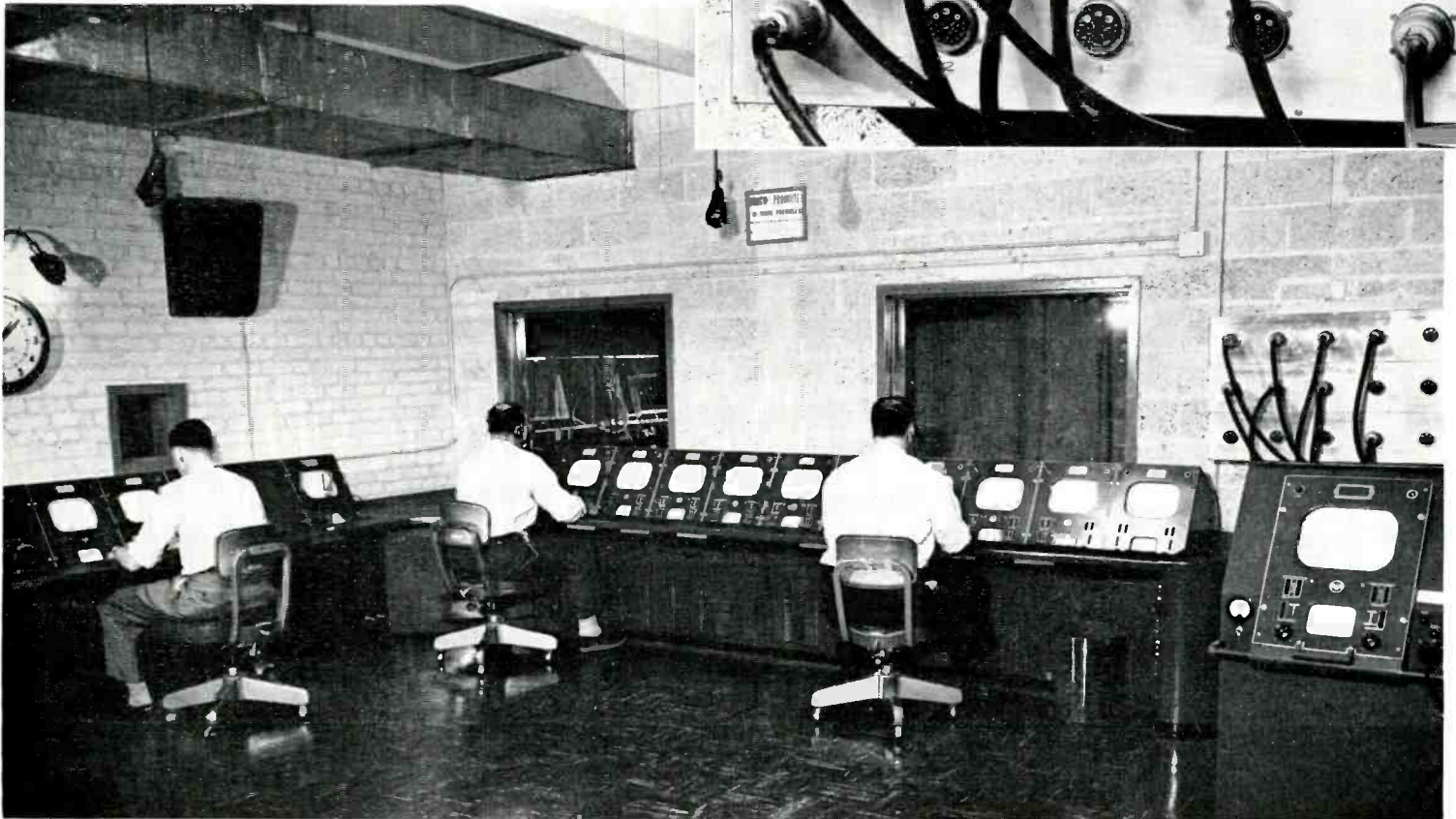
FIG. 29. The studio camera shading and monitor controls are centrally located in this console. At the extreme left part of the film shading and monitor controls are also visible.
