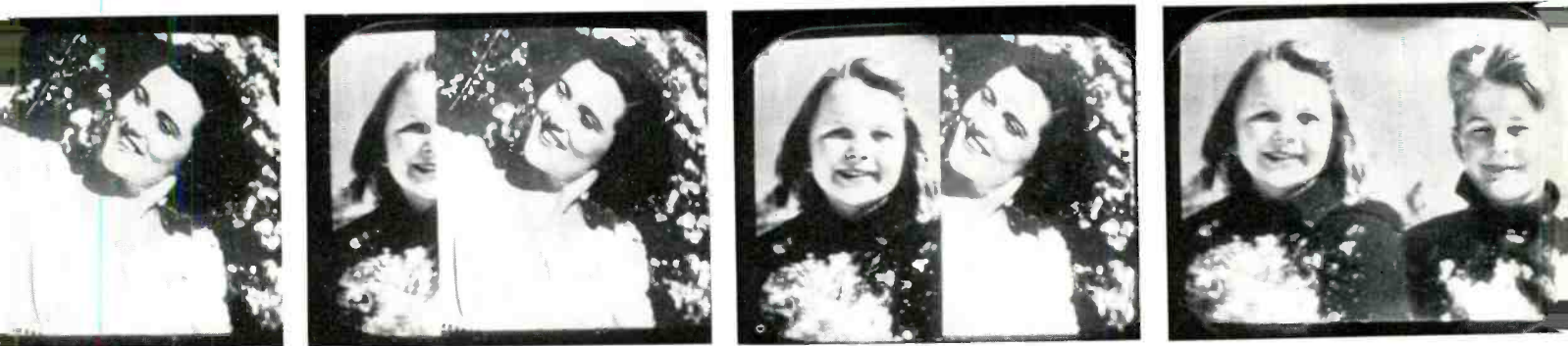
FIG. 9. These photos taken directly from the monitor screen illustrate how horizontal wipes may be used in progressive steps or continuously. Many arrangements can be made up from any two program sources.
