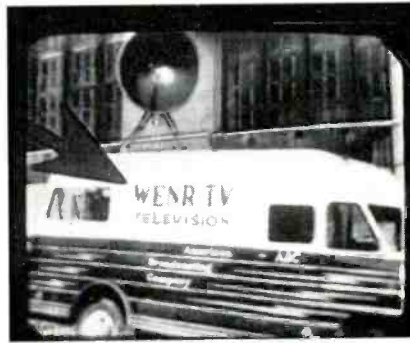
FIG. 12. In the pictures above the arrow or pointer is cut into the opaque mask. The background signal is black for these pictures and for those shown in Fig. 11.
