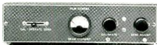
FIG. 4. Beam Current Metering Control Panel.
