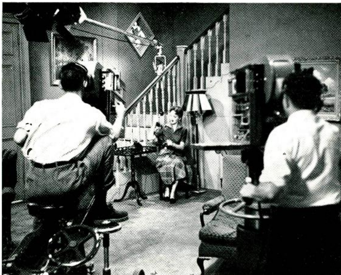
FIG. 9. Typical scene where boom must be raised rapidly from seated figure to rising position for wide-angle picture.
