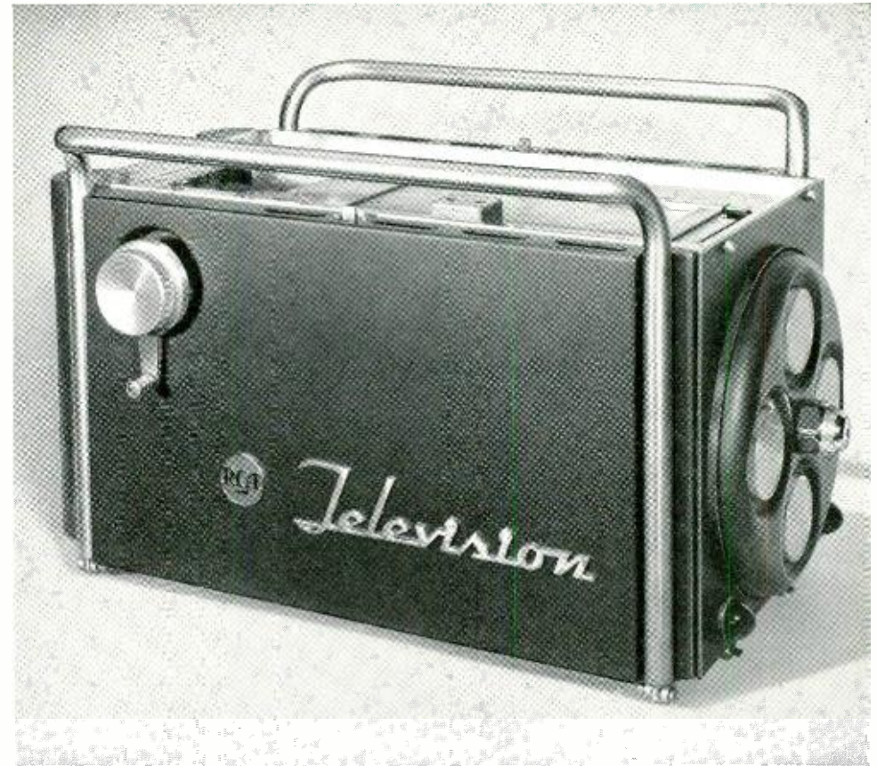
FIG. 6. Side view of camera with viewfinder removed. Note convenient carrying handles.
