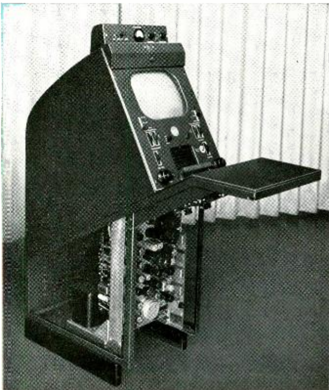
FIG. 3. Film Camera Control Chassis mounted below Master Monitor.
