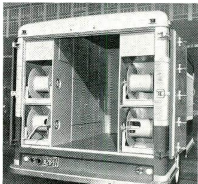
FIG. 4 (above). Rear view of the RCA TJ-53A Mobile Unit showing easy access to cable reels and compartment storage areas. Note convenient steps leading to roof area.
