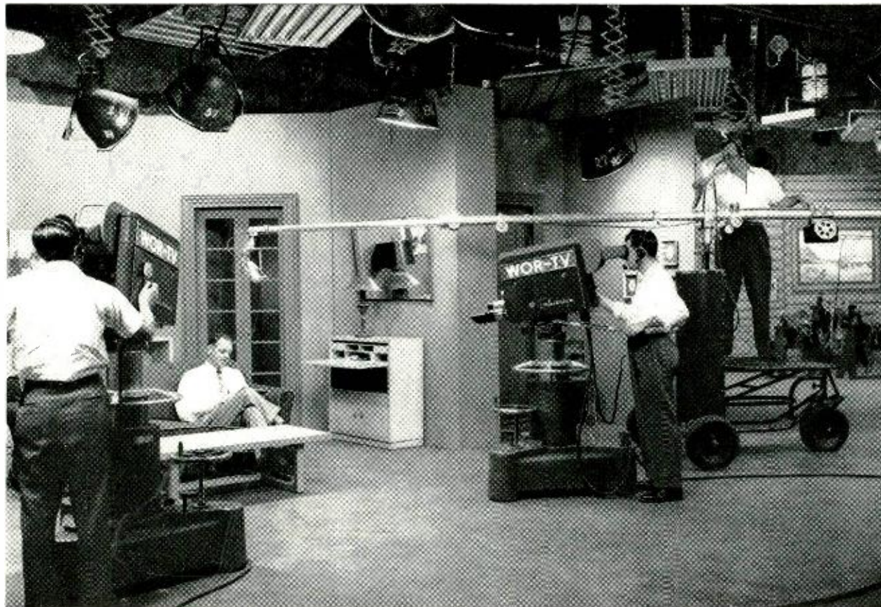
FIG. 8. Microphone boom MI-26574 using an RCA 77-D microphone.
