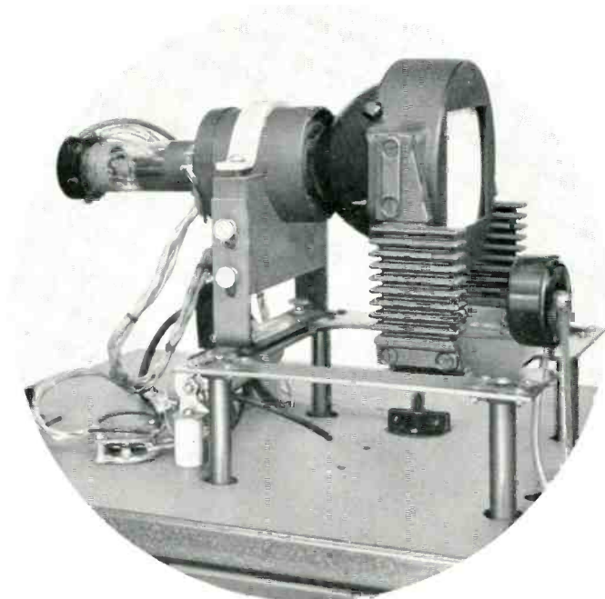
FIG. 7. Picture above shows the television projection tube assembly with the kinescope shield removed. Shown are the projection kinescope, RCA Type 5WP11, the kinescope and deflection yoke assemblies, and the insulator tube supports. The photonic cell mounted at extreme right of kinescope face is connected with meter in control panel and provides a relative indication of the tube's light output.
