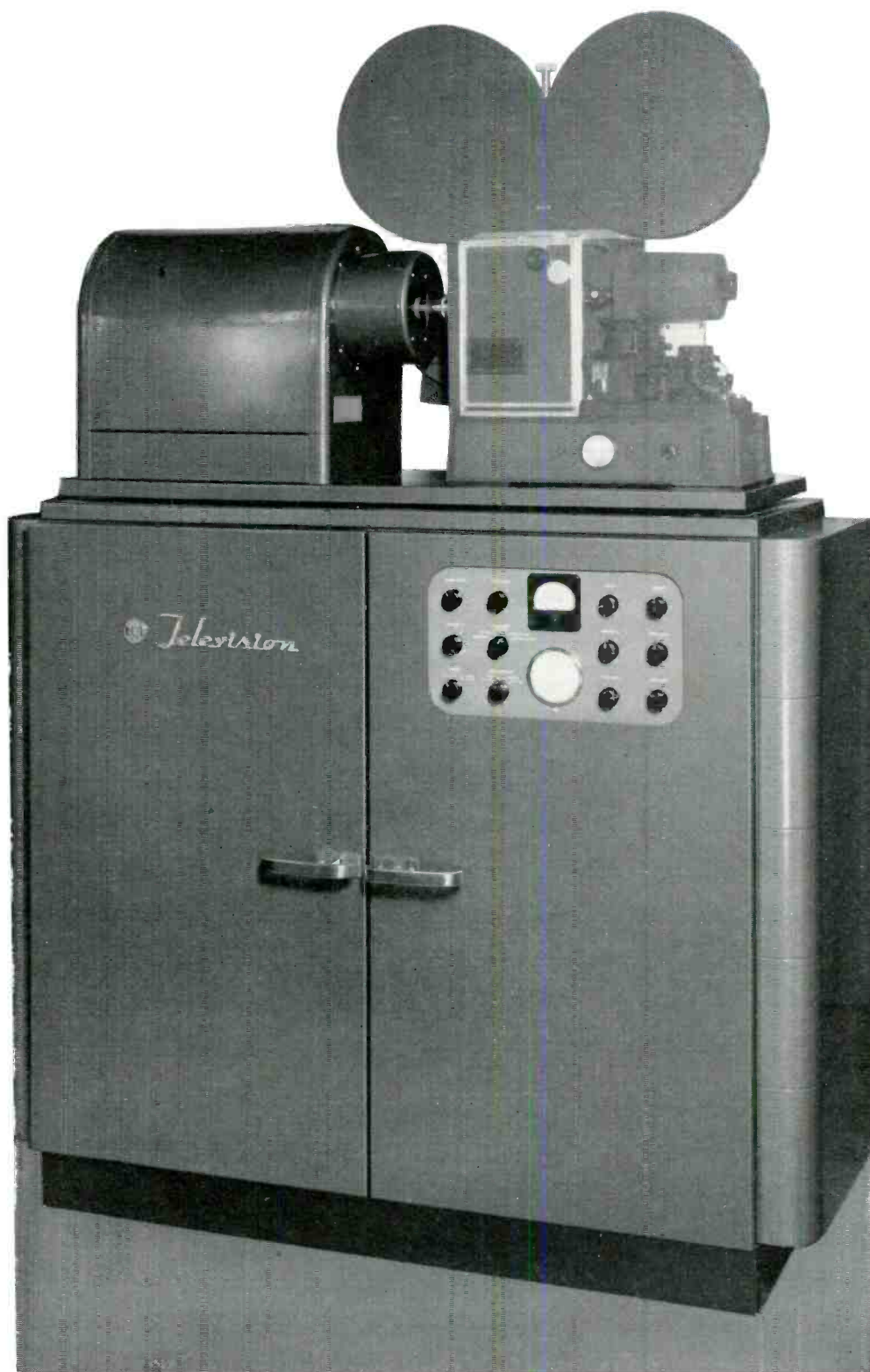
FIG. 2. Overall view of the TMP-20B Kinephoto Equipment which consists basically of a projection type Kinescope associated control panel, deflection circuits and power supplies. Shown in light gray tone are the 16mm motion picture camera TVE-75B and companion Sound Recording Equipment which are available as accessories.
