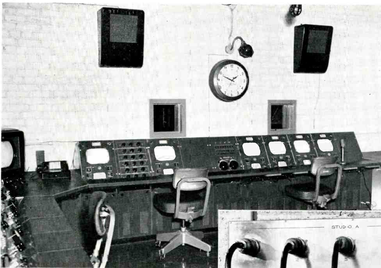
FIG. 28. A special Camera Cable Patching Panel designed by the WOR-TV engineering staff is located in the "Master Control Center."
