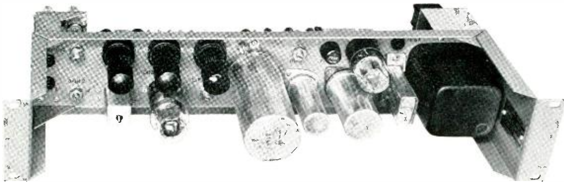
View of the TA-10A Mixing Amplifier chassis which is arranged for standard 19" rack mounting.
