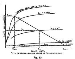
Power output for pentodes as Class A amplifiers can be calculated in much the same way as for triodes by means of the following formulas and a special plate characteristic family of curves, illustrated in Fig. 13.
