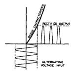
a-c cycle. The 80, 82, 83 and 5Z3 are examples of this type and are called full-wave rectifiers.
