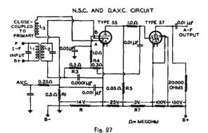
voltage for the 57 a-f amplifier. Under signal conditions, the 55 triode is biased to cut-off. No current flows through load resistor  $R_{\rm B}$  so that the 57 operates at maximum plate current—limited, of course, by the minimum bias supplied by the bleeder  $R_{\rm T}$ . Under this condition, the 57 amplifies the a-f voltage from diode B and passes it on to the audio-requency stages.
