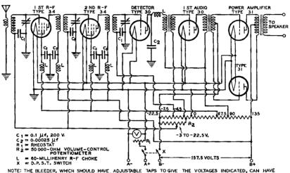
NOTE: THE BLEEDER, WHICH SHOULD HAVE ADJUSTABLE TAPS TO GIVE THE VOLTAGES INDICATED, CAN HAVE A TOTAL RESISTANCE OF 30000 OHMS.
