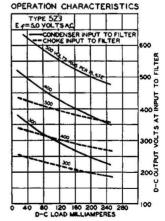
In this service, the plates of each 5Z3 are tied together at the socket. The allowable voltage and load conditions per tube are the same as for full-wave service.
