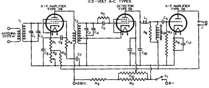
C<sub>1</sub>,C<sub>2</sub>=35 ДДf MIDGET TYPE C<sub>3</sub>C<sub>4</sub>=100 ДДf MIDGET TYPE C<sub>5</sub>,C<sub>6</sub>,C<sub>7</sub>=0.01 Дf MICA TYPE C<sub>8</sub>=0.1 Дf
