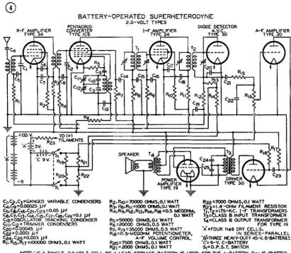
NOTE: IF A SINGLE 2.0-VOLT CELL OF A LEAD STORAGE BATTERY IS USED FOR THE A-BATTERY, R23 IS OMITTED SEE DATA UNDER INSTALLATION ON TYPE 30 FOR ADDITIONAL INFORMATION ON FILAMENT SUPPLIES.
