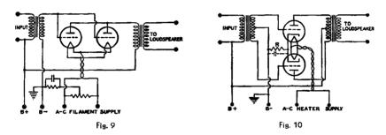
A Class A power amplifier is also used as a driver to supply power to a Class AB or a Class B output stage. Either triodes or pentodes as driver tubes may be used, but triodes are usually preferable since they produce less distortion.
