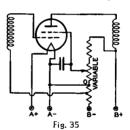
Screen voltage variation for the r-f amplifier stages is sometimes used for volume control of the receiver. Reduced screen voltage lowers the mutual conductance of the tube and results in decreased gain per stage. The voltage variation is obtained by means of a potentiometer shunted across the screen voltage supply. See Fig. 35.
