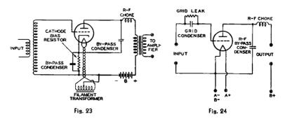
The grid-bias method of detection makes use of a tube which is operated with a grid bias such that the plate current with no signal is practically zero. The bias may be obtained from a cathode resistor (self-bias method), a C battery, or a bleeder circuit. When a signal is applied to the grid, rectification of the carrier occurs in the plate circuit,
