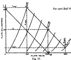
$\text{Per cent 2nd Harmonic Distortion} = \frac{\frac{\text{I max.} + \text{I min.}}{2} - \text{Io}}{\text{I max.} - \text{I min.}} \times 100$
