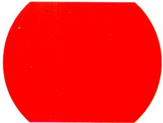
Figure 60 — Raster with Blue and Green Screen Controls CCW, Red Screen Control CW
