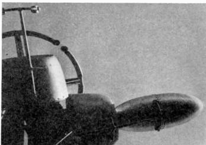
Fig. 17—Position of supporting bracket with respect to collar and ellipsoid. impedance, through a balance converter to a 55-ohm coaxial line, Figure 14.
