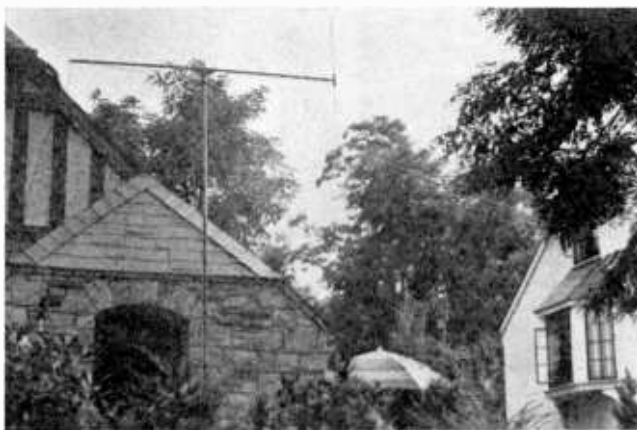
Fig. 8—Receiving antenna on a portable mast, with which data in Fig. 9 were obtained.
