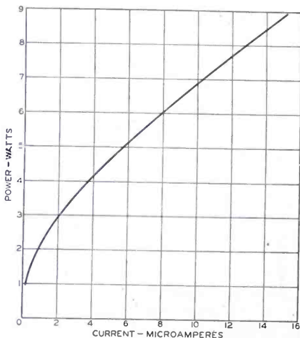
Fig. 6—Low-frequency calibration of an incandescent lamp and phototube used for power measurements.
