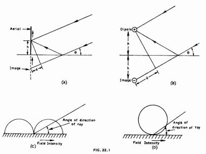
Fig. 22.1. Effects of the earth on the field pattern of a short vertical aerial (A) and of a short horizontal dipole (B). Both (A) and (B) are cross-sectional views, and in (B) the sign + indicates direction of current into the paper while the sign - indicates the opposite direction. Polar diagrams of a short vertical aerial and a short horizontal dipole, both close to earth, are shown in (C) and (D) respectively.
