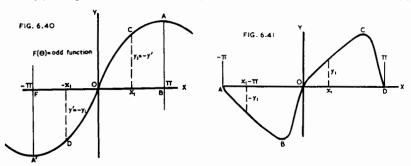
This is the equation for the condition when the fundamental and all the harmonics commence together at zero.
