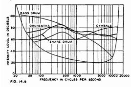
Fig. 14.6. Maximum r.m.s. intensity levels in 1/4 second intervals in critical frequency bands for whole orchestra and certain instruments.
