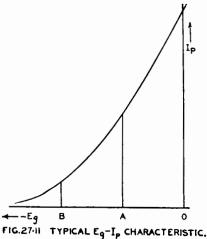
"diode characteristics" but as distinct from the diode, the overload point occurs at quite a low carrier voltage. This method of detection is therefore very much limited in application.
