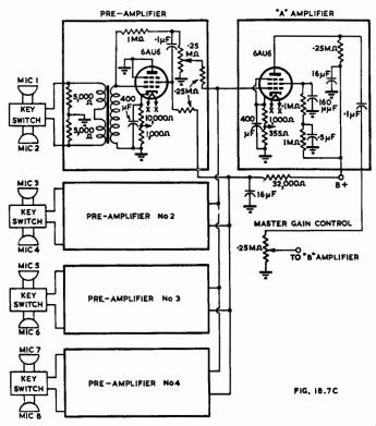
Fig. 18.7C. Essential amplifying and attenuating circuits of pre-amplifiers and "A" amplifier of single unit equipment for studio use (Ref. B18). See also Fig. 18.7D.
