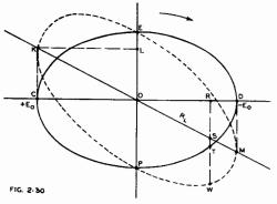
If an elliptical loadline is known, as for example the dashed ellipse of Fig. 2.30, its parallel components may readily be determined. Mark points K and M where the ellipse reaches its maximum and minimum voltage values, then draw the line KM; the slope of KM gives  $R_L$ . Mark O as the centre of the line KM; draw EOP vertically to cut the ellipse at points E and P.
