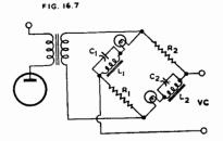
Fig. 16.7. Bridge type of volume expander using lamps which provides bass boosting at low levels.
