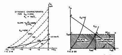
Fig. 2.19. Triode dynamic characteristic (solid line) for resistance loading. Fig. 2.20. Illustrating power dissipation in a resistance-loaded triode.
