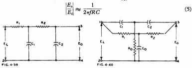
Fig. 4.39 is a two section low pass resistance-capacitance filter.
