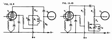
Fig. 15.9. Bass boosting with parallel resonant tuned circuit in plate circuit. Fig. 15.10. Bass boosting with parallel resonant tuned circuit in grid circuit.
