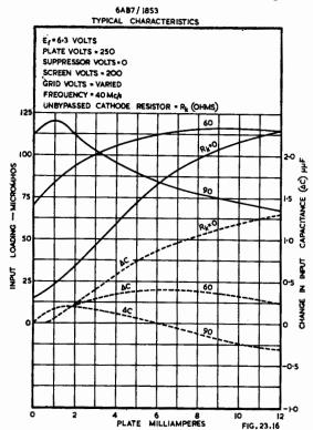
to use in practice. value can be determined by experiment. It will be found that this value, in addition to minimizing capacitance change, also reduces the change in input conductance caused by change in a.v.c. bias. The effect of unbypassed cathode resistance on the change in input capacitance and input conductance of types 6AC7/1852 and 6AB7/1853 is shown in Figs. 23.15 and 23.16. These curves were taken at a frequency of 40 megacycles. The curves for the 6AC7/1852 also hold good for the 1851.
