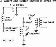
Combined F-M band Fig. 36.3. and A-M short wave band input circuit (Ref. 10).
