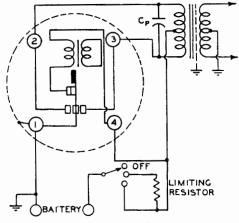
FIG. 32-13 STARTING ARRANGEMENTS FOR 24 AND 32 VOLT VIBRATORS.
