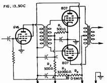
Fig. 13.50C. Class AB<sub>2</sub> amplifier with stabilized bias and screen voltages (Ref. E26).
