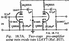
A two-stage pre-amplifier using type 12AY7 twin triode is shown in Fig. 18.7A. This has a total gain of 50 db, and the average noise and hum level referred to the input grid is 11  $\mu$ V (Ref. B17).
