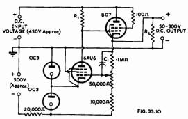
Fig. 33.10. Valve voltage regulator with a controllable output voltage.
