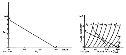
Fig. 2.17. Loadline is independent of valve curves.
