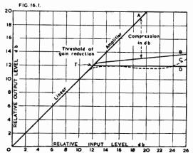
Fig. 16.1. Compression characteristics (B, C, D) of typical peak limiter or volume
