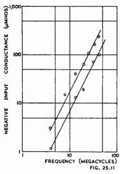
Fig. 25.11. Signal-grid (grid No. 4) conductance of a typical mixer designed for inner-grid injection of oscillator. Lines are drawn with slope of 2. Curve a taken with  $E_{c_1} = 0$ ,  $E_{c_4} = -3$  volts. Curve b taken with  $E_{c_1} = -6$ ,  $E_{c_4} = -6$  volts.
