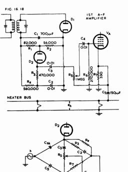
Fig. 16.18. Hum-reduction version of simple series limiter with equivalent circuit to show bridge configuration (Ref. 30).
