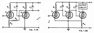
Fig. 7.79. Two-stage uncompensated amplifier with feedback (Ref. H15).
