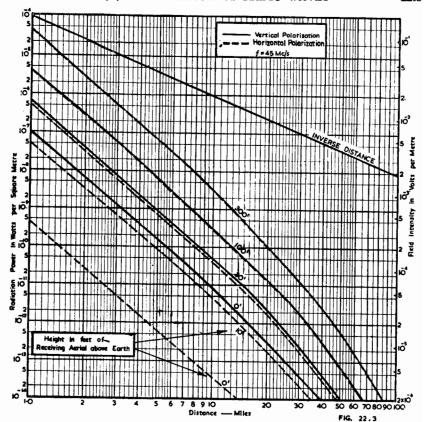
Fig. 22.3. Effect of raising the receiving aerial above the earth (1 KW at 45 Mc/s radiated over earth with conductivity  $\sigma = 10^{-13}$  e.m.u. and transmitting aerial 30 feet above the earth). The same curves also apply when the transmitting and receiving aerials are transposed.
