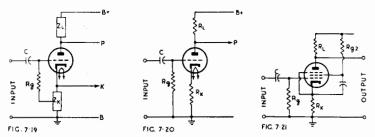
Fig. 7.19. General circuit of a cathode-degenerative amplifier. Fig. 7.20. Resistance coupled amplifier with unbypassed cathode bias resistor, giving cathode degeneration with current feedback.
