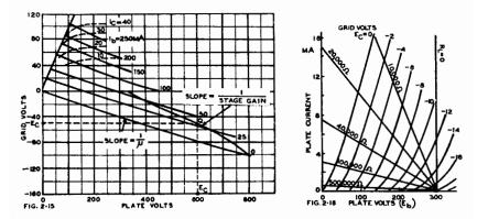
Fig. 2.15. Constant current characteristics for a typical small transmitting triode (801). Fig. 2.16. Triode plate characteristics with loadlines for five values of load resistance.
