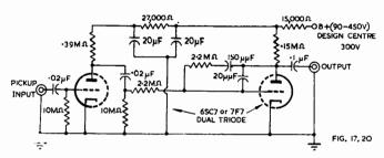
Fig. 17.20. Circuit diagram of equalizing amplifier for low-level electromagnetic packup using negative feedback over the second stage to accomplish equalization (Ref. 144).
