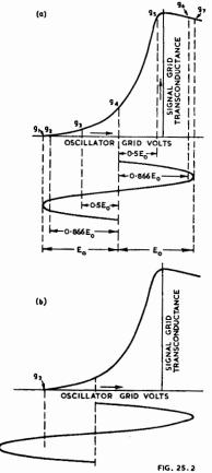
Fig. 25.2a. Points used for 30-degree analysis of conversion transconductance. Fig. 25.2b. Oscillator amplitude and bias adjusted for high conversion transconductance at oscillator fundamental, i.e.,  $g_1 = g_2 = g_3 = 0$ .
