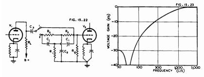
Fig. 15.22. Amplifier providing bass attenuation by Parallel-T network (Ref. 59). Fig. 15.23. Frequency characteristics of amplifier Fig. 15.22 when  $V_1$  = typical r.c.c. pentode,  $C_1$  = 0.001  $\mu$ F,  $C_2$  = 0.004  $\mu$ F,  $C_3$  = 0.02  $\mu$ F,  $R_1$  =  $R_2$  = 2  $M\Omega$ ,  $R_L$  = 0.2  $M\Omega$ ,  $R_v$  = 0.5  $M\Omega$ . The frequency for infinite attenuation is 56 c/s. Switch position (1) Fidelity (2) Bass attenuation (Ref. 59).
