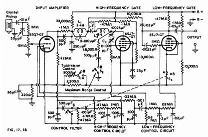
Fig. 17.38. Simple Scott dynamic noise suppressor (Ref. 251 based on Ref. 114).
