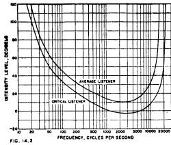
Fig. 14.2. Threshold of audibility curves for average and very critical (5% most acute) listeners in the absence of noise. Reference level 0 db = 0.0002 dyne per sq. cm. Curves by courtesy of Jensen Radio Manufacturing Company, based on Fletcher (Ref. A3).
