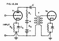
12.24. Circuit diagram of parallel-fed transformer-coupled voltage amplifier.
