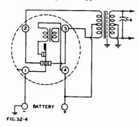
Fig. 32.4. Separate driver system energizing.
