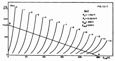
Screen  $I_{c2}$  versus  $E_{c2}$  characteristic for type 6J7;  $E_{bb} = 250$ volts,  $R_L = 0.25 M\Omega$ . A screen loadline is shown.
