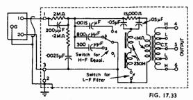
Fig. 17.33. Equalizer for use with Brush high-fidelity crystal pickup (Ref. 106).
