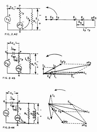
Fig. 2.42. Equivalent circuit and vector diagram of resistance-loaded valve.
