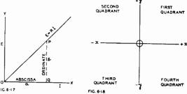
"cause" and "effect," the "cause" (known as the independent variable) is plotted horizontally on the x axis, and the "effect" (known as the dependent variable) vertically on the y axis. In other cases the choice of axes is optional.
