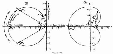
Fig. 7.53. (A) Locus of  $\beta A$  vectors ("Nyquist diagram") for a single stage resistance capacitance coupled triode amplifier with fixed bias (B) Similar locus for a 2 stage amplifier.
