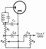
FIG. 27-2 DIODE DETECTOR CIRCUIT
