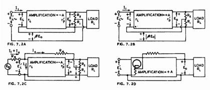
Fig. 7.2. Block diagrams of amplifiers with negative feedback. It is assumed that  $(R_1 + R_2)$  has a resistance very much greater than the load impedance; (A) and (B) have feedback external to the amplifier connected in series with the input voltage (C) has feedback connected in shunt with the input voltage (D) has the feedback connected to a cathode in the amplifier.
