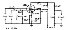
Fig. 18.18A. Fader-mixer circuit using type 6BE6 (Ref. C20).
