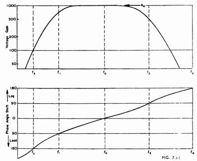
Fig. 7.52. Voltage gain and phase angle shift of an imaginary amplifier. The mid-frequency is f<sub>o</sub> and the maximum voltage gain A<sub>o</sub>.
