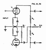
Fig. 12.33. Common plate impedance self-balancing phase inverter.
