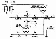
Fig. 16.26. Modified shunt noise limiter (Řef. 30).
