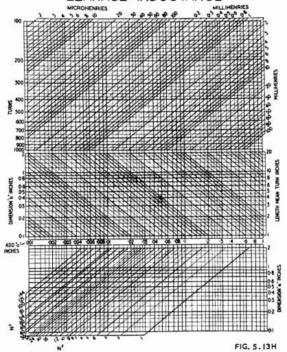
Fig. 5.13H. Leakage inductance chart (Ref. C28).
