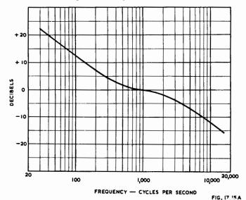
Fig. 17.15A. AES Standard Playback Curve (Ref. 307). See Supplement for new Standard Playback Curve.
