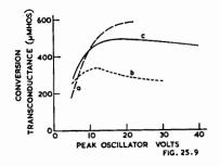
Fig. 25.9. Conversion transconductance of a typical mixer designed for inner-grid injection of oscillator. Signal-grid bias = -3 volts. a, fixed-bias operation of oscillator grid; b, oscillator-grid bias obtained through high-resistance grid leak; c, oscillator-grid bias obtained through a 50,000-ohm grid leak.
