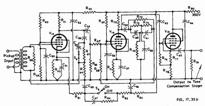
Fig. 17.35B. Williamson pre-amplifier including equalizer and high-pass filter (rumble attenuator). Ref. 270. In the original amplifier  $V_{13}=V_{14}=V_{15}=$  type EF37,  $V_{13}$  and  $V_{14}$  may be replaced by type 6J7 or 1620 if  $R_{71}=1600~\Omega$ .
