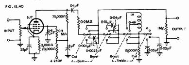
Fig. 15.40. Universal step-type tone control using inductors.
