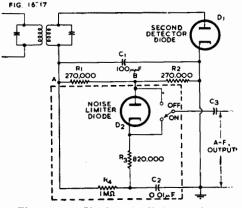
Fig. 16.17. Simple series limiter (Ref. 30).
