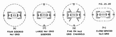
Fig. 25.20. Cross-sectional views of improved mixers designed for outer-grid injection of oscillator. The views show only the portions of the tube inside of and including the oscillator injection grid.
