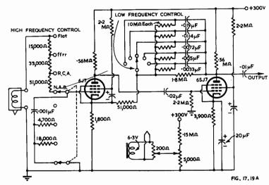
Fig. 17.19A. Circuit diagram of equalizing amplifier using negative feedback to provide bass equalizing (1) 250 c/s (2) 300 c/s (3) 500 c/s (4) 750 c/s (5) 1200 c/s cross-over frequency. A choice of four high-frequency de-emphasis circuits is provided (1) flat (2) ffrr (3) R.C.A. (4) N.A.B. (Ref. 239).
