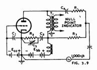
Fig. 3.9. Method of testing for plate resistance.
