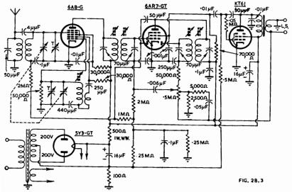
Fig. 28.3. Reflex superhet, receiver with screen reflexing (Ref. 4).
