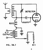
Fig. 34.1. Self quenched superregenerative receiver incorporating linear reflex detector.
