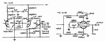
Fig. 15.48. Two-stage bass and treble tone control (Ref. 41).
