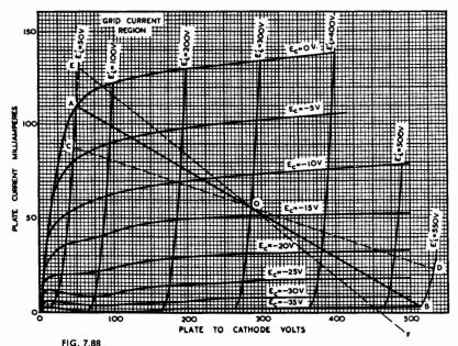
Fig. 7.88. Cathode follower characteristics of beam power tetrode and typical of all pentodes. Loadline AOB is normal; CD high resistance; EF low resistance illustrating grid current and plate current cut-off.
