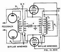
Fig. 13.50D. Basic principles of McIntosh Amplifier (Ref. E28).
