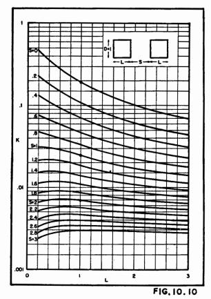
Fig. 10.10. Chart giving coefficient of coupling for a specified spacing between two coaxial solenoids having identical dimensions. The quantities S and L are measured in terms of coil diameters. (Ref. 56.)
