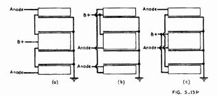
Fig. 5.13P. Arrangements for push-pull output transformer (Ref. C29).
