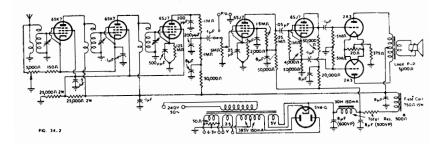
Fig. 34.2. Typical t.r.f. receiver
