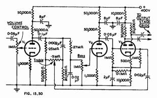
Fig. 15.50. Wide-range two-channel amplifier (Ref. 31).
