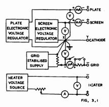
Fig. 3.1. Basic circuit for testing electrode currents.
