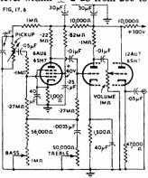
Fig. 17.6. Pre-amplifier for use with strain-sensitive pickup (Ref. 336)
