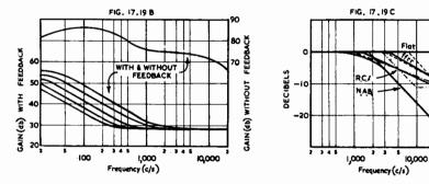
Fig. 17.19B. Frequency characteristics of circuit of Fig. 17.19A with high frequency control in "flat" position (Ref. 239).
