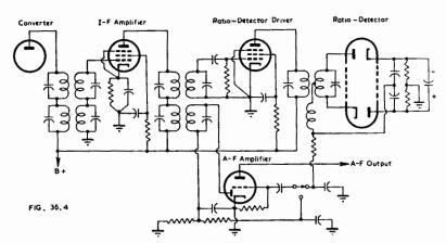
Fig. 36.4. Combined F-M A-M i-f channel using one A-M i-f amplifier and two F-M i-f amplifiers.
