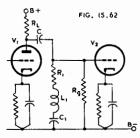
Fig. 15.62. Whistle filter using resonant circuit.
