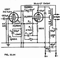
Fig. 15.64. Amplifier providing synthetic bass (Ref. 73).
