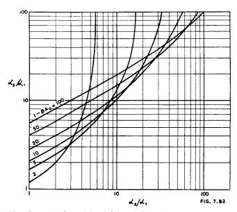
Fig. 7.82. Curves for determining  $\alpha_2$  for critical damping of two-stage compensated amplifier (Ref. H15).
