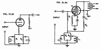
Fig. 15.53. Bass and treble boosting due to negative feedback incorporating L and C in cathode circuit (Ref. 26).
