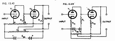
Direct-coupled amplifier with only one source of voltage (E, b). Fig. 12.42. Fig. 12.43. Direct-coupled amplifier with one source of voltage and one voltage divider.
