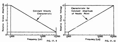
Fig. 17.9. Constant velocity recording characteristics showing relative variation of groove amplitude with frequency.
