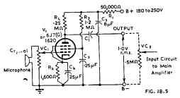
Fig. 18.5. Single stage pentode pre-amplifier for use with diaphragm-type crystal microphone.
