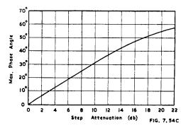
Fig. 7.54C. Maximum phase shift as a function of attenuation in the circuit of Fig. 7.59A (Ref. H18).
