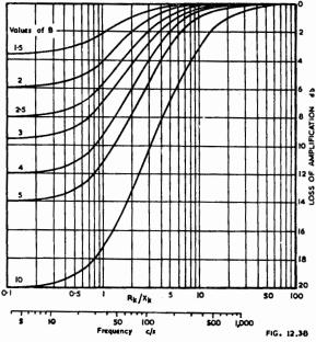
Fig. 12.3B. Universal attenuation curves with cathode bias (Ref. A11 Part 4).
