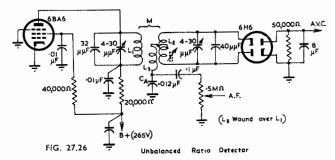
De-emphasis is obtained in the circuit of Fig. 27.26 by adjusting the value of the capacitor marked  $C_A$ . The time constant (0.4 second) of the diode load circuit is about twice as long as that previously recommended for typical cases, but the performance is quite good, and, as suggested in Ref. 37, the individual designer can set the constants to suit his own requirements.
