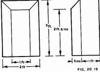
20.19. Loudspeaker enclosure to minimize diffraction effects (after Ref. 193).
