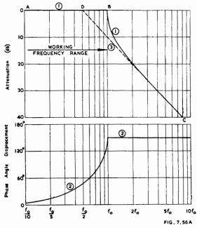
Fig. 7.56A. Bode's method—Curve (1) attentuation characteristic and (2) phase angle displacement characteristic for constant 150° phase angle displacement above upper working frequency  $f_o$ ; curve (3) constant slope 10 db/octave (Ref. H11).
