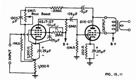
Fig. 15.11. Two stage amplifier with negative feedback over both stages providing bass-boost tone control (typical application).
