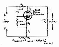
Fig. 31.7. Practical valve hum neutralizing circuit.
