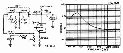
Fig. 15.15. Single stage amplifier incorporating a parallel-T network in the feedback loop (Ref. 57).
