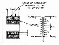
Fig. 5.12. Transformer wound with balanced secondaries.
