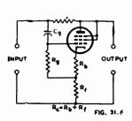
Fig. 31.6. Valve hum neutralizing circuit.
