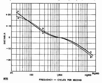
Fig. 17.15D. (A) Old AES Standard Playback Gurve; (B) New RIAA—AES—NARTB—RCA New Orthophonic Standard Playback Curve (RT14).
