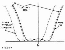
With any other type of coupling which has no mutual inductance component, one of the two humps remains at the intermediate frequency. The mistuning is then half the frequency bandwidth between humps.
