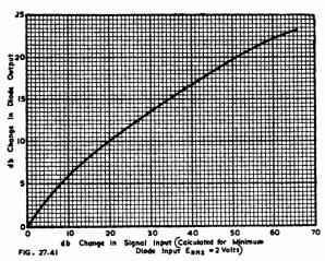
Fig. 27.41. Calculated a.v.c. characteristic for a single controlled stage using type 6SK7.
