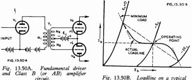
Loadline on a typical Fig. 13.50B. triode driver.
