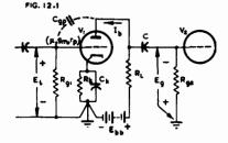
Fig. 12.1. Triode valve (V<sub>1</sub>) resistancecapacitance coupled to V<sub>2</sub>.
