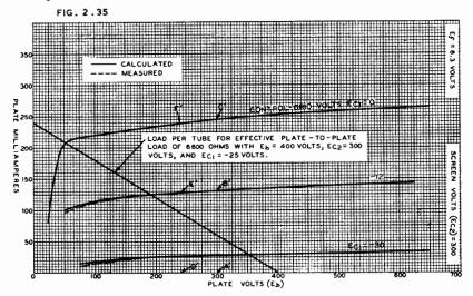
Fig. 2.35. Derived plate characteristics for type 807 with different screen voltage, making use of Figs. 2.33 and 2.34 with conversion factors (Ref. E2).
