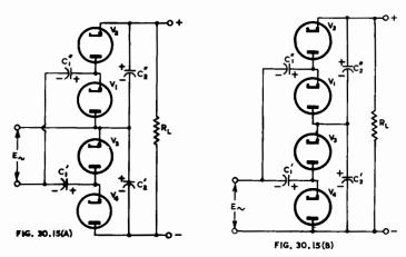
Figs. 30.15(A) and (B). Voltage quadrupler rectifier circuits.
