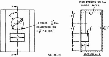
Fig. 20.13. Typical corner cabinet with vented baffle, designed for a Goodmans Axiom 12 inch loudspeaker with a bass resonant frequency of 55 c/s, which can be used with a speaker resonant at 75 c/s by removing the tunnel. Cubic capacity about 8000 cu. ins. = 4.6 cu. ft. (Ref. 182).
