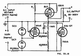
Fig. 33.13. Valve voltage regulator with a controllable output voltage as Fig. 33.10 but including constant current pentode to draw constant bleed current for varying output voltages.
