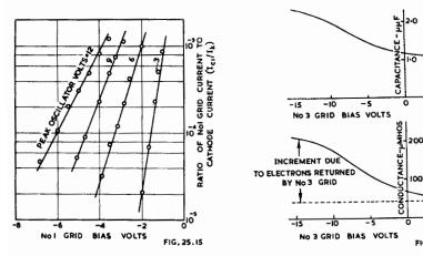
Fig. 25.15. Signal-grid (grid No. 1) current in a typical mixer with a 20-megacycle oscillator voltage applied to grid No. 3.  $E_{c_3} = -10$  volts,  $E_{c_2} = 100$  volts,  $E_b = 250$  volts,
