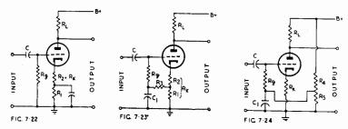
Fig. 7.22. Cathode degenerative amplifier with a small degree of current feedback. Cathode degenerative amplifier with a large degree of current feedback. Cathode degenerative amplifier with an alternative method of obtaining grid bias.
