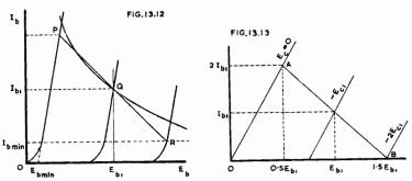
Plate characteristics of imaginary triode with "ideal" characteristics Fig. 13.12. above I b min and curved characteristics below this line. Fig. 13.13. Ideal triode characteristics with  $R_L = 2r_p$ .
