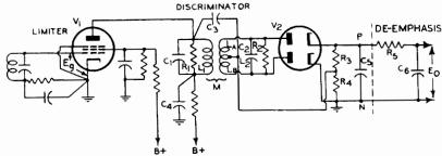
TYPICAL PHASE DISCRIMINATOR ARRANGEMENT FOR F-M DETECTION. FIG 27:17
