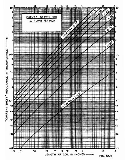
Fig. 10.4. Curves for the determination of Current Sheet Inductance (L<sub>s</sub>) for small solenoids, plotted against length of coil (l). For other pitches refer to Fig. 10.5.
