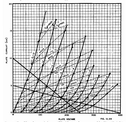
Fig. 13.9B. Plate characteristics type 6J5 with g m and g, curves and loadlines (Ref. B5).
