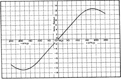
FIG. 27.18(B) Discriminator Characteristic Obtained From Design Example
