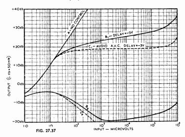
enough a.v.c. bias voltage to the a-f amplifier to give the required overall results. The improvement in the overall a.v.c. characteristics, when audio a.v.c. is used, can be seen from Figs. 27.36 and 27.37.
