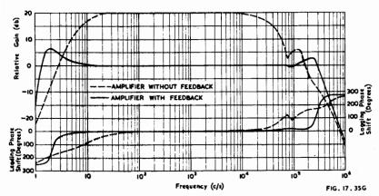
Fig. 17.35G. Loop gain and phase-shift characteristics of Williamson main amplifier (Ref. 270);
