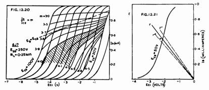
Fig. 12.20. Plate dynamic characteristics for type 6J7 with curves of constant plate to screen current ratio. The shaded area has m within  $\pm$  5%. Fig. 12.21. Cathode loadline (OF) with single plate dynamic characteristic for type 6J7. The broken lines show the limits of  $\pm$  10% tolerances in  $R_k$ .
