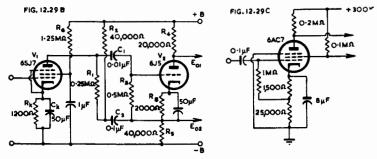
Fig. 12.29B. Phase splitter  $(V_2)$  using high input impedance to increase the gain of the preceding stage  $(V_1)$  by about six times.
