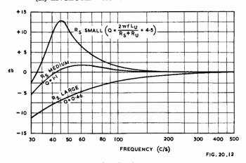
Fig. 20.12. Theoretical response of enclosed cabinet loudspeaker for various values of the effective damping resistance R<sub>s</sub>. Resonance frequency 45 c/s. (Ref. 135). References to enclosed cabinets: 13A, 29, 36, 80, 81, 84, 116, 116A, 135, 147, 151, 166, 168, 188.
