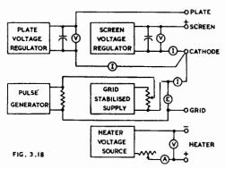
Fig. 3.18. Circuit for measuring electrode currents using single pulse generator method  $(I=peak-reading\ current\ indicator,\ E=peak-reading\ voltage\ indicator,\ V=moving\ coil\ voltmeter)$ . If high accuracy is required, correction should be made for the voltage drop across the current indicators. The regulation of the electrode supplies is not important for point by point testing, provided that the shunt capacitors are sufficiently large.
