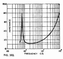
Fig. 20.2. Impedance versus frequency characteristic of a typical popular loudspeaker.
