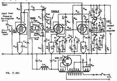
Fig. 17.35C. Williamson tone compensation and filter unit (Ref. 270). In the original amplifier  $V_0 = V_{10} = V_{11} =$  type EF37. All may be replaced by type 9002, or by type 6AU6 with a slight increase in gain, or by type 6J7 (or 6J5 triode) with a slight decrease in gain.
