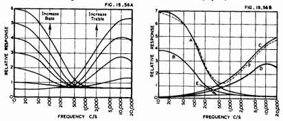
Fig. 15.56A. Response characteristics of Patchett tone control circuit with S<sub>1</sub> open and S<sub>2</sub> closed, and other control at minimum (Ref. 9).
