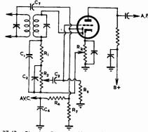
FIG. 27.42 Biased Detector Muting System
