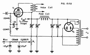
Fig. 13.52. Circuit of portion of a receiver using back bias.  $V_1$  is the power amplifier,  $V_2$  is the rectifier.
