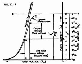
Dynamic characteristic of r.c.c. pentode for fixed screen voltage (b) compared with mutual characteristic (a).
