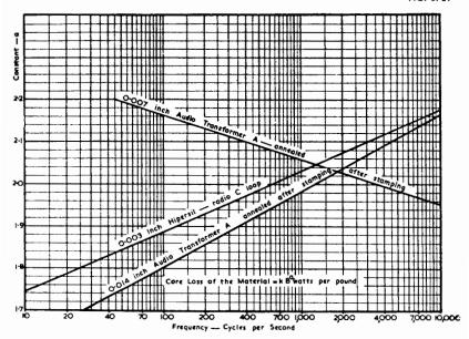
Fig. 5.21. Experimentally determined curve showing values of "a" as a function of frequency for several magnetic materials (Ref. E2).
