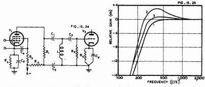
Fig. 15.24. Amplifier providing bass attenuation by constant k filter (Ref. 60). Fig. 15.25. Frequency characteristics of amplifier Fig. 15.24 when  $V_1=$  typical r.c.c. pentode,  $C_1=C_2=0.002~\mu F\pm 5\%$ ,  $C_3=1~\mu F$ , L=70~H with Q=6; Curve (1)  $R_1=R_2=0.25~M\Omega$ ; Curve (2)  $R_1=50~000~\Omega$ ,  $R_2=0.5~M\Omega$  (unbalanced); Curve (3) as Curve 2 with additional resistance in inductor to give Q=3~(Ref.~60).
