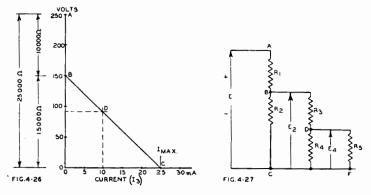
Graphical method for determining the output voltage from a potential Fig. 4.26. divider.
