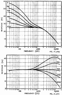
channel. Outputs from the three channels are added in a single valve feedback summing amplifier; potentiometers which add flat loss in the auxiliary channels permit control of the resultant transmission characteristic. The input allows for the connection of two G.E. variable reluctance pick-ups simultaneously. The maximum output is of the order of 1 volt, and the pre-amplifier may be used at a moderately remote location, owing to the cathode follower output.
