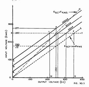
Fig. 30.3. Constant current curves for a 5Y3-GT rectifier; condenser-input filter with capitance 8µF and effective plate supply impedance 80 ohms per plate.
