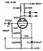
Fig. 12.35. Modified "see-saw" self-balancing phase inverter (Ref. C10). Fig. 12.36. Practical "Schmitt" common cathode impedance self-balancing inverter using type 6C8-G twin triode ( $\mu=36$ ).  $C_1$  and  $C_2$  should have high insulation resistance.
