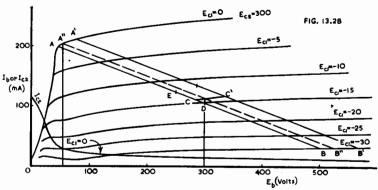
Plate characteristics of 6L6 or 807 illustrating method of correcting the Fig. 13.28. loadline for rectification. The corrected loadline is A" B".
