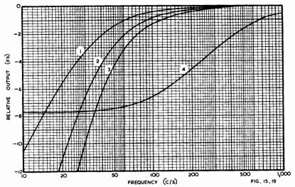
Fig. 15.19. Bass attenuation versus frequency characteristics: (1) Single grid coupling condenser (R=1 megohm,  $C=0.005~\mu F$ ); (2) Two stages each with identical values of time constant RC; (3) Three stages each with identical values of time constant; (4) R.c.c. pentode with by-passed cathode resistor (6]7,  $R_L=0.25~M\Omega$ ,  $R_k=2000~\Omega$ ,  $C_k=0.5~\mu F$ ) and screen adequately by-passed.
