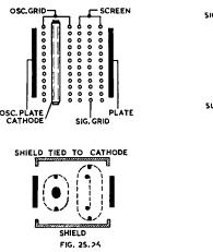
Fig. 25.26. Electrode arrangement of the triodehexode type 6K8(G).
