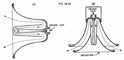
Fig. 20.22. Concentric folded horns (A) three section reflex (B) three section reflex radial type,
