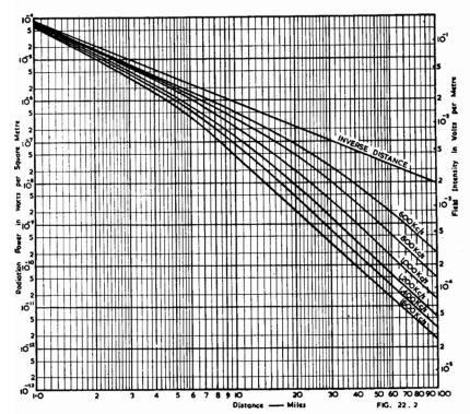
Attenuation at medium frequencies of the radiation from a transmitter (1 KW radiated, short aerial, average earth conductivity,  $\sigma = 7 \times 10^{-14}$  e.m.u.,  $\epsilon = 15$ ).
