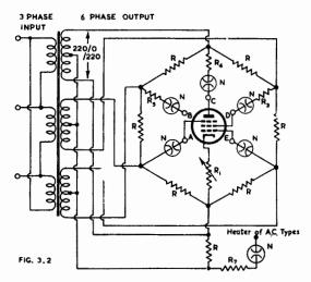
Fig. 3.2. Hexaphase shorts and continuity tester. Suitable values are R=5000 ohms,  $R_3=R_5=7500$  ohms,  $R_4=1500$  ohms,  $R_7=5000$  ohms,  $R_1=5000$  ohms for battery values other than power output, 33 000 ohms for normal a.c. types, or 15 000 ohms for power output values. Lamps (N) are 110 volt  $\frac{1}{2}$  watt split-anode neon.
