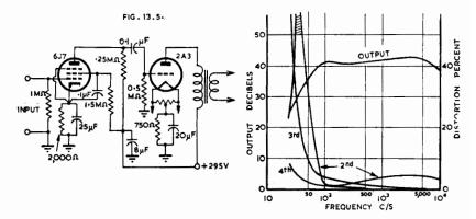
Fig. 13.54. Harmonic distortion of amplifier having type 6J7 pentode coupled to 2A3 triode loaded by a loudspeaker on a flat baffle. The distortion was measured by a wave analyser connected across the voice coil. The bass resonance frequency is 70 c/s.
