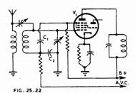
Fig. 25.22. Screen regeneration in converter stage.
