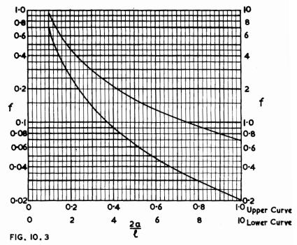
Fig. 10.3. Variation of f with  $(2 \ a/l)$ . Curves derived from U.S. Dept. of Commerce Circular' C74 "Radio instruments and measurements".
