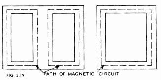
Fig. 5.19. Magnetic cores, showing method for calculation of length of magnetic path.
