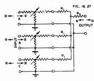
Fig. 18.27. Constant impedance mixer using three T type attenuators in parallel.
