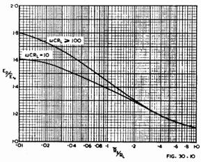
Fig. 30.10. Ratio of operating peak inverse voltage to peak applied a.c. for rectifiers used in condenser input filter circuits.
