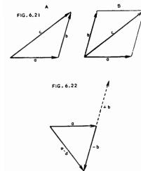
beginning of the first one to the end of the last one. Fig. 6.21A shows two vectors, a and b, which are added together to give the resultant c. Exactly the same result is obtained by placing a and b together, as in Fig. 6.21B, completing the parallelogram, and taking c as the diagonal. Vectors are generally printed in bold face type, to distinguish them from scalar values, which have no direction, although they have magnitude and sign (i.e. positive or negative).
