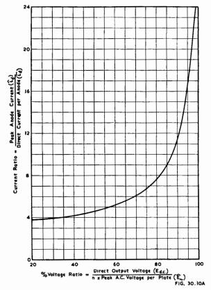
This curve is for full-wave, half-wave and voltage-doubler rectifiers with condenser-input filters. It applies for any size of condenser so long as the condenser is large enough to give maximum output voltage for the given output current and r.m.s. voltage input. For half-wave and voltage-doubler rectifiers the direct current per anode  $\vec{l}_d = I_L$ ; for full wave rectifiers  $\vec{l}_d = \frac{1}{2}I_L$ . n = 1 for full-wave and half-wave rectifiers.
