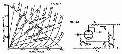
Fig. 12.4. Plate characteristics of high-mu triode (6SQT) with  $E_{bb}=400$  volts and  $R_L=0.5$  megohm. Cathode bias loadlines for selected values of cathode bias resistance  $(R_k)$  have been drawn in.
