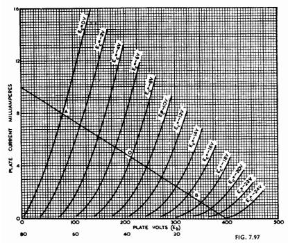
Method of calculating performance of cathode degenerative triode without drawing special characteristics.
