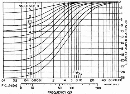
Fig. 12.11A. Curves for the frequency response of a resistance-coupled pentode with screen dropping resistor  $R_s$  and screen by-pass reactance  $X_s$  (=  $1/\omega C_s$ ). The value of B is given by eqn. (1a). The frequency for  $R_s/X_s = 1$  is given by  $f = 1/2\pi R_s C_s$ . The frequency scale should be traced and the tracing moved horizontally until f corresponds to  $R_s/X_s = 1$  (method after Sturley).
