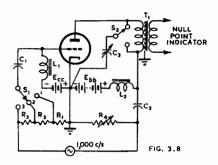
Fig. 3.8. Bridge test for measuring amplification factor.
