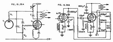
Fig. 15.35A. Amplifier with variable treble attenuation due to negative feedback. Fig. 15.35B. Amplifier with negative feedback providing treble attenuation or treble boosting (Ref. 67).
