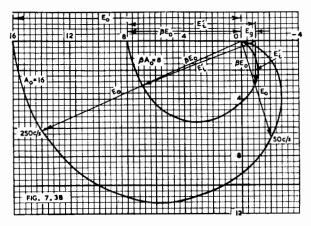
Fig. 7.38. Construction to demonstrate correction of phase shift by negative feedback.
