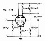
Fig. 12.46. Direct-coupled amplifier incorporating twin triode with relative positions opposite to those in Fig. 12.45 (extracted from Ref. D19).
