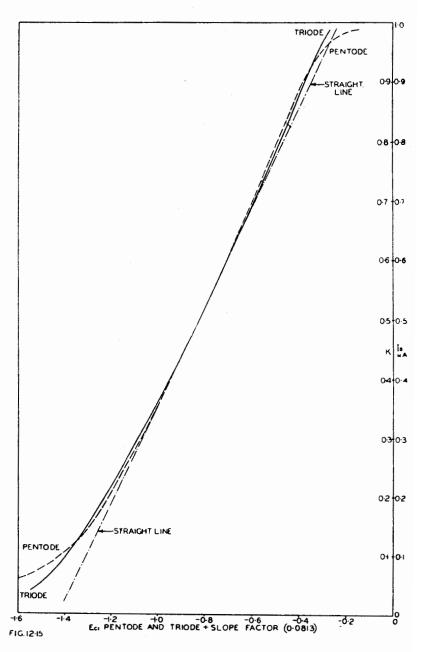
Fig. 12.15. Comparison between pentode and triode dynamic characteristics of the same valve (6SJ7 with  $E_{bb}=250$  volts,  $R_L=0.25$  megohm,  $E_{c2}=22.5$  volts for pentode,  $E_{c2}$  connected to plate for triode characteristics; triode characteristics divided by slope factor 0.0813 and superimposed so that points for  $I_b=0.5$  mA coincide).
