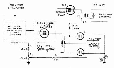
Fig. 16.27. Degenerative noise limiter, acting between first and second i-f stages (Ref. 30).
