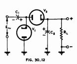
Fig. 30.12. Half wave voltage doubler rectifier circuit.
