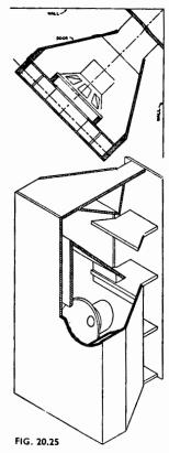
Fig. 20.25. Top and isometric view of the Klipsch bass reproducer Model K-3. (Ref. 48).
