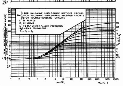
Fig. 30.8 (above). Ratio of r.m.s. diode current to average diode current for one anode, expressed as a function of  $\omega CR_L$ ; (below) Ratio of peak diode current to average diode current for one anode, expressed as a function of  $\omega CR_L$  (Ref. 6).
