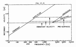
Fig. 17.13. Ideal recording characteristics.
