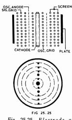
Fig. 25.25. Electrode arrangement of the pentagrid type 6A8(G).
