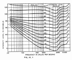
Fig. 19.7. Contours of equal loudness level (0 db = 10<sup>-16</sup> watt/cm<sup>2</sup>)—Ref. 28, after Fletcher and Munson (Ref. 40).
