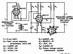
Fig. 33.14. Voltage regulator utilizing a special voltage reference tube (type 5651) to give extremely good voltage regulation.
