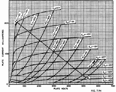
Fig. 7.94. Feedback characteristics of beam power tetrode (6L6 or 807 with  $E_{c2}=300~V)$  and 10% voltage feedback ( $\beta=-0.1$ ).
