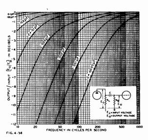
Fig. 4.36. Attenuation in decibels versus frequency for a resistance-capacitance coupling or filter (Fig. 4.35A) in which the total resistance (R) = 1 megohm. If applied to a resistance-coupled valve amplifier,  $R = R_\sigma + r_\rho R_L/(r_\rho + R_L)$ . If  $r_\rho$  is less than 10 000 ohms, the error in neglecting the second term is less than 1%. If the valve is a pentode, R may be taken as  $(R_\sigma + R_L)$  with a sufficient accuracy
