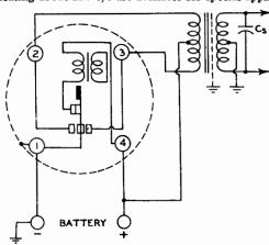
FIG.32-1 INTERRUPTER TYPE VIBRATOR.
