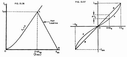
Fig. 13.36. Method of deriving the approximate power output and load resistance of a Class  $AB_1$  amplifier from the characteristics of a single valve. The method may also be used with poorer accuracy for Class  $A_1$ .
