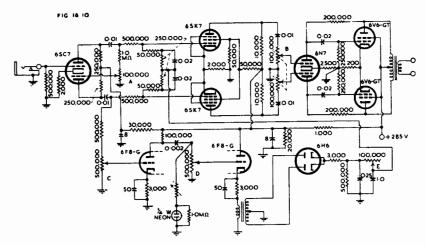
Fig. 16.10. Volume expander incorporating remote cut-off pentodes (Ref. 23). Controls A = balance, B = volume, C = input level, D = expansion, E = time constant.
