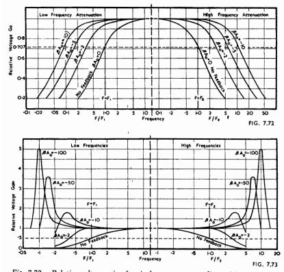
Fig. 7.72. Relative voltage gain of a single stage r.c.c. amplifier without feedback and with three selected values of feedback (Ref. H4).
