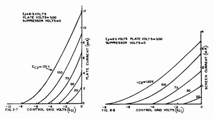
Fig. 2.7. Mutual characteristics of a pentode, with constant plate voltage, and five fixed screen voltages.
