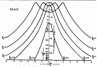
Selectivity Curves for Two Identical Coupled Circuits,
