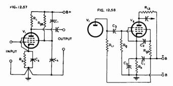
Fig. 12.57. Hum neutralization in a r.c.c. pentode.
