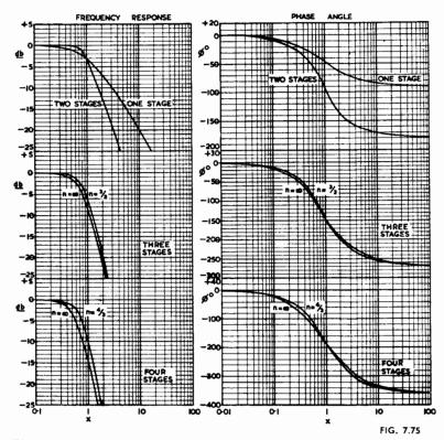
Fig. 7.75. Frequency response and phase angle of frequency response for 1,2,3, and 4 r.c.c. stages designed for maximum flat response by Mayr's method (Ref. H13).
