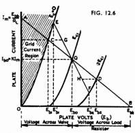
Fig. 12.6. Plate characteristics of r.c.c. triode with normal loadline AB, operating point Q, and working loadline EQF due to grid resistor shunting.
