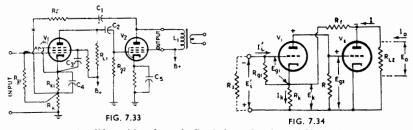
Fig. 7.33. Amplifier with voltage feedback from the plate of  $V_2$  to the cathode of V<sub>1</sub>, also incidentally incorporating negative current feedback due to the unbypassed resistor  $R_k$ . Fig. 7.34. Simplified a.c. equivalent of Fig. 7.33 for calculations.
