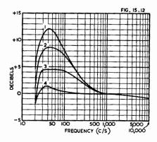
Fig. 15.12. Frequency characteristics of amplifier in Fig. 15.11. Condition (1) tone control max. resistance (2) three quarters max. (3) half max. (4) one quarter max. resistance. The curves have been superimposed to coincide at 1000 c/s.
