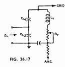
Fig. 26.17. Alternative load circuit for crystal filter stage.
