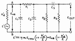
FIG. 27-8 EQUIVALENT DIODE CIRCUIT AT AUDIO FREQUENCIES.
