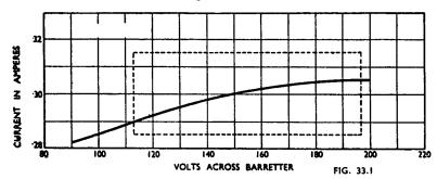
Fig. 33.1. The characteristic of a typical barretter.
