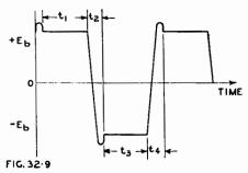
As the effect of overclosure is to produce high transient voltages, and as during life the tendency is for  $t_1$  and  $t_3$  to become shorter, the vibrator will rapidly deteriorate. By aiming at slight under-closure the effect during life is for conditions to approach 100% closure.
