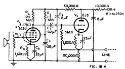
This circuit has the disadvantage that the cathode follower stage may give rise to audible hum. It should therefore be restricted to use with a sensitive type of crystal microphone or to applications where a low hum level is not essential.
