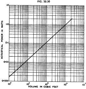
Fig. 20.30. Acoustical power required to produce an intensity level of 80 db as a function of the volume of the auditorium for optimum reverberation times (after Olson, Ref. 13, by kind permission of the author and of the publishers and copyright holders, Messrs. D. Van Nostrand Company Inc.).
