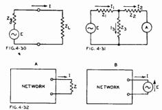
Fig. 4.32. (A) An impedance Z in a network with current I and voltage drop ZI (B) Equivalent circuit having identical results so far as current and voltage drop are concerned, with a generator developing a voltage E=ZI. This illustrates the Compensation Theorem.
