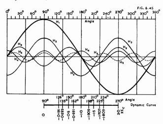
fourth, and higher order even harmonics reach their maximum values (either positive or negative) at  $0^{\circ}$ ,  $90^{\circ}$ ,  $180^{\circ}$ ,  $270^{\circ}$  and  $360^{\circ}$  on the fundamental scale.
