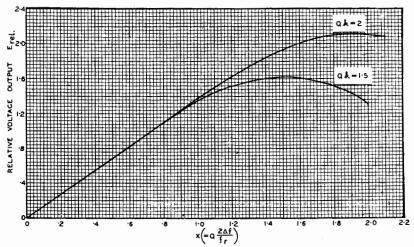
FIG. 27:18(A) GENERALISED PHASE DISCRIMINATOR CURVES OF RELATIVE VOLTAGE OUTPUT  $(\mathsf{E}_{\mathsf{rel.}})$  VERSUS X WITH E2/4-2; Q4-15 AND 2.
