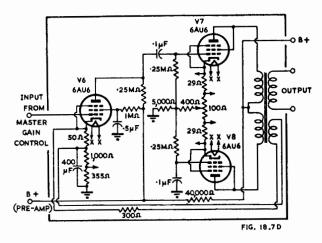
Fig. 18.7D. "B" amplifier of same equipment as Fig. 18.7C (Ref. B18).
