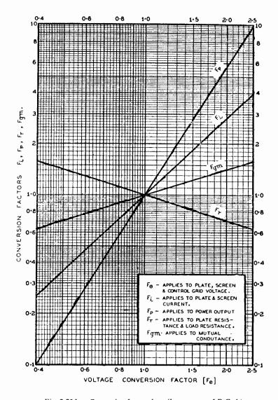
Fig. 2,32A. Conversion factor chart (by courtesy of R.C.A.).
