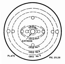
Fig. 25.29. Electrode arrangement of pentagrid type 6BE6.
