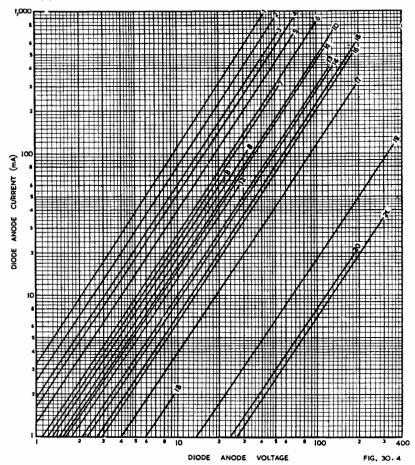
Fig. 30.4. Average anode characteristics of some rectifier valves (based on Ref. 6, with additions). The value of  $r_d$  for any rectifier at any diode current may be determined by dividing the diode anode voltage by the diode current.
