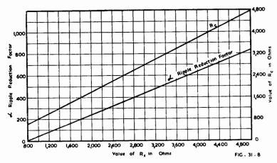
Fig. 31.8. Values of  $\alpha$  and R as a function of R, for the circuit of Fig. 31.7.
