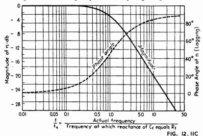
Fig. 12.11C. Magnitude and phase of factor for use in Fig. 12.11D (Ref. A12). Reprinted by permission from RADIO ENGINEERS' HANDBOOK by F. E. Terman, copyrighted in 1943, McGraw-Hill Book Company Inc.
