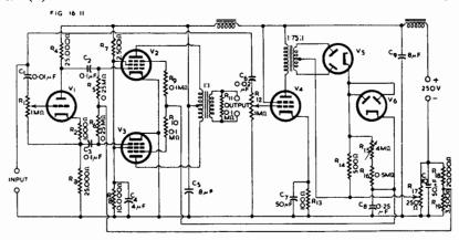
Fig. 16.11. Volume expander incorporating push-pull suppressor-controlled pentodes (Ref. 7).  $V_1 = MH_4$ ,  $V_2 = V_3 = AC/SP1$ ,  $V_4 = KT41$ ,  $V_5 = V_6 = AZ3$ .
