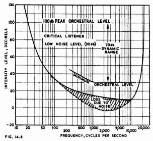
Fig. 14.8. Effective hearing characteristic for very critical listener with low room noise level, showing 70 db dynamic range for orchestra in a concert hall. Minimum orchestral level based on Ref. E13.
