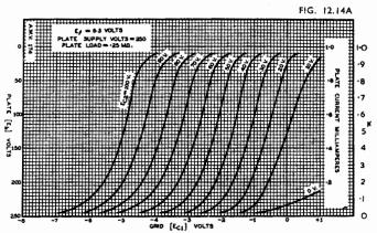
Fig. 12.14A. Family of dynamic characteristics for typical r.c.c. pentode (type 6]7 with  $E_{bb} = 250$  volts,  $R_L = 0.25$  megohm).
