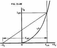
Fig. 13.49. Typical grid mutual characteristic illustrating Class B operating conditions.
