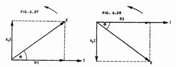
A similar procedure applies with a capacitance instead of an inductance (Fig. 6.28) except that the capacitive reactance is  $X_c$  instead of  $X_L$  and the vector of peak voltage drop across  $C(\mathbf{X}_c\mathbf{I})$  is drawn vertically downwards, since it must be opposite to  $\mathbf{X}_L\mathbf{I}$ . The current (I) here leads the voltage (E) by the angle  $\theta$ .
