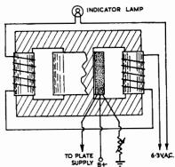
FIG. 27.50 Saturated Reactor Tuning Indicator
