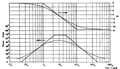
Fig. 7.54B. Attenuation and phase characteristics of "step circuit" Fig. 7.59A for particular case with step attenuation 20db (Ref. H18).
