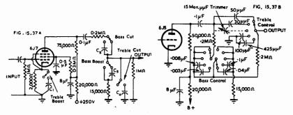
Fig. 15.37A. Simple universal tone Fig. 15.37B. Step-type tone control control not using inductors. not using inductors (Ref. 70).
