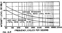
The masking teffect of room noise is shown by Fig. 14.3 for average and for very quiet residences. These curves may be applied directly to the hearing characteristics of Fig. 14.2. The result is shown in Fig. 14.4 for average conditions and in Fig. 14.5
