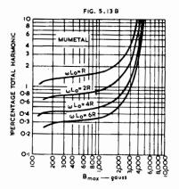
5.13B. Total harmonic Fig. distortion plotted against flux density for different ratios of primary reactance to R where R = plate resistance + primary resistance (Ref. C9).
