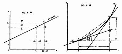
As with the simpler case of the straight line, take a second point (Q) with its x coordinate increased by  $\Delta x$ . Also, as before, call the increment in the y coordinate  $\Delta y$ . It will therefore be seen that, commencing at point P, an increment ( $\Delta x = PC$ ) in the value of x results in an increment  $(\Delta y = CQ)$  in the value of y.
