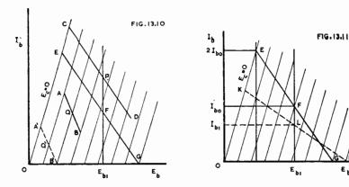
"Ideal" plate characteristics of triode to illustrate choice of optimum Fig. 13.10. loadline.
