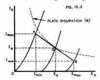
Fig. 13.2. Loadline applied to triode plate characteristics to determine power output and distortion.
