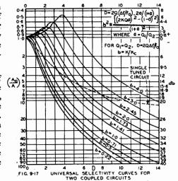
Band width is:  $f_o \sqrt{k^2 - k_c^2} \approx 8.6 \text{ Kc/s}$ . Ratio of gain in valley to that at peak is:
