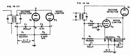
Fig. 16.23. Balancing-type noise limiter Fig. 16.24. Triode shunt-type noise (Ref. 30). limiter (Ref. 30).
