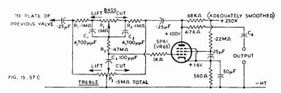
Fig. 15.57C. Tone control circuit. Tolerances  $R_1$ ,  $R_2$ ,  $C_1$ ,  $C_2$ ,  $R_3$ ,  $C_3 \pm 5\%$ , and  $P_2$  are linear potentiometers,  $P_2$  having a fixed tapping at 50% rotation. source impedance should not be more than 10,000 ohms.  $C_4$  should normally be  $0.05\mu F$ if following stage has 0.25 M \Omega grid leak (Ref. 91). Type 6AU6 could be used as substitute for the type shown, with suitable values of cathode and screen resistors, to give an output of about 2 V r.m.s.
