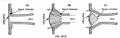
Fig. 20.21. Different forms of sound chambers in horn loudspeakers.
