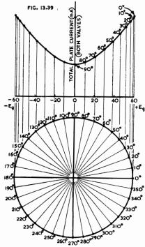
Fig. 13.39. Plate current (both valves) with 10° angular increments.
