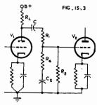
Fig. 15.3. Conventional bass boosting circuit (plate shunt compensation).
