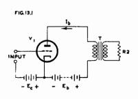
Fig. 13.1. Basic circuit of a Class  $A_1$ triode with transformer-coupled load.
