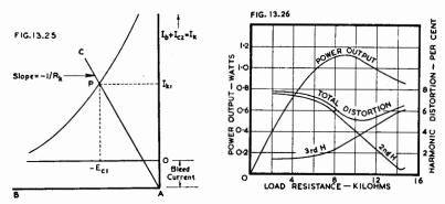
Fig. 13.25. Cathode loadline of pentode with additional bleed current passing through the cathode resistor, plotted on mutual characteristics. Fig. 13.26. Power output and harmonic distortion of typical pentode plotted against load resistance. Valve type 6AK6,  $E_b = E_{c2} = 180 V$ ,  $E_{c1} = -9$ , peak signal = 9 volts.
