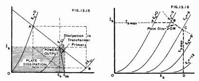
Fig. 13.15. Power output and dissipation relationships in a Class A triode. Fig. 13.16. Plate characteristics of small battery operated power triode with limits of maximum plate dissipation, maximum plate voltage and maximum plate current.
