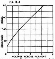
Resistance characteristic Fig. 16.4. of typical 4-6 volt 0.04 A metal filament lamp used in volume expanders (Ref. 45).
