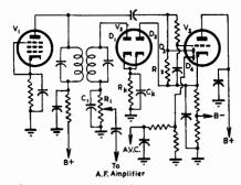
FIG. 27.43 Biased Detector Muting System with D.C. Amplified a Deloyed A.V.C.
