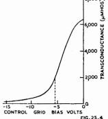
Fig. 25.4. Transconductance characteristic of a typical variableμ, radio-frequency pentode.
