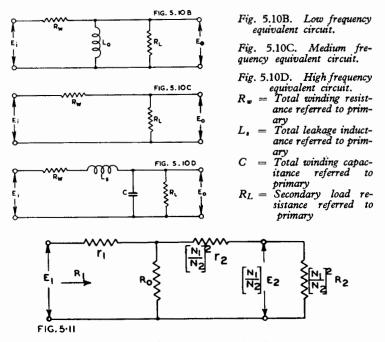
Fig. 5.11. Simplified equivalent circuit referred to the primary.
