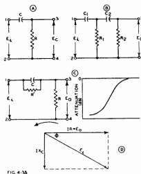
Fig. 4.35. (A) is a resistance capacitance high-pass filter; (B) is a two section filter; (C) is a modified form of A, providing attenuation within top and bottom limits; (D) is the vector diagram of A.
