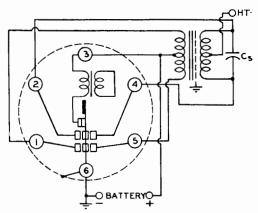
FIG. 32.2 SELF-RECTIFYING TYPE VIBRATOR.
