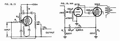
Fig. 15.13. Single stage amplifier giving bass boosting with adjustable frequency characteristic (Ref. 36).
