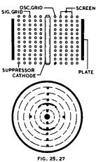
Fig. 25.27. Electrode arrangement of the pentagrid type 6SA7(GT).
