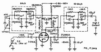
Circuit of pre-amplifier and filter circuit with high attenuation at 10 000 Fig. 17.24B. c/s (Ref. 113).
