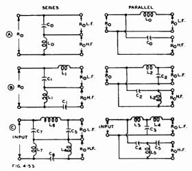
Fig. 4.53. Frequency dividing networks (A) 6db (B) 12db (C) 18db for the octave beyond the cross-over frequency, L.F. indicates low frequency, H.F. indicates high frequency speakers.
