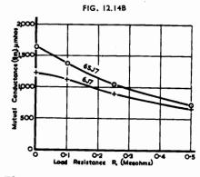
Fig. 12.14B. Mutual conductance of resistance-capacitance coupled pentodes types 6]7 and 6SJ7 plotted against load resistance. In each case the value of K is taken as being adjusted to give maximum mutual conductance.
