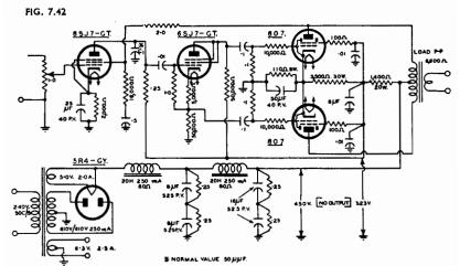
Fig. 7.42. 30 watt push-pull amplifier with voltage feedback from one output plate to the screen of the first stage. Stability is ensured by adjustment of condenser  $C_1$ .
