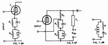
Fig. 7.66. One form of subsidiary feedback (after Ref. A7). Fig. 7.67. Another form of subsidiary feedback (after Ref. A7). Fig. 7.68. Two terminal network as cathode load impedance.
