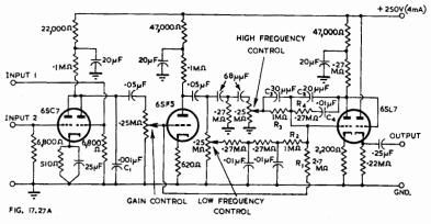
RESPONSE Fig. 17.27. (A) Circuit of continuously variable equalizing pre-amplifier (B) Variation in attenuation in low frequency control (C) Variation in attenuation in high frequency con-
