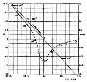
Summation of two attenuation characteristics having slopes of zero Fig. 7.64. and 11 db/octave.
