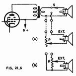
may be neglected provided that R is not less than five times the voice-coil impedance. At low levels this arrangement has a high impedance but here again the effect will not be serious.
