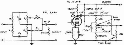
Fig. 15.44A. Simple duo-control circuit giving individual control of bass and treble. Typical values are:  $R_1 = 0.25 \ M\Omega$ ;  $R_2 = R_3 = 0.5 \ M\Omega$ ;  $R_4 = 0.25 \ M\Omega$ ;  $R_5 = R_6 = 0.5 \ M\Omega$ ;  $C_1 = 0.01 \ \mu F$ ;  $C_2 = 0.001 \ \mu F$  (Ref. 22). Fig. 15.44B. Simple tone control giving bass and treble boosting (Ref. 41).
