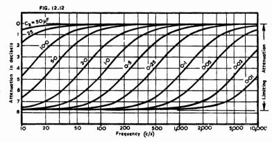
Fig. 12.12. Attenuation characteristics for selected values of cathode by-pass condenser with valve type 6J7 and  $E_{bb} = 250$  volts,  $R_L = 0.25$ ,  $R_g = 0.5$ ,  $R_s = 1.5$  megohms,  $R_k = 2000$  ohms: screen adequately by-passed.
