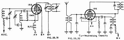
Fig. 25.31. Self-excited 1R5 converter circuit.
