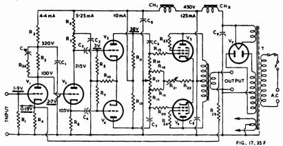
Fig. 17.35F. Williamson main amplifier—new version (Ref. 270). Voltages underlined are peak signal voltages at 15 watts output.
