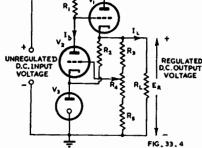
Referring again to Fig. 33.4. If constant output voltage is to be maintained across the load, the valve  $V_1$  must be capable of adjusting its voltage drop to compensate for voltage input changes. A similar condition exists if the input voltage is constant and variable output voltage is required. The valve has therefore to satisfy conditions at four points as set out in Table 2.
