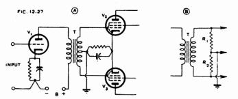
Fig. 12.27. (A) Triode valve  $(V_1)$  followed by transformer (T) having centre-tapped secondary and exciting the grids of the push-pull stage  $(V_2, V_3)$ . (B) Modified form with non-centre-tapped transformer, using two resistors to provide an equivalent centre-tap.
