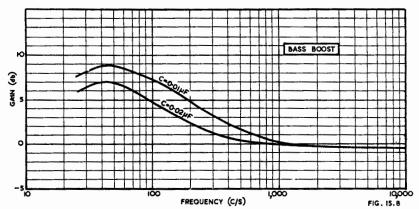
Fig. 15.8. Frequency characteristics with the circuit of Fig. 15.7,  $V_1=6$ J7,  $R_L=0.05~M\Omega$ ,  $R_1=0.2~M\Omega$ ,  $R_k=2000~\Omega$ ,  $C_k=25~\mu F$ ,  $R_s=1.5~M\Omega$ ,  $C_s=0.1~\mu F$ ,  $C=0.02~\mu F$ ,  $R_v=1~M\Omega$ .
