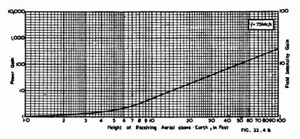
Fig. 22.4 (A) Attenuation at 75 Mc/s of the radiation from a transmitter (1 KW radiated over earth with  $\sigma=10^{-13}$  e.m.u.,  $\epsilon=5$ , with receiving aerial at zero height); (B) Multiplying factor for height of receiving aerial above earth.
