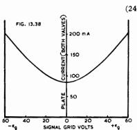
Fig. 13.38. Plate current (both valves) plotted as a function of the signal grid voltage.
