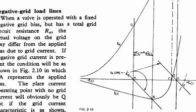
Fig. 2.10. Grid current characteristics with grid loadlines.
