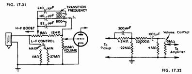
Fig. 17.31. Flexible equalizer for high-fidelity crystal pickups (Ref. 127). Fig. 17.32. Equalizer for Acos GP12 high fidelity crystal pickup, for 250 c/s cross-over frequency (Ref. 120).
