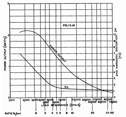
Fig. 13.14. Power cutput and distortion of type 45 triode plotted against load resistance. The curves were derived graphically, with allowance for shifting loadline. The operating conditions are:  $E_b = 250$  volts,  $F_c = -50$  volts, peak grid signal voltage 50 volts,  $I_b = 34$  mA (zero signal),  $r_p = 1610$  ohms.
