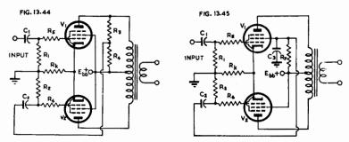
Fig. 13.44. Push-pull circuit using phase inversion in the power stage. Fig. 13.45. Push-pull circuit using screen resistance coupling from  $V_1$  to the grid of  $V_2$ .
