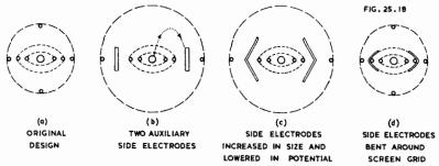
Fig. 25.18. Cross-sectional views of mixer designed for outer-grid-injection of oscillator. The views show only the portions of the tube inside of and including the oscillator injection grid.
