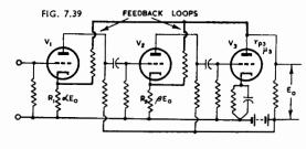
Fig. 7.39. Amplifier with interconnected positive and negative feedback loops in which the negative loop is completely contained within the positive.
