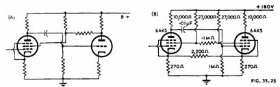
Positive feedback circuits for eliminating screen bypass capacitors Fig. 35.25. (Ref. 51).
