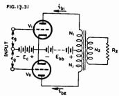
Fig. 13.31. Fundamental circuit of push-pull power amplifier.
