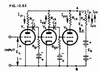
Fig. 12.52. Three stage amplifier demonstrating the effects of impedance  $(R_4)$  in the power supply.
