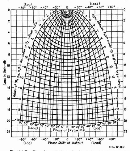
Fig. 12.11D. Curves from which the loss in gain and phase shift of output at low frequencies resulting from resistance-condenser bias impedance R<sub>i</sub>C<sub>i</sub>, can be calculated in a resistance-coupled amplifier for the general case where both screen and bias impedances are of importance (Ref. A12). Reprinted by permission from RADIO ENGINEERS' HANDBOOK by F. E. Terman, copyrighted in 1943, McGraw-Hill Book Company Inc.
