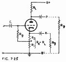
Fig. 7.25. Conventional phase splitter.
