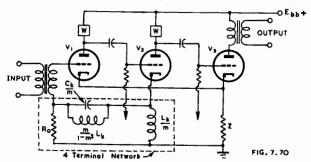
Fig. 7.70. Three stage amplifier incorporating subsidiary feedback in the form of a 4 terminal network. m = 0.87. W = "Wheeler" network (based on Ref. A29).
