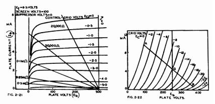
Fig. 2.21. Loadlines of resistance-loaded pentode.
