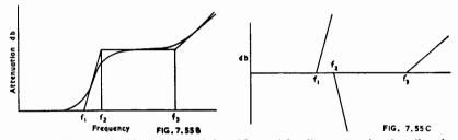
Fig. 7.55B. Attenuation characteristic with straight line approximation (based on Bode, Ref. H11).
