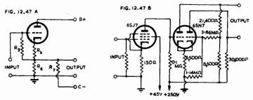
Fig. 12.47A. Cathode follower used as d.c. amplifier (Ref. D15), Fig. 12.47B. Direct-coupled amplifier with r-c pentode exciting phase inverter (Ref. D14).
