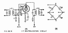
value required. The neutralization is generally not sufficiently critical to require different capacitance values in different receivers of the same type, as even partial neutralization is helpful and often sufficient.
