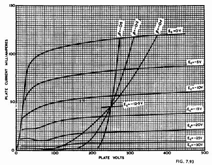
Fig. 7.93. Single input voltage curve for each of three values of voltage feedback for beam power tetrode (6V6-GT with  $E_{\rm c2}=250$  V), to illustrate effect of feedback.
