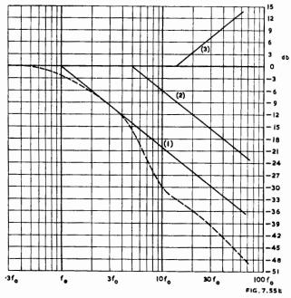
Fig. 7.55E. Typical attentuation characteristic of amplifier with feedback (broken curve) and component "semi-infinite" slopes (1, 2 and 3) from which Fig. 7.55A is constructed (Ref. H18).
