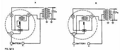
Fig. 32.5. Two alternative methods of shunt coil energizing; (A) with separate starting contacts (B) conventional shunt energizing.
