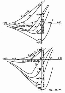
Fig. 25.10. Signal grid (grid No. 4) admittance of a typical mixer designed for innergrid injection of oscillator at 31.5 megacycles. Curves taken with no oscillator voltage applied. Data represents electronic admittance only (i.e. "cold" values were subtracted from measured values before plotting.)
