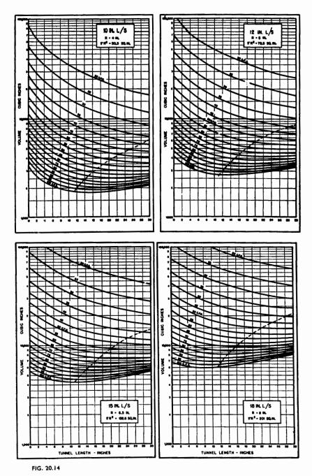
Fig. 20.14. Curves showing tunnel length for 10, 12, 15 and 18 inch Goodmans loudspeakers with bass resonant frequencies from 20 to 100 c/s. The tunnel length should not exceed 1/12 of the wavelength of the speaker bass resonant frequency; points to the right of the broken lines should not be used (Ref. 182).
