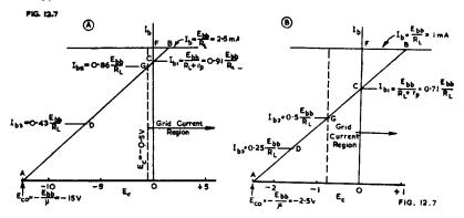
Fig. 12.7. "Ideal" linear dynamic characteristics (A) for general purpose triode with  $\mu=20$ ,  $r_p=10\,000$  ohms,  $R_L=0.1$  megohm and  $E_{bb}=250$  volts; (B) for high-mu triode with  $\mu=100$ ,  $r_p=0.1$  megohm,  $R_L=0.25$  megohm and  $E_{bb}=250$  volts.
