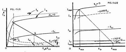
Fig. 13.21. Plate, screen and cathode current characteristics of pentode.
