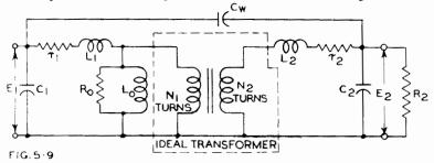
Fig. 5.9. Equivalent circuit of a practical transformer.
