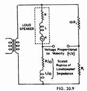
Fig. 20.9. Bridge circuit to give a voltage proportional to the velocity of the cone, to be fed back to the input. (Ref. 184).
