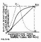
Fig. 5.15. BH characteristics of a typical transformer steel. The dashed curve is the permeability  $\mu$  where  $\mu = B/H$ .
