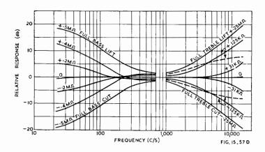
Fig. 15.57D. Measured frequency response curves of circuit of Fig. 15.57C. on curves are resistance values between potentiometer slider amd centre of element. Dotted curves are with  $P_2$  centre-tap disconnected from earth and with one 0.33  $M\Omega$  resistor connected from each end of  $P_2$  to earth (Ref. 91).
