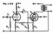
This circuit (Fig. 7.51B) may also be used with any desired degree of feedback. The effective plate resistance of  $V_2$  may be increased or decreased by the positive feedback as shown by the following analysis and Fig. 7.51C. Here  $R_1$  replaces  $R_7$  and  $R_8$  in parallel, no input signal is applied but a signal generator E is inserted in the plate circuit. It is assumed that  $R_4$  is very much greater than  $R_3$ . We thus obtain
