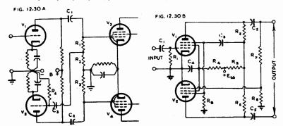
Fig. 12.30A. Conventional form of phase inverter in which  $V_1$  excites  $V_3$ , and  $V_2$  excites  $V_4$ , the grid of  $V_2$  being connected to a tapping on the grid resistor of  $V_3$ . Fig. 12.30B. Phase inverter with pentodes using the suppressor grids for self-balancing (Ref. C19).
