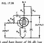
A modification of the circuit of Fig. 17.28 is described in Ref. 280 which gives both bass boosting (with a "very low frequency roll-off") and high frequency de-emphasis. Values of components are:  $R_1=0.33$  megohm,  $R_2=1.0$  megohm,  $R_L=0.22$  megohm,  $C=600~\mu\mu\mathrm{F}$  approx. (adjustable),  $C_2=25~\mu\mu\mathrm{F}$  approx. (adjustable) shunted across  $R_2$ , and  $V_1 = EF37$ .
