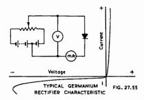
There is little change in rectifier characteristics from 15°C to 50°C, but above this temperature up to 100°C, both forward and back slope resistances decrease slowly.
