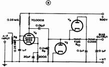
Fig. 16.9. Volume expander using negative feedback; (A) amplifier (B) circuit for supplying control bias to the amplifier (Refs. 22, 24).  $V_1 = V_2 = V_3 = V_4 = SP41$ ;  $V_6$  and  $V_6$  together = 6H6.
