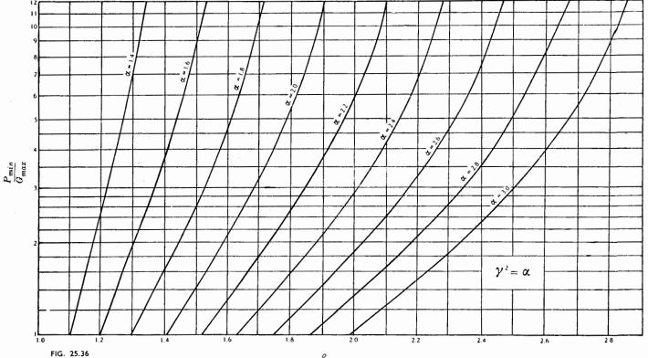
Fig. 25.36. Charts giving high values of  $P_{min}$  for geometrical-mean tracking.
