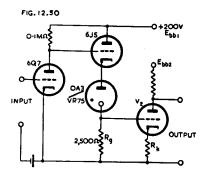
Fig. 12.50. Improved two stage amplifier with gas tube coupling, in which o cathode follower is introduced for better performance.
