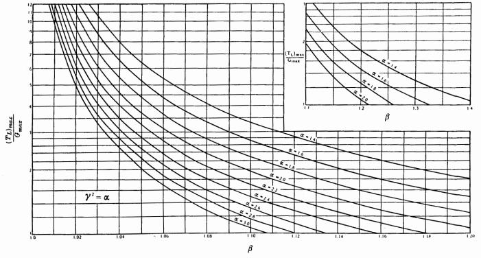
FIG. 25.38 Fig. 25.38. Chart giving high values of  $T_{L_{max}}$  for geometrical-mean tracking.
