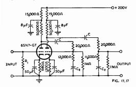
Fig. 17.17. Circuit diagram of two stage bass equalizing amplifier with bass boosting in each stage. Pin 4 of the 6SN7-GT should be used for the input circuit. Total boost is 20 db and max. slope 6 db/octave. C = 0.25 μF for good bass response or 0.1 μF for some bass attenuation;  $C_2 = 0.1 μF$  for cross-over 250 c/s or 0.05 μF for 500 c/s. Voltage gain at 1000 c/s = 22 times = 26.8 dbvg.
