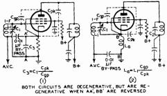
FIG. 26-20 METHODS FOR STABILISING R-F AND I-F AMPLIFIERS
