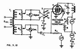
Fig. 3.12. Phase reversal method of measuring conversion transconductance.
