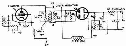
FIG. 27-19 ALTERNATIVE ARRANGEMENT FOR PHASE DISCRIMINATOR.
