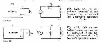
The current in any impedance,  $Z_I$ , connected to two terminals of a network consisting of any number of impedances and generators (or voltage sources) is the same as though  $Z_L$  were connected to a simple generator, whose generated voltage is the open-circuited voltage at the terminals in question, and whose impedance is the impedance of the network looking back from the terminals, with all generators replaced by impedances equal to the internal impedances of these generators.
