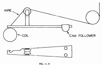
Fig. 11.4. Type of finger recommended for universal winding.
