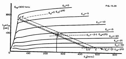
Fig. 13.29. Plate characteristics of 6L6 or 807 giving graphical method for deriving the effect of internal resistance in the voltage supply source.
