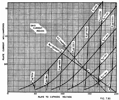
Fig. 7.85. Cathode follower characteristics of small general purpose triode. The solid loadline is for  $R_k = 15\,000$  ohms, the dashed loadline is for the addition of an a.c. shunt load.
