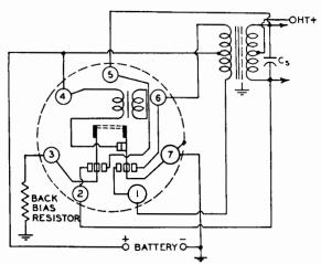
FIG. 32-3 SPLIT-REED SELF-RECTIFYING TYPE VIBRATOR.
