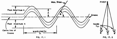
Fig. 17.1. Unmodulated (left) and modulated (right) groove of lateral recording. Fig. 17.2. Motion of stylus tip with lateral recording.
