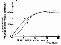
Fig. 25.14. Conversion transconductance of a typical mixer designed for outer-grid injection of oscillator. Signalgrid bias,  $E_{c_1} = -3$  volts. Curve a corresponds to fixed No. 3 grid bias,  $E_{c_3} = -8$  volts. Curve b corresponds to bias obtained through a 50 000-ohm grid leak.
