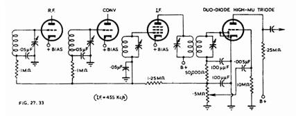
The circuit values shown are typical for an intermediate frequency of 455 Kc/s. An a.v.c. resistor of 1.25 megohms is used so that the total resistance to earth from any grid does not exceed 2 megohms. If there were only two controlled stages this could be increased to about 1.75 megohms with a consequent decrease in the a.c. shunting.
