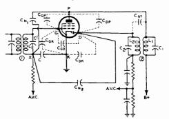
FIG. 26-21 NEUTRALIZATION IN DIODE PENTODE
