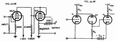
Fig. 12.48. Two stage amplifier with the plate of the first stage directly-coupled to the screen of the second stage (Ref. D14).
