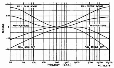
Fig. 15.57B. Response characteristics of Fig. 15.57A (Ref. 77).
