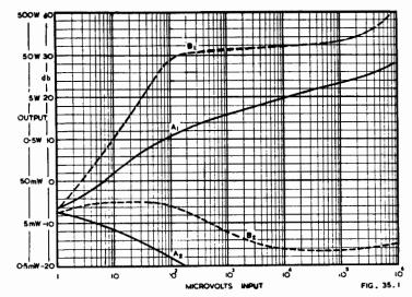
Fig. 35.1. A.V.C. and noise characteristics.
