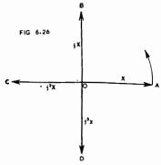
reversal of direction which is the same as a change of sign. The operator  $j^2$  is therefore equivalent to multiplication by -1.
