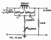
Fig. 15.62A. Narrow-band rejection filter (Ref. 81).
