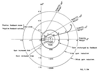
Fig. 7.54. Additional information furnished by a "Nyquist diagram" (see also Fig. 7.53 A and B.)
