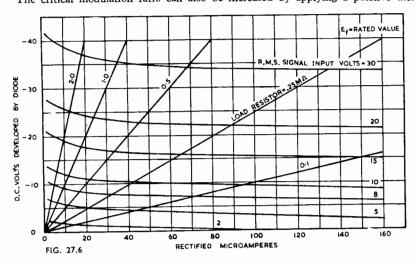
bias voltage to the diode plate. This arrangement is only satisfactory if the bias can be changed for each i-f input voltage  $(E_{\tau ms})$  see Ref. 1 (page 348).
