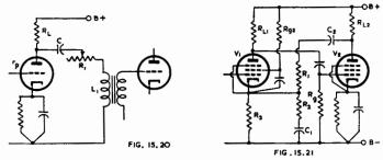
Fig. 15.20. Amplifier, giving variable low-frequency cut-off using a-f transformer and parallel feed.
