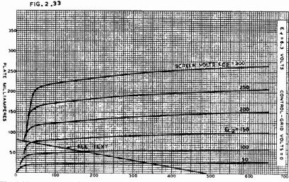
Fig. 2.33. Zero bias plate characteristics for type 807 beam power amplifier with six values of screen voltage (Ref. E2).
