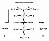
Fig. 18.16. Multiple T section attenuator.
