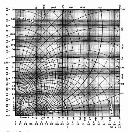
Fig. 4.21F. Chart for conversion between resistance and reactance, and conductance and susceptance  $Z = (R \pm jX) \cdot 10^n, \quad Y = (G \mp jB) \cdot 10^{-n}.$
