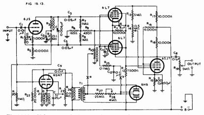
Fig. 16.13. Volume expander incorporating push-pull 6L7 control valves (Ref. 21).
