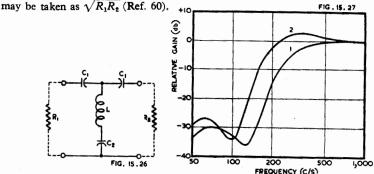
Fig. 15.26. One T section of a series M-derived filter. Fig. 15.27. Frequency characteristics of filter Fig. 15.26; Curve (1)  $R_1=R_2=0.25~M\Omega$ ,  $C_1=0.0023~\mu F$ ,  $C_2=0.024~\mu F$ , L=74~H; Curve (2)  $R_1=50~000~\Omega$ ,  $R_2=0.5~M\Omega$  (unbalanced),  $C_1=0.0058~\mu F$ ,  $C_2=0.035~\mu F$ , L=73~H(Ref.~60).
