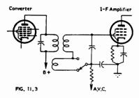
Fig. 11.3. Expanding selectivity with switched tertiary coil.
