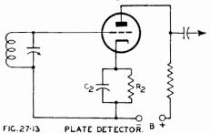
Screen grid and pentode valves with self-bias have been used as plate detectors very satisfactorily for a number of years, although the distortion with the usual arrangement is too high for them to be used in any but the cheapest radio receivers at the present time. Such a detector is, however, permissible for some types of short-wave reception and for amateur communication work where its high grid input impedance results in higher sensitivity and selectivity.
