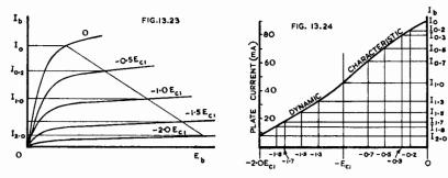
Fig. 13.23. Calculation of pentode power output and distortion using the five equal-voltage ordinate method.
