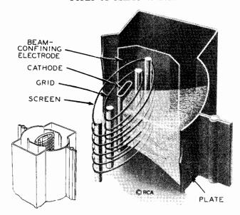
ELECTRON BEAM SHEETS FORMED BY GRID WIRES
