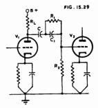
Fig. 15.29. Conventional treble boosting circuit.
