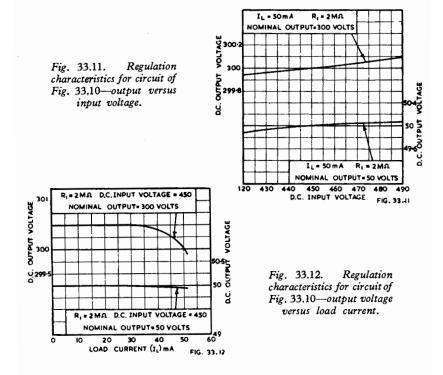
To draw a constant value of bleed current from the variable voltage supply, in order to prevent soaring of the output voltage on no load, some form of constant current device must be used. Refer to explanation of points 2 and 4 under Table 2. A suitable circuit is shown in Fig. 33.13 in which a 6V6-GT type valve is used as a constant current pentode; with plate voltages from 50 to 300 the plate current will only vary from 18.5 to 19.0 mA.
