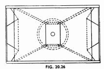
Fig. 20.26. Side and front views of the Klipsch bass reproducer Model K-3. (Ref. 48).
