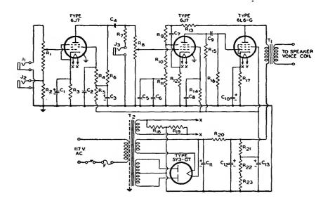
C<sub>1</sub>=16  $\mu$ f, electrolytic, 150 v. C<sub>2</sub> C<sub>8</sub>=0.1  $\mu$ f, paper, 400 v. C<sub>3</sub> C<sub>18</sub>=10  $\mu$ f, electrolytic, 450 v. C<sub>4</sub> C<sub>9</sub>=0.05  $\mu$ f, paper, 400 v. C<sub>8</sub>=0.1  $\mu$ f, paper, 200 v. C<sub>7</sub>=820  $\mu$ f, mica, 500 v. C<sub>19</sub>=20  $\mu$ f, electrolytic, 25 v. C<sub>10</sub> C<sub>12</sub>=25  $\mu$ f, electrolytic, 450 v. F=Fuse, 1 ampere J<sub>1</sub>=Jack for high-impedance crystal microphone input.
