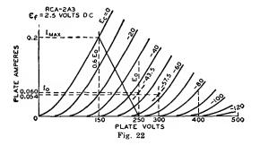
The method for calculating maximum power output for triodes in push-pull class A operation is as follows: Erect a vertical line at  $0.6E_o$  (see Fig. 22), intersecting the  $E_c=0$  curve at the point  $I_{max}$ . Then,  $I_{max}$  is determined from the curve for use in the formula
