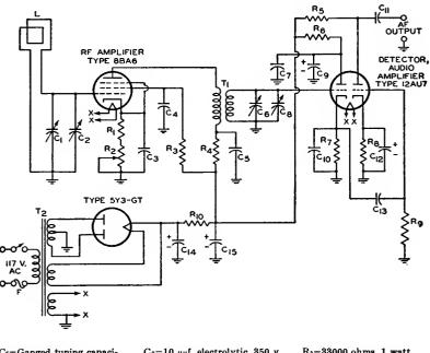
C<sub>1</sub> C<sub>6</sub>=Ganged tuning capacitors, 10-365 μμf
