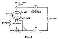
with a signal, the plate current varies with the signal. Because a small voltage applied to the grid can control a comparatively large amount of plate current, the signal is amplified by the tube. Typical three-electrode tube types are the 6C4, 6J5, and 2A3.
