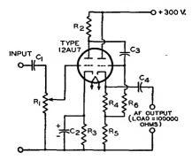
$\begin{array}{l} C_1 \ C_3 \!=\! 0.1 \ \mu f, \ paper, \ 400 \ v. \\ C_2 \!=\! 25 \ \mu f, \ electrolytic, \ 25 \ v. \\ C_4 \!=\! 5 \ \mu f, \ paper, \ 200 \ v. \end{array}$
