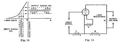
amplification, or gain, provided by the tube. The voltage amplification due to the tube is expressed by the following convenient formulas:
