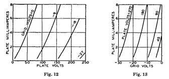
is obtained by varying plate voltage and measuring plate current for different grid bias voltages, while the transfer-characteristic curve is obtained by varying grid bias voltage and measuring plate current for different plate voltages. A platecharacteristic family of curves is illustrated by Fig. 12. Fig. 13 gives the transfercharacteristic family of curves for the same tube.
