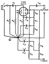
$\begin{array}{l} C_1 \ C_4 \ C_6 = 0.05 \ \mu\text{f}, \ paper, \ 600 \ v. \\ C_2 \ C_3 = 20 \ \mu\text{f}, \ electrolytic, \ 450 \ v. \\ C_5 = 0.01 \ \mu\text{f}, \ paper, \ 600 \ v. \\ J = Input \ connector, \ shielded \end{array}$
