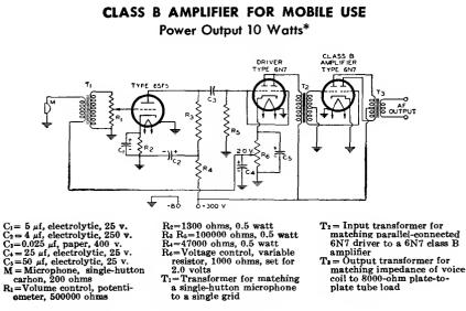
\* Peak signal-input voltage to 6SF5 grid required for full power output is 0.15 volt.
