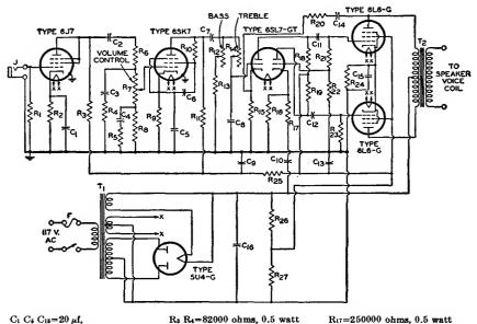
electrolytic, 25 v.  $C_2 C_4 C_7 = 0.01 \mu f$ , paper, 600 v.  $C_4 = 0.005 \mu f$ , paper, 100 v.  $C_4 = 0.000 \ \mu$ , paper, 100 v.  $C_5 = 0.5 \ \mu$ , paper, 600 v.  $C_8 = 330 \ \mu\mu$ , mica  $C_9 \ C_{12} = 30 \ \mu$ , electrolytic, 450 v.  $C_{10} \ C_{11} \ C_{12} \ C_{14} = 0.1 \ \mu$ , paper, 600 v.  $C_{16}=40 \ \mu f$ , electrolytic, 450 v. F=Fuse, 3 amperes J=Jack for high-impedance phono-pickup input R<sub>1</sub>=1 megohm, 0.5 watt R<sub>2</sub>=1800 ohms, 0.5 watt
