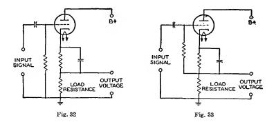
it presents negligible reactance at the lowest frequency to be handled. In both cases the B-supply should be increased to make up for the voltage taken for biasing. Example: Select a suitable tube and determine the operating conditions and circuit components for a cathode-follower circuit having an output impedance that will match a 500-ohm transmission line. Procedure: First, determine the approximate transconductance required.
