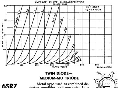
tector, amplifier, and avc tube. It is equivalent in performance to miniature type 6BF6. Outline 3, OUTLINES SECTION. Tube requires octal socket
