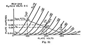
Line XY is known as the load resistance line. Its slope corresponds to the value of the load resistance. The load resistance in ohms is equal to  $(E_{max} - E_{min})$  divided by  $(I_{max} - I_{min})$ , where E is in volts and I is in amperes.
