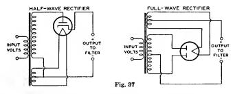
is approximately doubled. When mercury-vapor rectifier tubes are connected in parallel, a stabilizing resistor of 50 to 100 ohms should be connected in series with each plate lead in order that each tube will carry an equal share of the load. The value of the resistor to be used will depend on the amount of plate current that passes through the rectifier. Low plate current requires a high value; high plate current, a low value. When the plates of mercury-vapor rectifier tubes are connected
