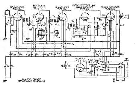
C<sub>1</sub> C<sub>4</sub> C<sub>8</sub> = Ganged tuning ca-pacitors, 20-450  $\mu\mu f$ C<sub>2</sub> C<sub>5</sub> C<sub>7</sub>=Trimmer capacitors,
