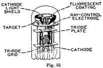
contain two main parts: (1) a triode which operates as a dc amplifier and (2) an electron-ray indicator which is located in the bulb as shown in Fig. 55. The target is operated at a positive voltage and, therefore, attracts electrons from the cathode. When the electrons strike the target they produce a glow on the fluorescent coating of the target. Under these conditions, the target appears as a ring of light.
