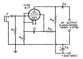
$C_1 = 0.25 \ \mu f$ , paper, oil-filled, C1=0.20 pm; 50 600 v. C2=0.5 µf, paper, oil-filled, 600 v.
