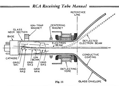
The electron gun includes a cathode for the production of free electrons, an electron "lens" system for accelerating the electrons and forming or focusing them into a very narrow beam, and, optionally, a device for "trapping" unwanted ions out of the electron beam.
