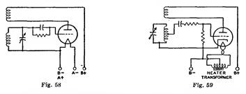
produced by electrostatic or electromagnetic coupling between the grid and plate circuits. When sufficient energy is fed back to more than compensate for the loss in the grid circuit, the tube will oscillate. The action consists of regular surges of power between the plate and the grid circuit at a frequency dependent on the circuit constants of inductance and capacitance. By proper choice of these values, the frequency may be adjusted over a very wide range.
