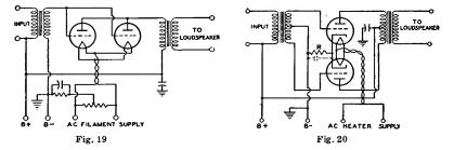
Operation of power tubes so that the grids run positive is inadvisable except under conditions such as those discussed in this section for class AB and class B amplifiers.
