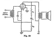
The application of the constantvoltage type of inverse feedback to a power output stage using a single beam power tube is illustrated by Fig. 28. In this circuit,  $R_1$ ,  $R_2$ , and C are connected across the output of the 6L6 as a voltage divider. The secondary of the grid-input transformer is returned to a point on this voltage divider. Capacitor C blocks the dc plate voltage from the grid. However, a portion of the tube's af output voltage, approximately equal
