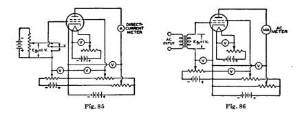
under conditions which approximate actual operating conditions. The alternating component of the plate current is read by means of an acammeter of the dynamometer type. The transconductance of the tube is equal to the ac plate current divided by the input-signal voltage. If a one-volt rms signal is applied to the grid, the plate-current-meter reading in milliamperes multiplied by one thousand is the value of transconductance in micromhos.
