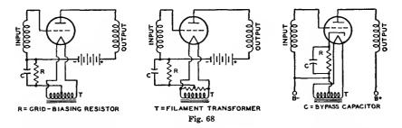
equal to the plate current in the case of a triode, or to the sum of the plate and grid-No.2 currents in the case of a tetrode, pentode, or beam power tube. Because the voltage drop along the resistance is increasingly negative with respect to the cathode, the required negative grid-bias voltage can be obtained by connecting the grid return to the negative end of the resistance.
