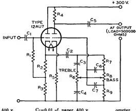
$\begin{array}{l} C_1{=}0.01 \ \mu f, \ paper, \ 400 \ v. \\ C_2{=}0.02 \ \mu f, \ paper, \ 200 \ v. \\ C_4{=}0.005 \ \mu f, \ mica, \ 200 \ v. \\ C_5{=}0.05 \ \mu f, \ paper, \ 400 \ v. \\ C_5{=}0.05 \ \mu f, \ paper, \ 400 \ v. \\ C_5{=}0.001 \ \mu f, \ paper, \ 200 \ v. \\ \end{array}$
