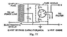
rms value. Transformers having electrostatic shielding between primary and secondary are not likely to transmit rf disturbances to the line. Often the interference may be eliminated simply by making the plate leads of the rectifier extremely short. In general, the particular method of interference elimination must be selected by experiment for each installation.
