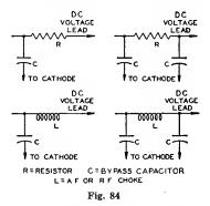
low-impedance path, while the choke or resistor assists in diverting the signal through the capacitor by offering a high impedance to the power-supply circuit.
