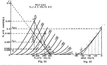
power in the grid circuit. The sum of this loss and the loss in the input transformer is the total driving power required by the grid circuit. The driver stage should be capable of a power output considerably larger than this required power in order that distortion introduced in the grid circuit be kept low. The input transformer used in a class  $AB_2$  amplifier usually has a stepdown turns ratio.
