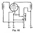
the high uniformity of the screen-grid current characteristic in pentodes and beam power tubes. Because the screengrid voltage rises with increase in bias and resulting decrease in screen-grid current, the cutoff characteristic of a pentode is extended by this method of supply.
