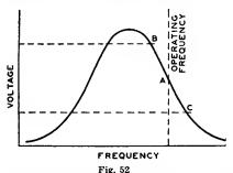
of Fig. 52. With modulation, the frequency swings between B and C, and
