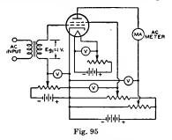
applied to the grid. Thus, the tube is tested under conditions which approximate actual operating conditions. The alternating component of the plate current is read by means of an ac ammeter of the dynamometer type. The transconductance of the tube is equal to the ac plate current divided by the inputsignal voltage. If a one-volt rms signal is applied to the grid, the plate-currentmeter reading in milliamperes multiplied by one thousand is the value of transconductance in micromhos.
