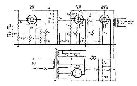
C<sub>1</sub>=16  $\mu$ f, electrolytic, 150 v. C<sub>2</sub> C<sub>8</sub>=0.1  $\mu$ f, paper, 400 v. C<sub>3</sub> C<sub>13</sub>=10 $\mu$ f, electrolytic, 450 v. C<sub>4</sub> C<sub>9</sub>=0.05  $\mu$ f, paper, 400 v. C<sub>8</sub>=0.25  $\mu$ f, paper, 200 v. C<sub>7</sub>=820  $\mu$ f, mica, 500 v. C<sub>10</sub>=20  $\mu$ f, electrolytic, 25 v. C<sub>11</sub>C<sub>12</sub>=25 $\mu$ f, electrolytic, 450 v.
