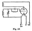
inductance and capacitance. By proper choice of these values, the frequency may be adjusted over a very wide range.
