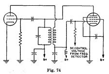
circuit. Because the plate current and plate voltage of the reactance tube are almost  $90^{\circ}$  out of phase, the control tube affects the tank circuit in the same manner as a reactance. The grid bias of the tube determines the magnitude of the effective reactance and, consequently, a control of this grid bias can be used to control the oscillator frequency.
