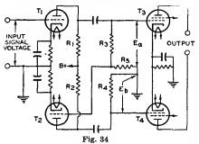
of triode  $T_3$ . A portion of the output voltage of  $T_1$  is also applied through the resistors  $R_3$  and  $R_5$  to the grid of  $T_2$ . The output voltage of  $T_2$  is applied to the grid of triode  $T_4$ .
