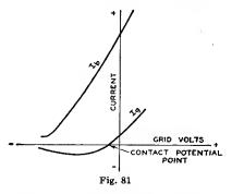
the initial velocity of emission of electrons from the cathode and an electrothermal effect due to the differences in temperature and in material composition of the grid and the cathode.
