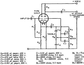
$R_6 R_8$ =Tone control, potenti-ometer, 1 megohm, audio taper (10 per cent of total re-sistance at 50 per cent rotation) R<sub>9</sub>=22000 ohms, 0.5 watt
