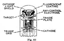
reach that portion of the target behind the electrode. Because the target does not glow where it is shielded from electrons, the control electrode casts a shadow on the glowing target. The extent of this shadow varies from approximately  $100^{\circ}$  of the target when the control electrode is much more negative than the target to  $0^{\circ}$  when the control electrode is at approximately the same potential as the target.
