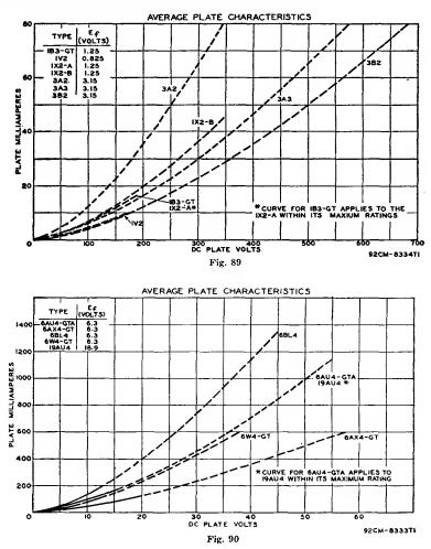
The value of peak plate current in a given rectifier circuit is largely determined by filter constants. If a large choke is used at the filter input, the peak plate current is not much greater than the load current; but if a large capacitor is used as the filter input, the peak current may be many times the load current. In order to determine accurately the peak plate current in any rectifier circuit, measure it with a peak-indicating meter or use an oscillograph.
