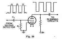
discriminates against the video information. Because the bias developed on the grid is proportional to the strength of the incoming signal, the circuit also has the advantage of being relatively independent of signal fluctuations.
