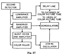
band from approximately 2.4 to 4.5 Mc is fed to a bandpass amplifier, as shown in the block diagram in Fig. 37. The color synchronizing signal, or "burst," con-
