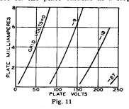
plate-voltage change—the latter equal to the product of the grid-voltage change and amplification factor. The  $\mu$  of a tube is often useful for calculating stage gain. This use is discussed in the ELECTRON TUBE APPLICATIONS SECTION.
