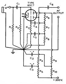
$\begin{array}{l} C_1 \ C_4 \ C_6 = 0.05 \ \mu f, \ paper, \ 600 \ v. \\ C_2 \ C_3 = 20 \ \mu f, \ electrolytic, \ 450 \ v. \\ C_6 = 0.01 \ \mu f, \ paper, \ 600 \ v. \\ J = Input \ connector, \ shielded \end{array}$
