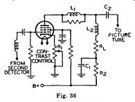
frequency. The inductance  $L_1$  isolates the output capacitance of the tube so that only stray capacitance is placed across the load. As a result, a highervalue load resistor is used to provide higher gain without affecting frequency response or phase relations. The decoupling circuit,  $C_1R_2$ , is used to improve the low-frequency response. Tubes used as video amplifiers include types 6CL6 and 12BY7, or the pentode sections of types 6AW8 and 6AN8.
