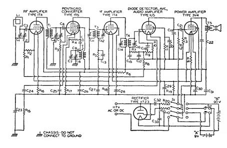
$C_1 C_4 C_8 = Ganged tuning ca$ pacitors, 20-450  $\mu\mu f$ C<sub>2</sub> C<sub>5</sub> C<sub>7</sub>=Trimmer capacitors.
