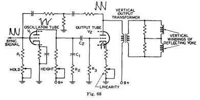
to illustrate the development of the desired current through the vertical output transformer and deflecting yoke.
