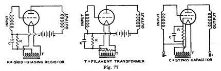
the resistor, or if the tube or tubes employ more than three electrodes, the total current determines the size of the resistor.
