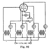
on the type of tube being tested. Any two shorted electrodes complete a circuit and light one or more lamps. Since two electrodes may be just touching to give a high-resistance short, it is desirable that the indicating lamps operate on very low current. It is also desirable to maintain the filament or heater of the tube at its operating temperature during the short-circuit test, because short-circuits in a tube may sometimes occur only when the electrodes are heated.
