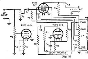
by changing the bias on grid No. 3. When the bias on grid No. 3 is made less negative, the gain of the 6L7 increases. The signal to be amplified is applied to grid No. 1 of the 6L7 and is amplified by the 6L7. The signal is also applied to the
