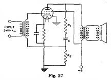
plate-current waveform, the af plate voltage has a waveform shown by  $e'_p$ . The plate-voltage waveform is inverted compared to the plate-current waveform because a plate-current increase produces an increase in the drop across the plate load. The voltage at the plate is the difference between the drop across the load and the supply voltage; thus, when plate current goes up, plate voltage goes down; when plate current goes down, plate voltage goes up.
