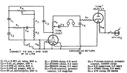
NOTES: (1) The point marked "GROUND AC RETURN" should he connected to a cold-water pipe or other conductor providing a direct, low-resistance return to ground. (2) High-impedance (2000 ohms or more) headphones are required.
