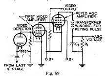
voltage developed across  $R_1$  is negative, it is suitable for application to the grids of the rf and if tubes as an agc voltage.
