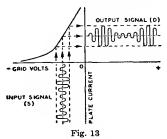
shows, by means of the grid-voltage vs. plate-current characteristics curve, the effect of an input signal (S) applied to the grid of a tube. The output signal (O) is the resulting amplified plate-current variation.
