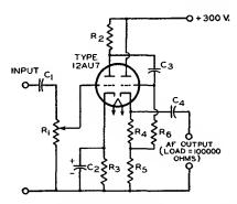
$\begin{array}{l} C_1 \ C_4 = 0.1 \ \mu f, \ paper, \ 400 \ v. \\ C_2 = 25 \ \mu f, \ electrolytic, \ 25 \ v. \\ C_4 = 5 \ \mu f, \ paper, \ 200 \ v. \end{array}$
