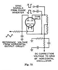
units and the grid of the horizontal-oscillator tube is essentially a low-pass filter which prevents the horizontal sync pulses from affecting the horizontal-oscillator performance.
