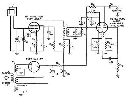
C1 C6=Ganged tuning capacitors, 10-365  $\mu\mu f$ C<sub>2</sub> C<sub>3</sub>=Trimmer capacitors,
