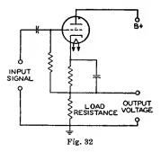
micromhos, the plate resistance is 62500 ohms, the amplification factor is 100, and the plate current is 0.0012 ampere. When these values are used in the expression for determining the cathode load resistance, we obtain
