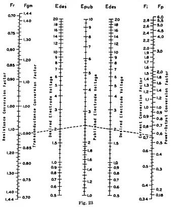
0.57,  $F_r$  is 1.12, and  $F_{gm}$  is approximately 0.892. These factors may be applied directly to operating values shown in the tube data, or to values calculated by the methods described previously.
