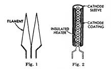
Directly heated filament-cathodes require comparatively little heating power. They are used in almost all of the tube types designed for battery operation because it is, of course, desirable to impose as small a drain as possible on the batteries. Examples of battery-operated filament types are the 1A7-GT, 1R5, 1U4, and 3V4. AC-operated types having directly heated filament-cathodes include the 2A3 and 5Y3-GT.
