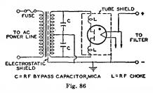
capacitors should have a voltage rating high enough to withstand the peak voltage of each half of the secondary, which is approximately 1.4 times the rms value.
