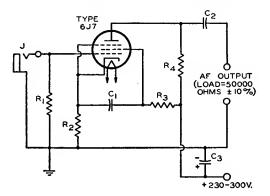
C<sub>1</sub>=0.25  $\mu$ f, paper, oil-filled, 600 v. C<sub>2</sub>=0.5  $\mu$ f, paper, oil-filled,
