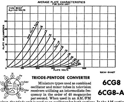
receiver, the triode unit is used as an oscillator for both sections. In the AM section, the pentode unit is used as a high-gain pentode mixer; in the FM section, the pentode unit is used either as a pentode mixer or as a triode-connected mixer depending on signal-to-noise considerations. Type 6CG8-A has a controlled heater
