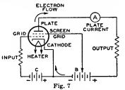
this shielding action is increased by a bypass capacitor connected between screen grid and cathode. By means of the screen grid and this bypass capacitor, the grid-plate capacitance of a tetrode is made very small. In practice, the gridplate capacitance is reduced from several micromicrofarads  $(\mu\mu f)$  for a triode to 0.01  $\mu\mu f$  or less for a screen-grid tube.
