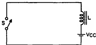
Fig. 85—Simplest form of deflection circuit.
