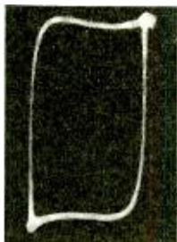
Fig. 18—Demonstration of time of transmission. Vertical deflection—input, wave shape as shown in Fig. 11. Horizontal deflection output.
