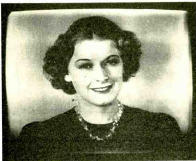
Fig. 8—Photograph of a 441-line television picture on the viewing screen of the Kinescope.
