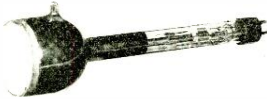
Fig. 6—Developmental model of a projection Kinescope. The face of the tube is carefully ground and polished.
