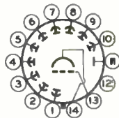
DIRECTION OF LIGHT: INTO END OF BULB
