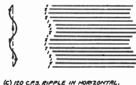
Fig. 6—Effect of ripple on thirty- to sixty-cycle interlaced pattern.
