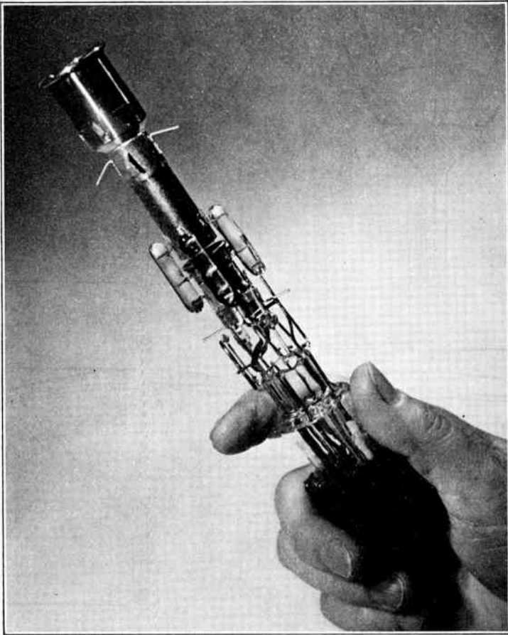
Fig. 11.8. Typical Kinescope Gun.
