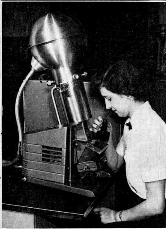
Fig. 4.4. RCA Electron Microscope, Type EMT.
