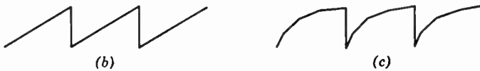
Fig. 19.10. Gamma Control Circuit for Flying-Spot Scanner. (a) Circuit. (b) Sawtooth wave. (c) Output of circuit for sawtooth input.
