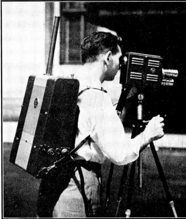
Fig. 21.6. Vidicon Camera with Backpack Transmitter. (Ohler, reference 5.)
