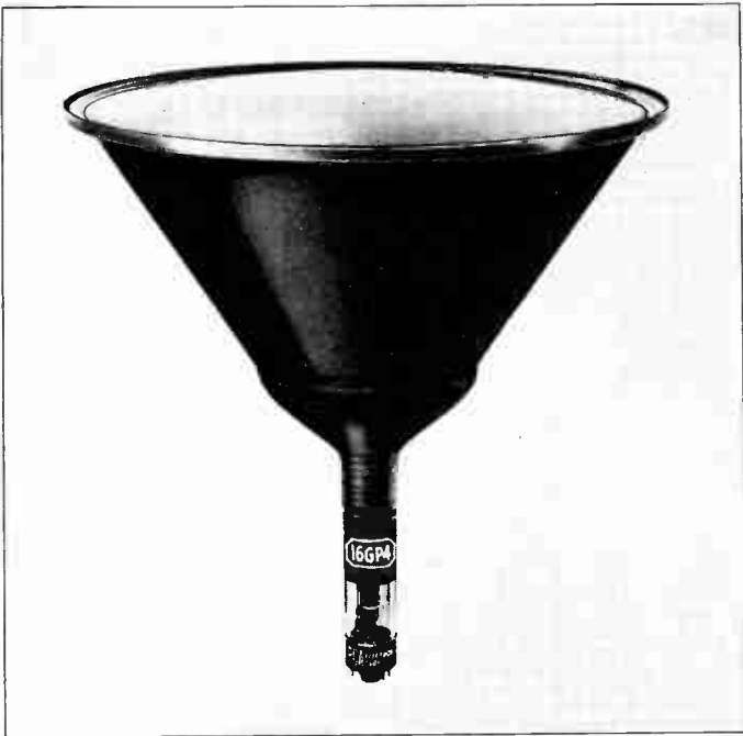
Fig. 11.31. The 16GP4, a Round Metal Kinescope.
