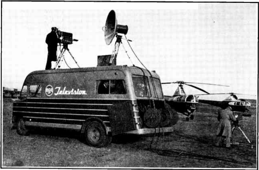
Fig. 21.23. A Mobile Unit for Remote Pickup.
