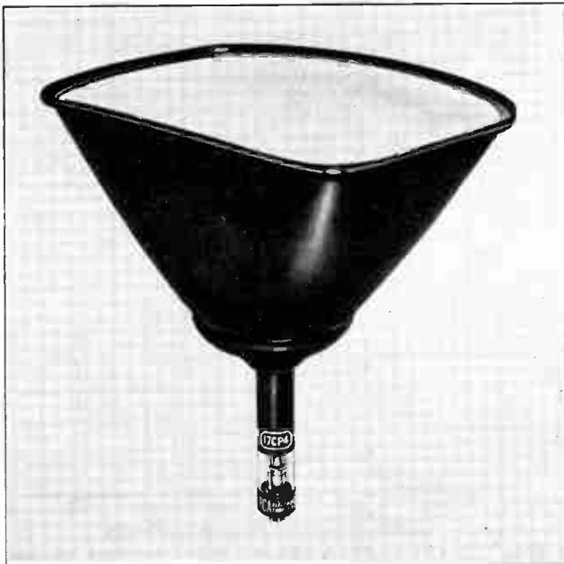
Fig. 11.32. The 17CP4, a Metal Kinescope with Rectangular Face Plate.
