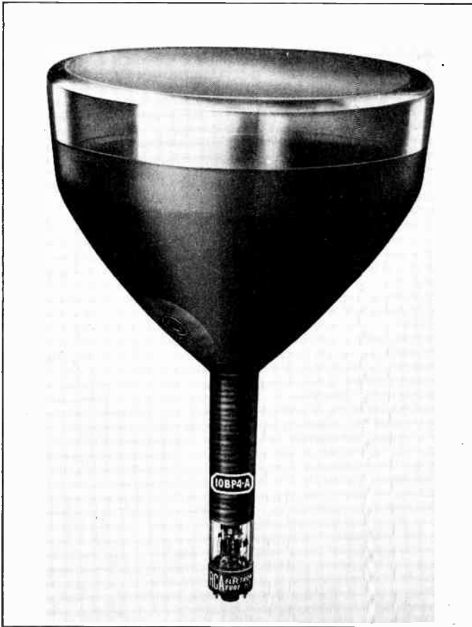
Fig. 11.28. The 10BP4-A Monitor Kinescope.
