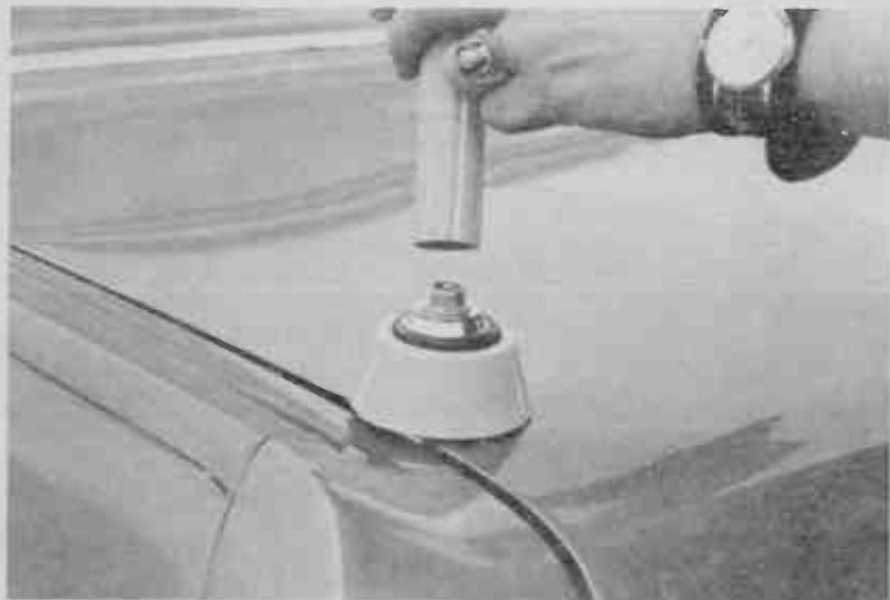
Position coil on base
