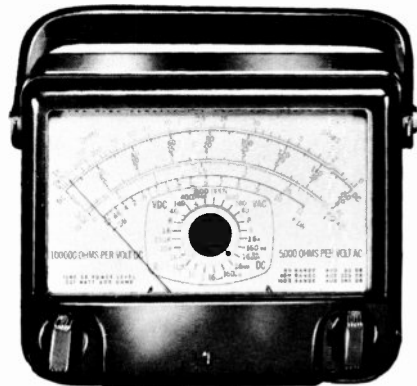
Fig. 1-7. High sensitivity VOM—measures 16 \mu a full scale.
