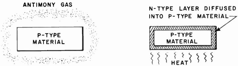
Fig. 3-3. When heat is applied to a piece of p-type germanium material in an atmosphere of antimony gas, a layer of n-type material is diffused into the outside like a crust.
