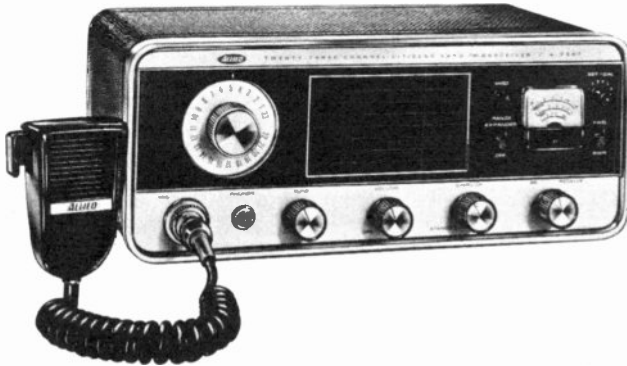
Fig. 3-7. The Allied Model A2567 transceiver has frequency synthesized circuit for 23-channel operation. It provides crystal-controlled transmit and receive functions on all Class-D band channels.
