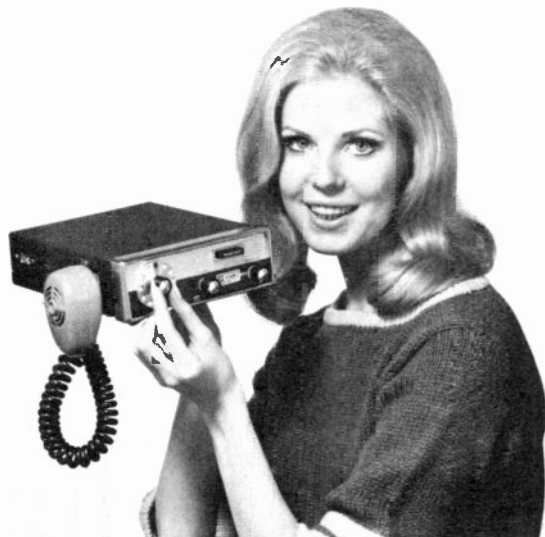
Fig. 1-4. A Knight-Kit® Citizens Band multichannel transceiver. A Class-D input with 5 watts input, it can be used as a mobile unit in a car, boat or truck, or with available accessories as a base station or portable unit.
