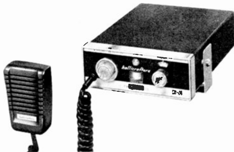
Fig. 3-3. The Hallicrafters Model CB-24 shown here is one example of a multichannel fixed-tuned CB transceiver.
