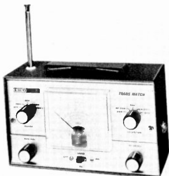
Fig. 8-8. The Eico Model 715 CB transmitter tester for checking modulation and RF power output of a transmitter.
