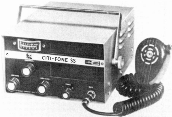
Fig. 3-5. Citi-Fone 23-channel transceiver for base or mobile use.
