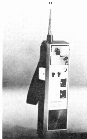
Fig. 3-16. This Lloyds Walkie Talkie includes a call signal capability as an integral part of its circuitry.
