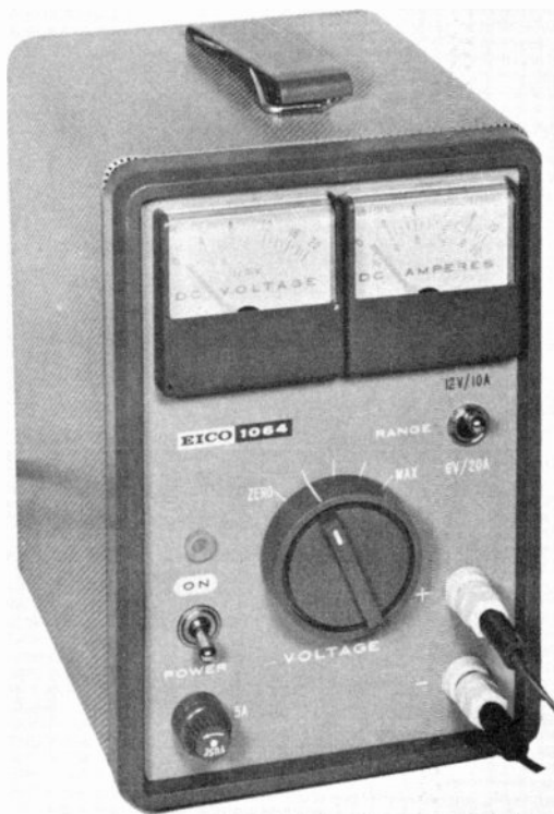
Fig. 8-1. A typical 6/12-volt filtered DC power supply.
