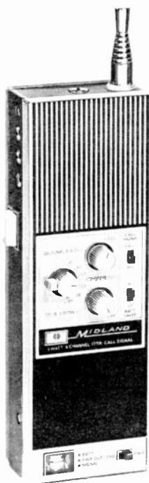
Fig. 3-13. Midland 5-watt 6-channel walkie-talkie is available with rechargeable batteries.
