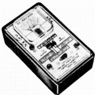
Fig. 8-7. The Seco Model 500 test set can be used for checking crystals; it also provides an RF test signal for other types of troubleshooting.
