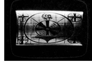
Low emission in the low-voltage rectifier tube, or faulty semiconductor rectifiers, are to blame here.
