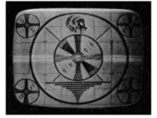
Fig. 15. Effect of heater-tocathode leakage in local oscillator.
