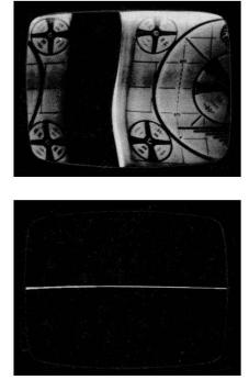
Fig. 22. Horizontal-sync pulse absent but oscillator on frequency.
