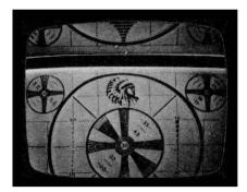
Fig. 21. Vertical-sync pulse absent but oscillator on frequency.
